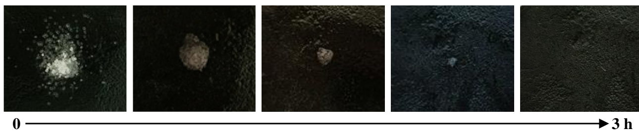
Figure S17. Self-cleaning test of composite hydrogel.
