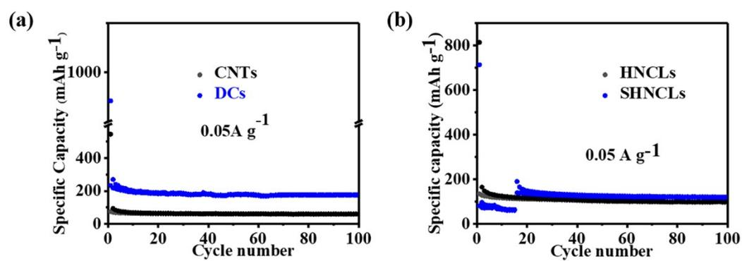
Fig. S10 The cycling performances of DCs, CNTs, HNCLs and SHNCLs at 0.05 A g<sup>-1</sup> for 100 cycles.
