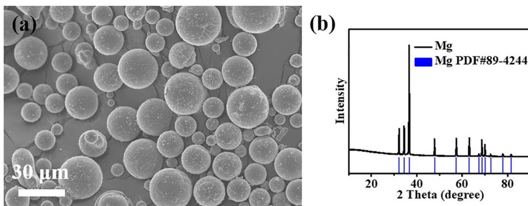
**Fig. S1** (a) The SEM image of Mg spheres. (b) The XRD pattern of Mg spheres.
