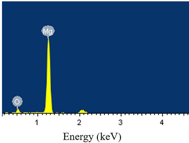
**Fig. S5** The EDX image of Mg sphere.
