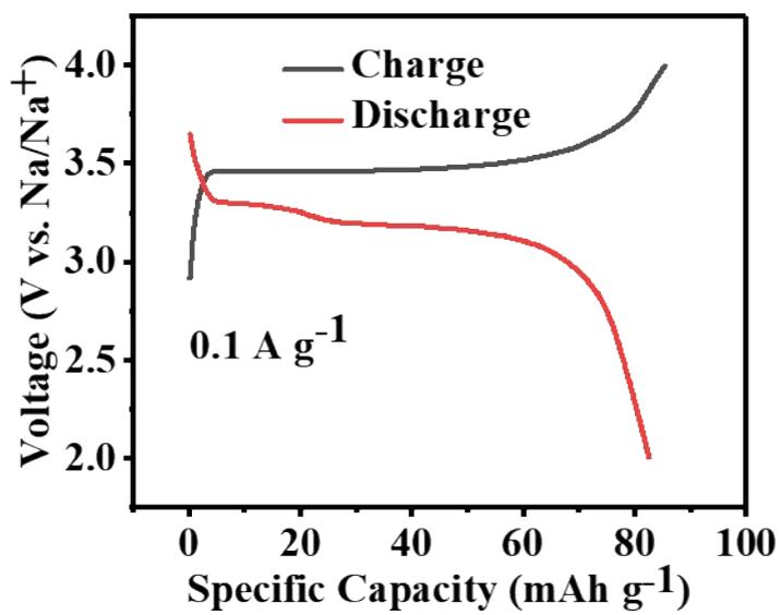
Fig. S12 The charge/discharge curve of  $\text{Na}_3\text{V}_2(\text{PO}_4)_3$  electrode at half cell.
