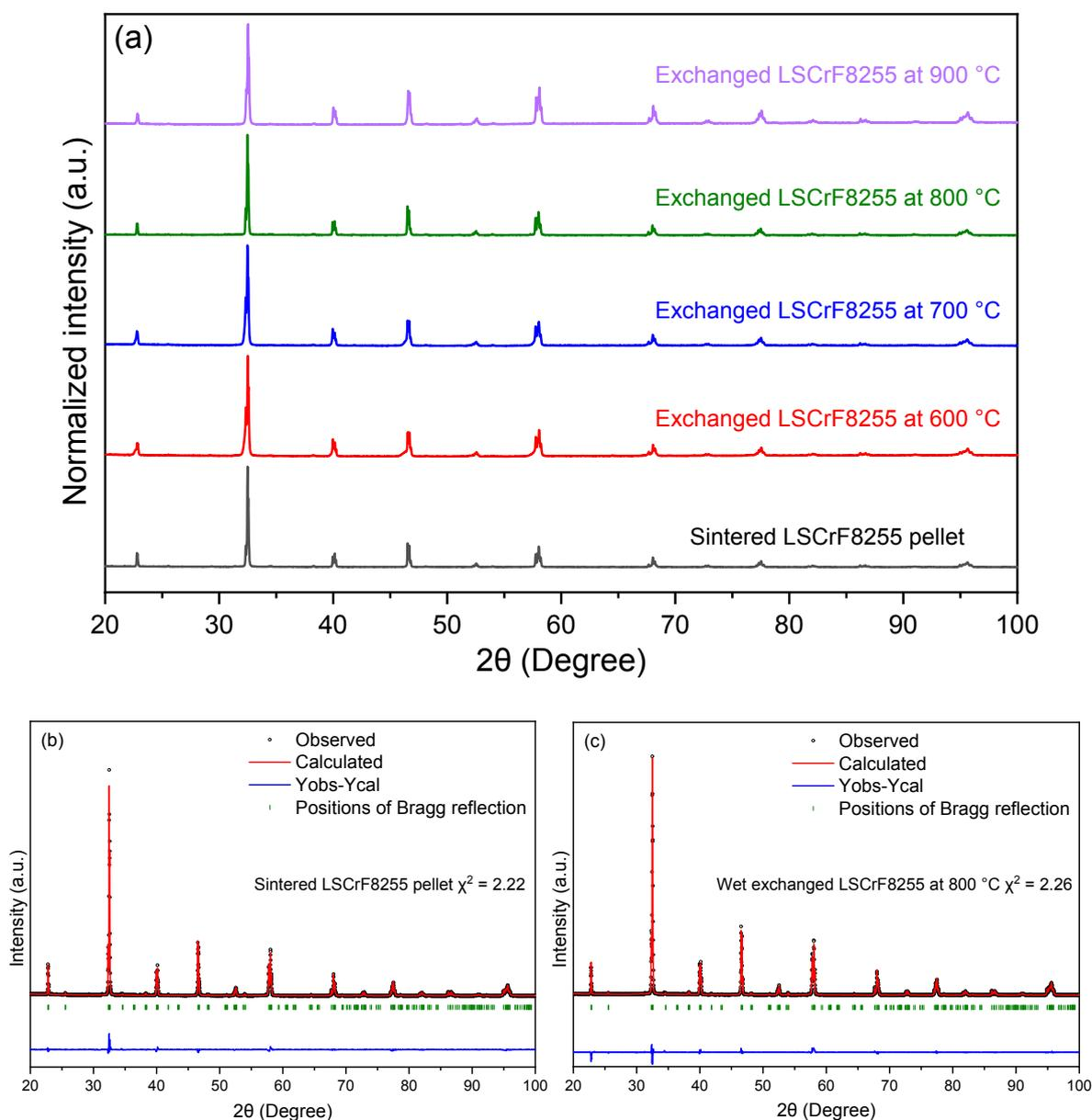
Figure S2. (a) XRD patterns of the sintered and wet exchanged LSCrF8255 pellets. (b and c) Rietveld refinement results of the sintered LSCrF8255 pellet and the wet exchanged LSCrF8255 at 800 °C where the black circles are the observed experimental data; the red solid line represents the calculated intensities; the blue solid line is the difference in intensity between the observed and calculated data (space group: *Pnma*); and the green vertical bars are the Bragg reflection positions.
