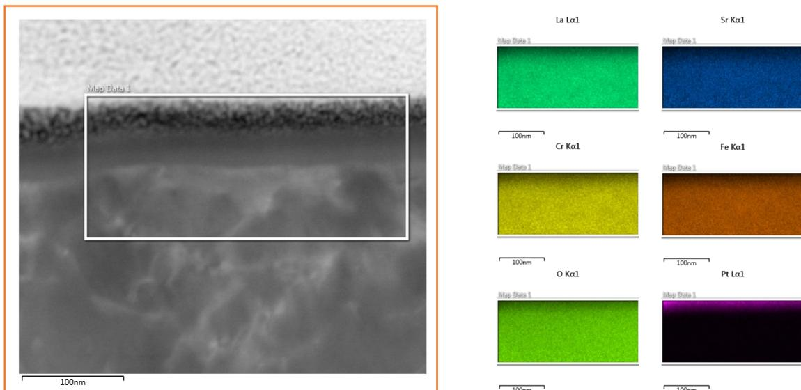
Figure S4. Representative STEM-EDX map showing an unsegregated grain. The sample surface was coated with Pt during TEM foil preparation.
