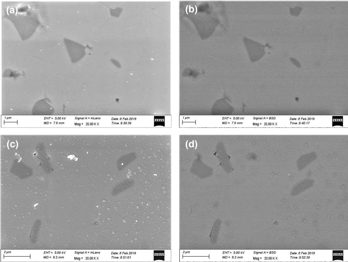
Figure S3. (a and b) SEM secondary electron (SE) and backscattered-electron (BSE) images of the LSCrF8255 sample wet exchanged at 600 °C; (c and d) SE and BSE images of the LSCrF8255 sample wet exchanged at 700 °C.
