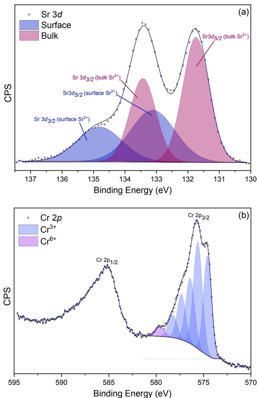
Figure S1. Fitted XPS spectra from the sintered pre-exchanged LSCrF8255 sample showing a) Sr 3d and b) Cr 2p
