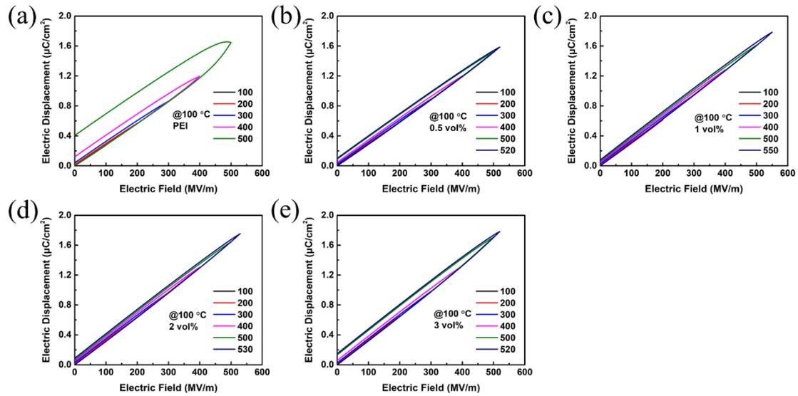
**Fig. S8.** Electric displacement-electric field (D-E) loops of nanocomposites with varied filler content measured at 100 °C, (a) PEI, (b) 0.5vol%, (c) 1vol%, (d) 2 vol%, and (e) 3 vol%.
