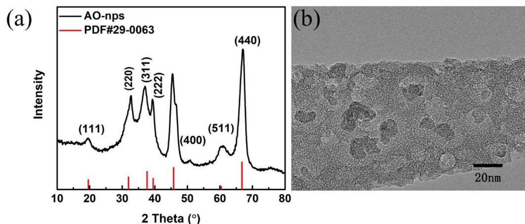
**Fig. S1.** (a) X-ray diffraction (XRD) patterns of the nanostructured Al<sub>2</sub>O<sub>3</sub> fillers. (b) TEM image of Al<sub>2</sub>O<sub>3</sub> particles.
