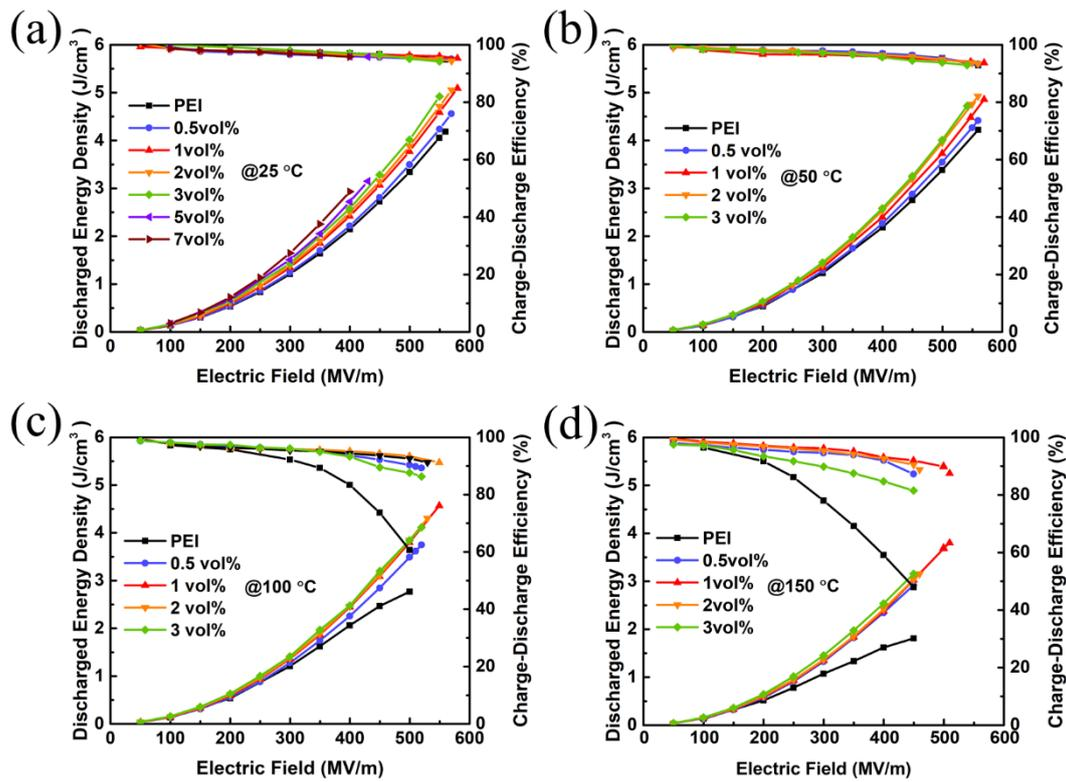
**Fig. S12.** Discharged energy density and charge-discharge efficiency of PEI/AO-nps nanocomposite films with varied filler contents measured at (a) 25 °C, (b) 50 °C, (c) 100 °C, and (d) 150 °C.
