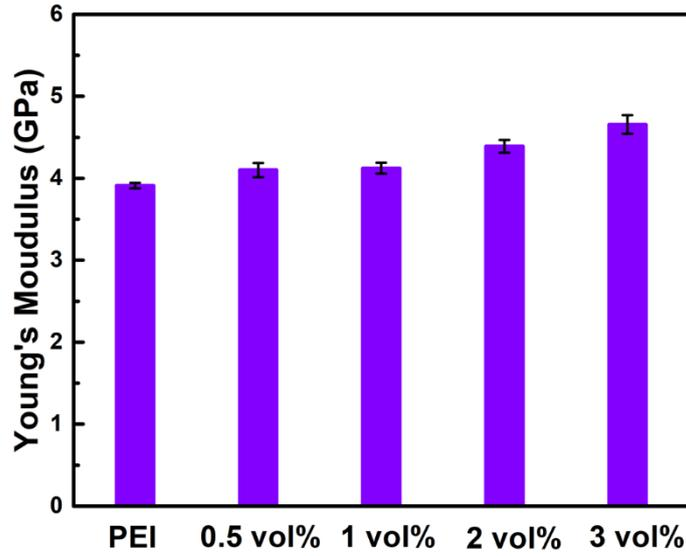
**Fig. S5.** Young's modulus of the nanocomposites with varied filler content measured at room temperature.
