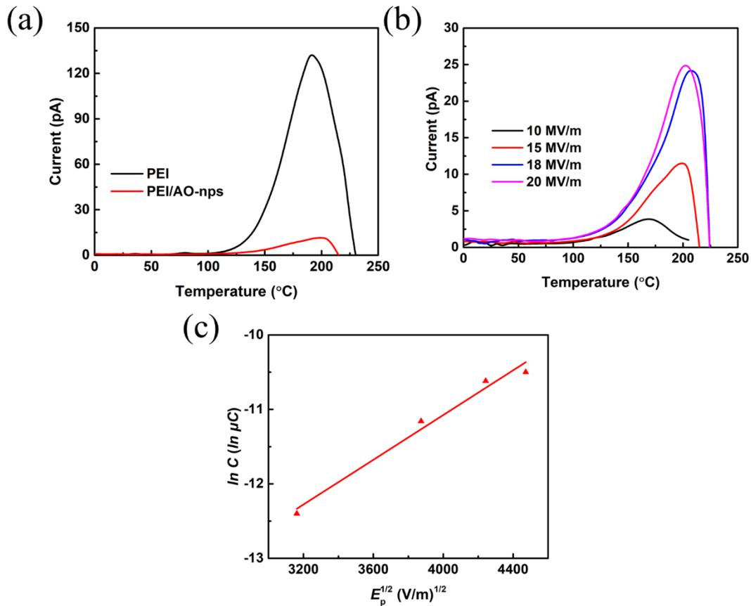
**Fig. S11.** (a) TSDC curves of PEI and PEI/AO-nps under poling electric field of 15 MV/m at 150 °C for 30 min. (b) TSDC spectra for PEI/AO-nps film under different poling electric field at 150 °C for 30 min. (c) The relationship between  $\ln C$  and  $E_p^{1/2}$ .
