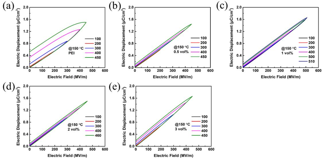
**Fig. S9.** Electric displacement-electric field (D-E) loops of nanocomposites with varied filler content measured at 150 °C, (a) PEI, (b) 0.5vol%, (c) 1vol%, (d) 2 vol%, and (e) 3 vol%.
