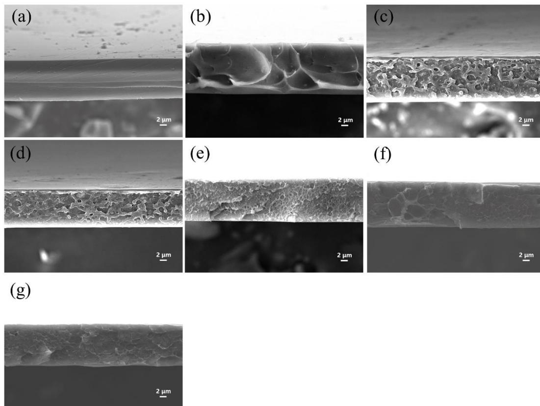
**Fig. S2.** Cross-sectional SEM images of (a) pure PEI film, (b) PEI nanocomposites with 0.5 vol% AO-nps, (c) PEI nanocomposites with 1 vol% AO-nps, (d) PEI nanocomposites with 2 vol% AO-nps, (e) PEI nanocomposites with 3 vol% AO-nps, (f) PEI nanocomposites with 5 vol% AO-nps, and (g) PEI nanocomposites with 7 vol% AO-nps.
