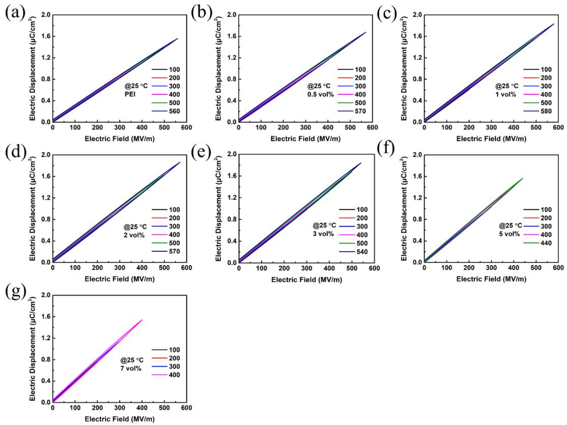
**Fig. S6.** Electric displacement-electric field (D-E) loops of nanocomposites with varied filler content measured at 25 °C, (a) PEI, (b) 0.5 vol%, (c) 1 vol%, (d) 2 vol%, (e) 3 vol%, (f) 5 vol%, and (g) 7 vol%.
