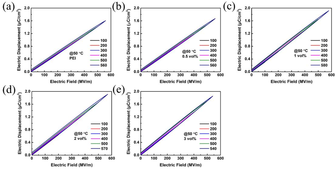
**Fig. S7.** Electric displacement-electric field (D-E) loops of nanocomposites with varied filler content measured at 50 °C, (a) PEI, (b) 0.5vol%, (c) 1vol%, (d) 2 vol%, and (e) 3 vol%.
