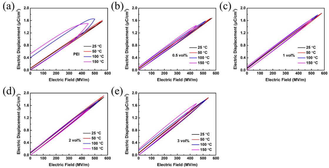
**Fig. S10.** Maximum electric displacement-electric field (D-E) loops of nanocomposites measured at different temperature, (a) PEI, (b) 0.5vol%, (c) 1vol%, (d) 2 vol%, and (e) 3 vol%.
