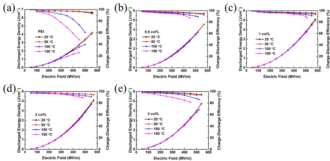
**Fig. S13.** Discharged energy density and charge-discharge efficiency of PEI/AO-nps nanocomposite films measured at different temperature, (a) PEI, (b) 0.5 vol%, (c) 1 vol%, (d) 2 vol%, and (e) 3 vol%.
