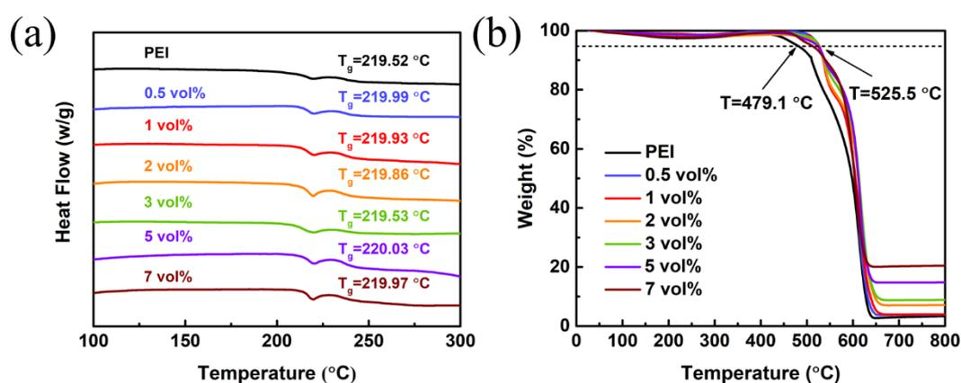
**Fig. S3.** (a) DSC and (b) TGA curves of pristine PEI and the PEI/AO-nps nanocomposite films.
