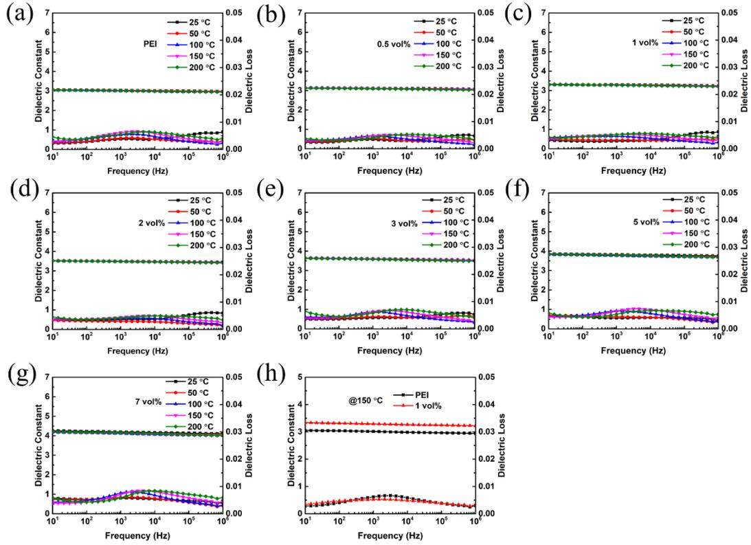
**Fig. S4.** Dielectric spectra of nanocomposites with varied frequency and temperature, (a) PEI, (b) 0.5vol%, (c) 1vol%, (d) 2 vol%, (e) 3 vol%, (f) 5 vol%, and (g) 7vol%. (h) Frequency-dependent dielectric properties of the PEI and PEI composite with 1vol% AO-nps at 150 °C.
