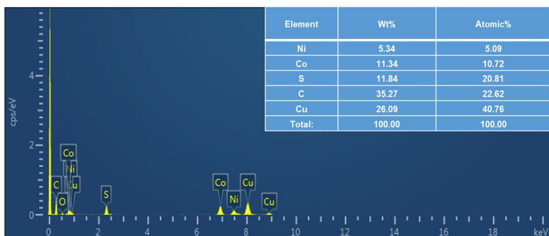
Fig. S5. EDS spectrum of \text{NiCo}_2\text{S}_4 nanotube (the inset table shows the corresponding atomic contents).
