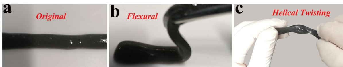
Figure S5. Excellent mechanical properties of the PBPM-2 hydrogel: (a) original state of the PBPM-2 hydrogel; (b) flexural and (c) helical twisting state of the PBPM-2 hydrogel.
