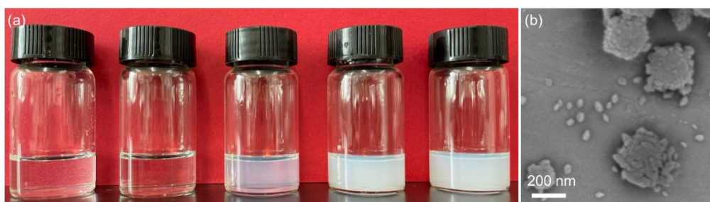
Figure 4. (a) The time-dependent growth picture of Ga-MOFs from left to right at 15, 20, 25, 30 and 35 min; (b) the FE-SEM image of the Ga-MOF at 25 min.
