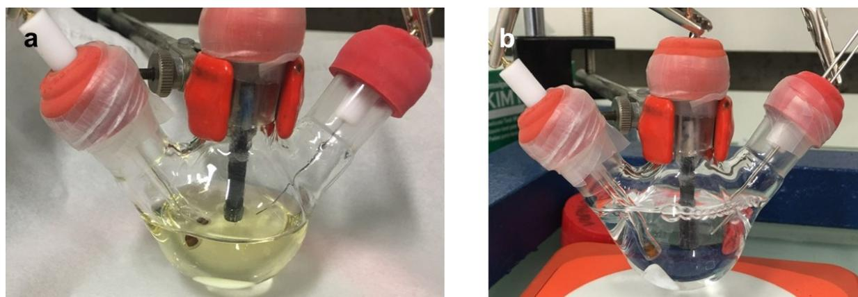
**Figure S17.** Photographic pictures of the electrochemical cells taken during the DMS oxidation performed under argon (a) and O<sub>2</sub> (b). No coloration of the solution is observed under oxygen due to the fast reaction between sulfur radicals and the oxygen molecules.
