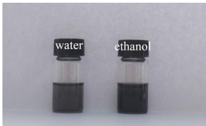
Fig. S1. Digital photo of the distribution of \text{Ti}_3\text{C}_2\text{T}_x nanosheets ( 1.0 \text{ mg mL}^{-1} ) in water and ethanol solution.
