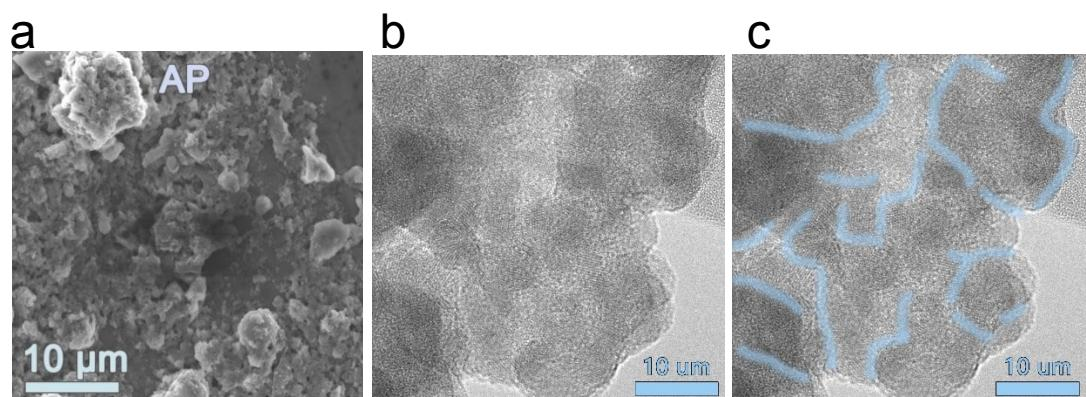
**Figure S1.** (a) SEM image of amorphous phosphorus; (b) original TEM image of amorphous phosphorus; (c) TEM image highlighting (light blue) the grain interface in amorphous phosphorus
