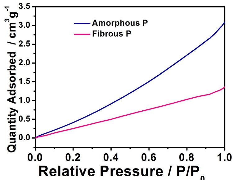
**Figure S10.** CO<sub>2</sub> adsorption curve of amorphous P and fibrous P
