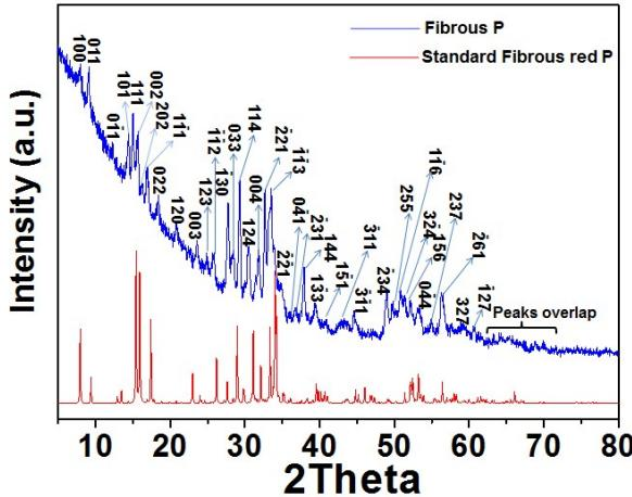
**Figure S2.** XRD pattern of fibrous red P in detail.
