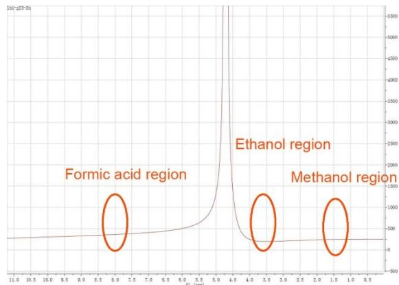
**Figure S8.** Hydrogen nuclear magnetic resonance spectrum of solution after CO<sub>2</sub> reduction on fibrous P. No peak related to formic acid, methanol or ethanol can be found.
