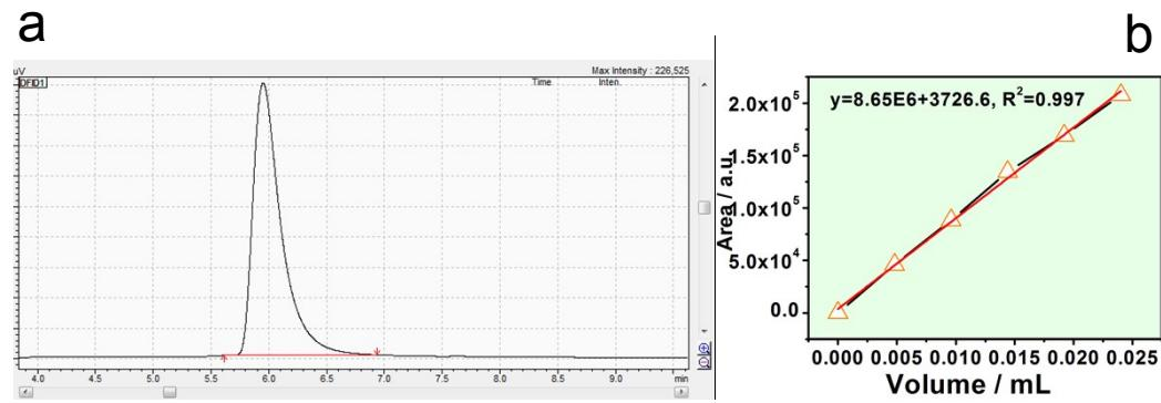
**Figure S7.** GC curve showing the formation of CO and (b) standard curve showing the peak area as a function of CO volume.
