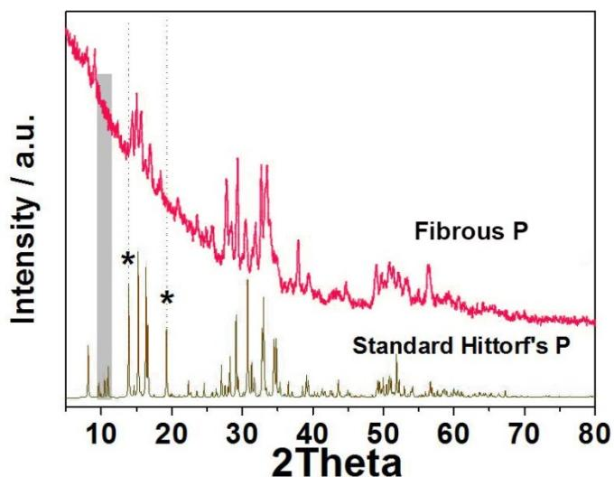
**Figure S3.** Comparison of the XRD pattern for experimental-synthesized fibrous P and standard hittorf's P
