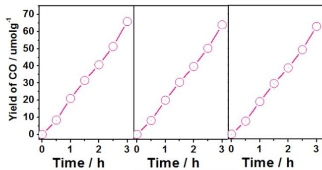
**Figure S9.** Cycling test of CO<sub>2</sub> reduction into CO on Fibrous P.
