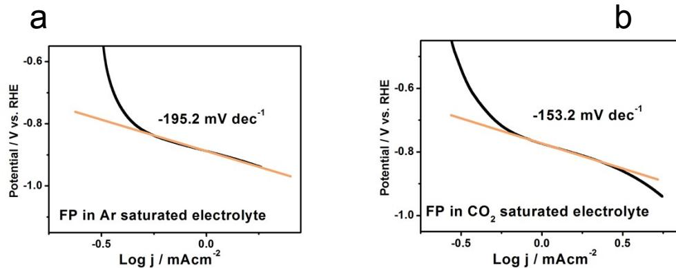
**Figure S13.** Tafel plot of fibrous P in (a) Ar, and (b)  $\text{CO}_2$  saturated 1M  $\text{KHCO}_3$  electrolyte
