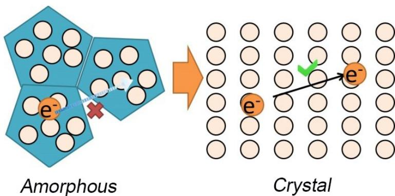
**Scheme S1.** Diagram comparing the charge transfer in amorphous and crystal structure.
