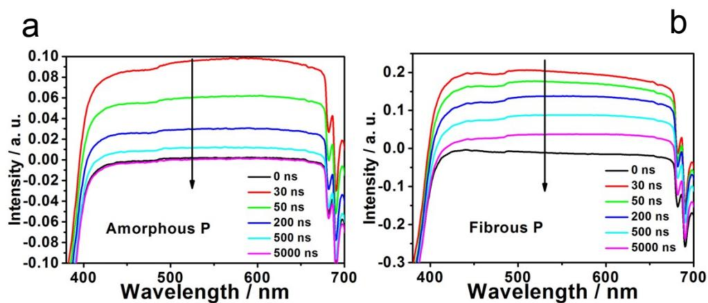
**Figure S11.** Nanosecond transient absorption spectra of (a) amorphous and (b) crystalline red phosphorus.
