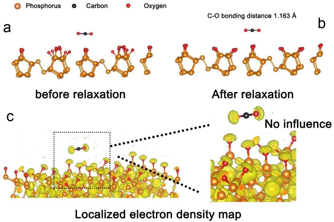
**Figure S16.** Structure of fibrous P with an oxygen layer (a) before, and (b) after structure relaxation. (c) Localized electron density map.
