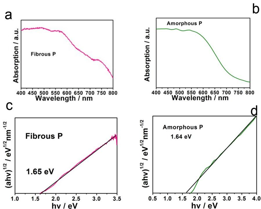
**Figure S5.** Absorption spectra of (a) fibrous P and (b) amorphous P. Kubelka–Munk plots converted from the absorption spectra of (a) fibrous P and (b) amorphous P.
