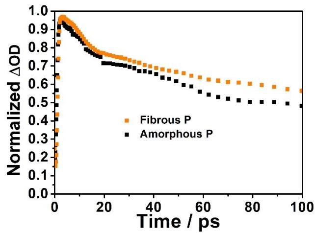
**Figure S12.** Magnified femtosecond absorption transient spectrum of amorphous P and fibrous P in the beginning 100 ps.
