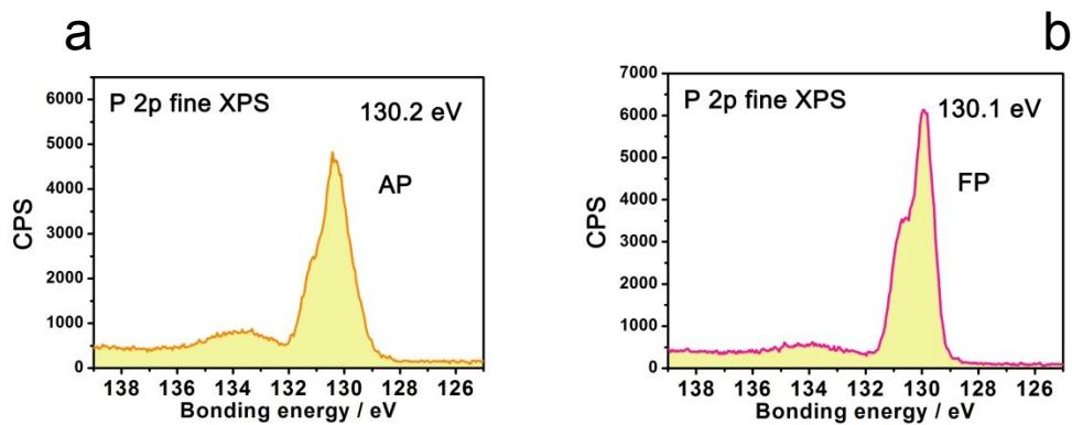
**Figure S4.** The P 2p fine XPS spectra of (a) amorphous P and (b) fibrous P
