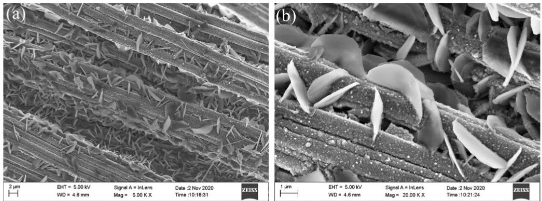
Fig. S7 FE-SEM images for NiO/CC electrode after the 1<sup>st</sup> cycle discharge. (Under a limited capacity of 2000 mA h g<sup>-1</sup> at 0.2 mA cm<sup>-2</sup>)
