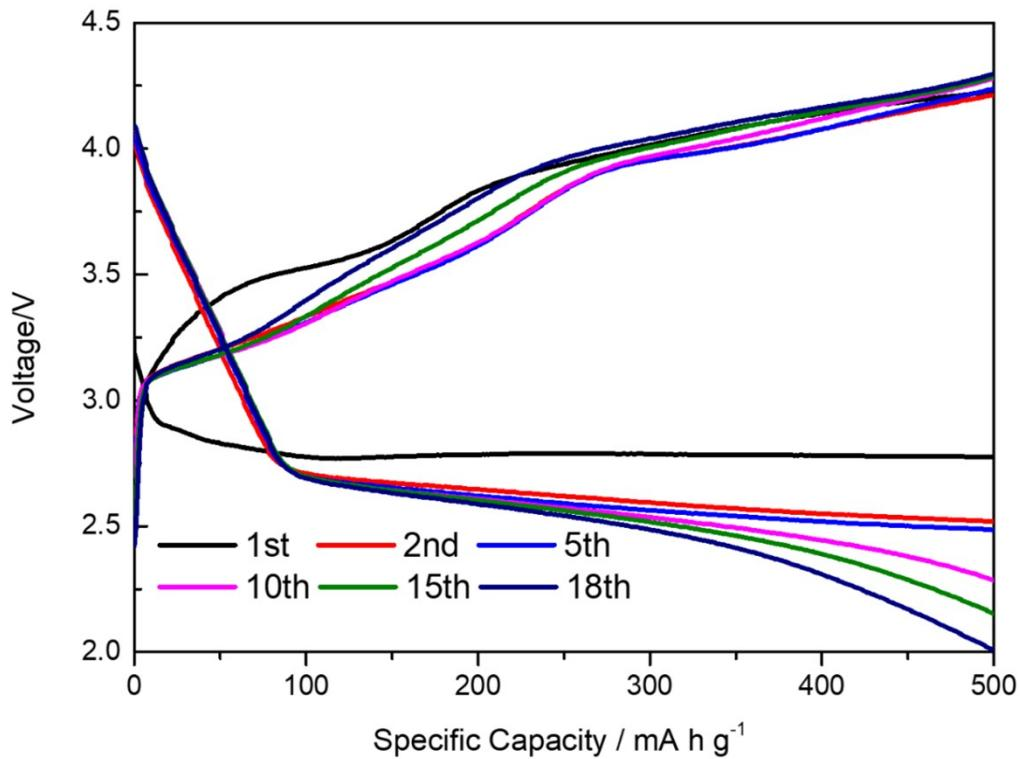
Fig. S5 The discharge and charge curves of LOBs with the NiO/CC under a limited capacity of  $500 \text{ mA h g}^{-1}$  at  $0.2 \text{ mA cm}^{-2}$ .
