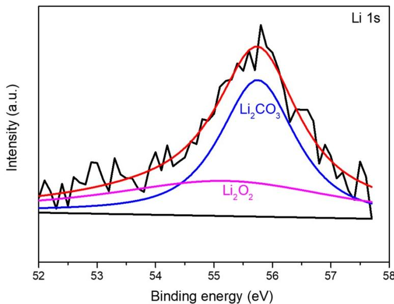
Fig. S6 The ex-situ XPS spectra of  $\text{CuCo}_2\text{O}_4@\text{NiO/CC}$  cathode after first overcharge (The charge specific capacity of  $11721 \text{ mA h g}^{-1}$  exceeds the corresponding discharge specific capacity of  $9335 \text{ mA h g}^{-1}$ ) in Li 1s regions at  $0.2 \text{ mA cm}^{-2}$ .
