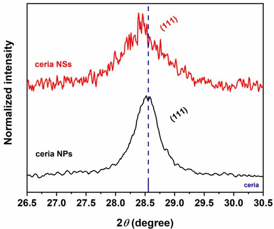
**Fig. S3** XRD patterns of ceria NSs and NPs in the (111) diffraction region. The (111) peak positions of ceria NSs and NPs are  $28.45^\circ$  and  $28.55^\circ$ , respectively.
