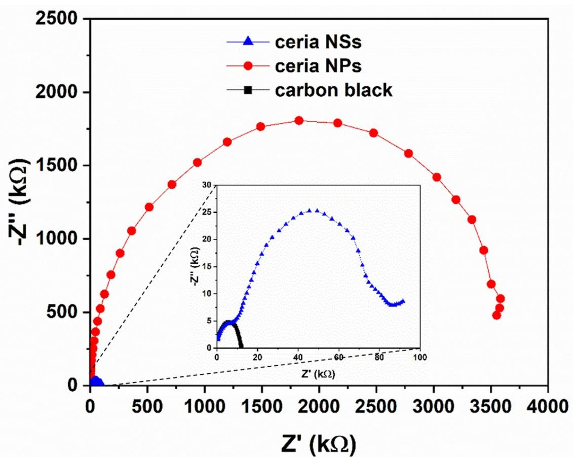
**Fig. S2** Nyquist plots of ceria NSs and NPs. For comparison, the Nyquist plot of carbon black is also included.
