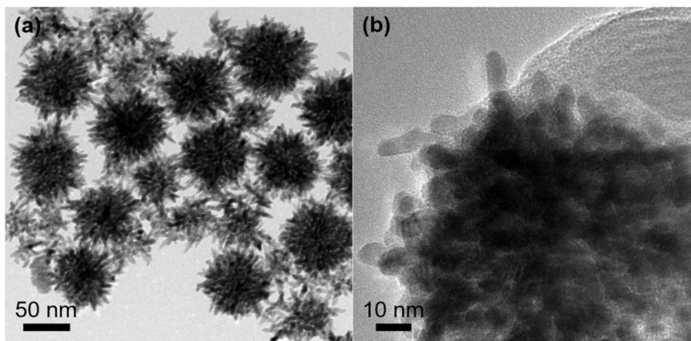
**Fig. S9** TEM images of (a) PtNi NDs and (b) PtNi/ceria\* prepared by depositing the PtNi NDs on pre-synthesized ceria NSs.
