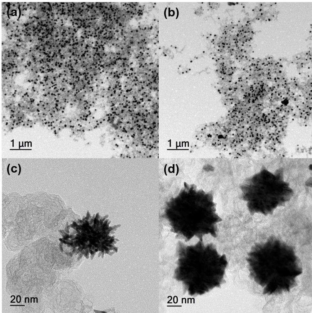
**Fig. S7** TEM images of (a,c) Pt<sub>3</sub>Ni/C and (b,d) PtNi/C. The average sizes of the Pt<sub>3</sub>Ni and PtNi NDs were  $57.1 \pm 6.3$  and  $62.9 \pm 6.1$  nm, respectively.
