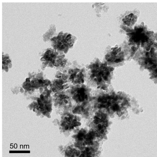
**Fig. S6** TEM image of PtNi/ceria after the ADT, demonstrating that the dendrite structure of PtNi/ceria was preserved after the ADT.
