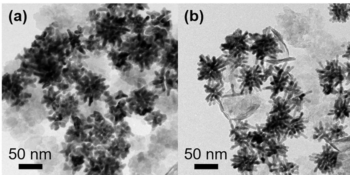
**Fig. S1** TEM images of (a) Pt<sub>3</sub>Ni/ceria and (b) Pt/ceria. The average sizes of the Pt<sub>3</sub>Ni and Pt NDs were  $56.5 \pm 8.7$  and  $58.2 \pm 6.3$  nm, respectively.
