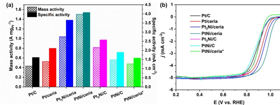
**Fig. S8** (a) Mass and specific activities of various catalysts towards MOR. (b) ORR polarization curves of various catalysts.  $E_{1/2}$  values of Pt/C, Pt/ceria, Pt<sub>3</sub>Ni/ceria, PtNi/ceria, Pt<sub>3</sub>Ni/C, PtNi/C, and PtNi/ceria\* were 0.889, 0.925, 0.944, 0.978, 0.900, 0.876, and 0.898 V vs. RHE, respectively.
