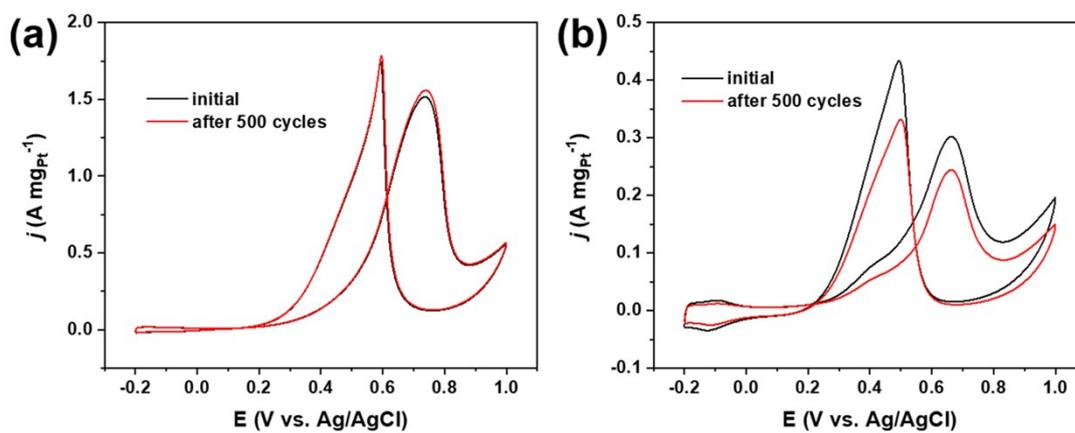
**Fig. S5** CVs of (a) PtNi/ceria and (b) Pt/C in 0.1 M  $\text{HClO}_4$  + 0.5 M methanol at a scan rate  $50 \text{ mV s}^{-1}$  before and after 500 potential cycles between -0.2 and 1.0 V vs. Ag/AgCl.
