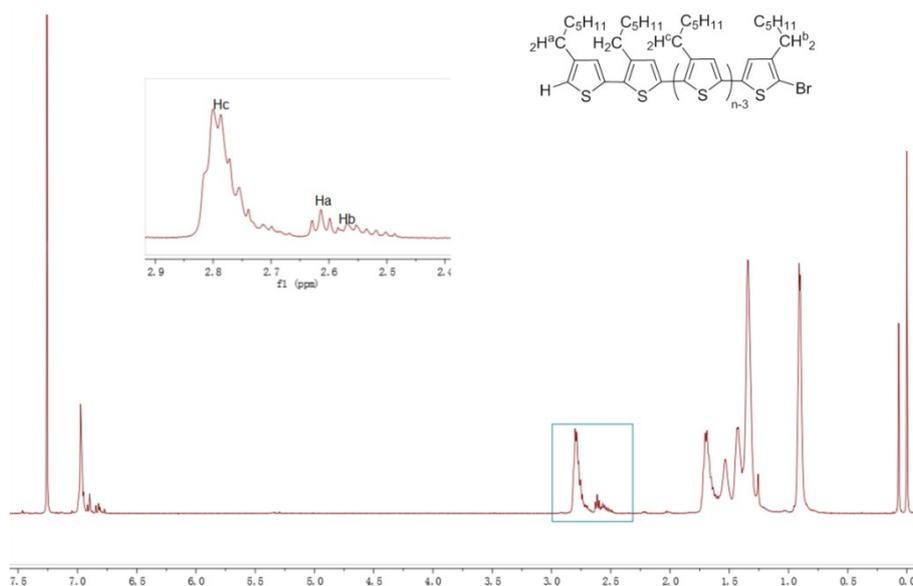
**Figure S1.**  $^1\text{H NMR}$  spectrum (400 MHz,  $\text{CDCl}_3$ , 298K) of pre-polymer P3HT.
