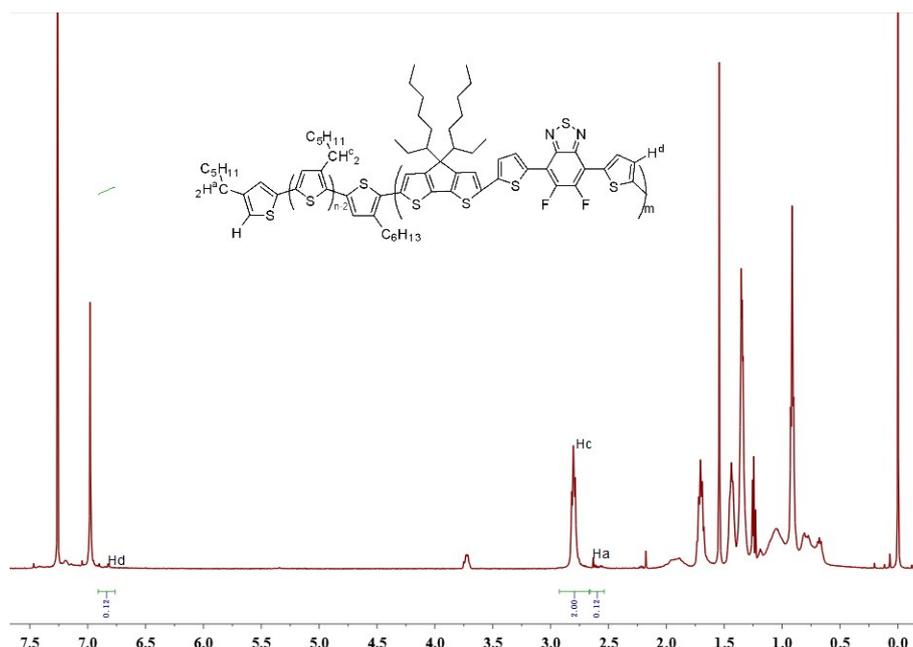
**Figure S3.**  $^1\text{H}$  NMR spectrum (400 MHz,  $\text{CDCl}_3$ , 298K) of polymer CDT.
