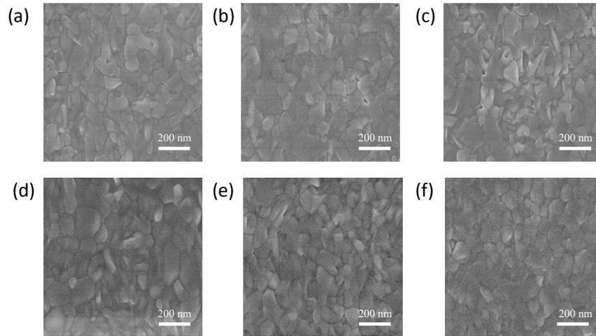
**Figure S9.** Top-view SEM images of perovskite films on DTS (a), CDT (b) and DTP (c) films. And SEM images of perovskite films on DTS/PSBMA (a), CDT/PSBMA (b) and DTP/PSBMA (c) films.
