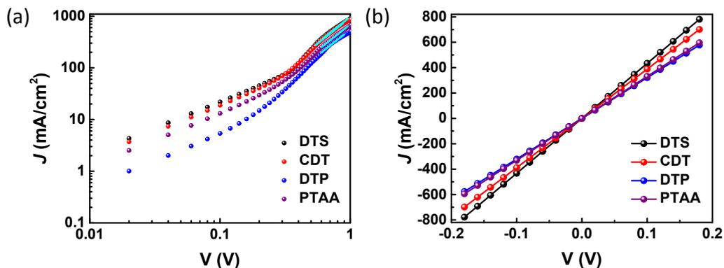
**Figure S11.** (a) Measured  $J$ - $V$  curves for ITO/PEDOT: PSS/HTL/Ag devices with different HTLs. (b) The  $J$ - $V$  diagrams of conductivity of different HTL films. The device structure is ITO/HTL/Ag.
