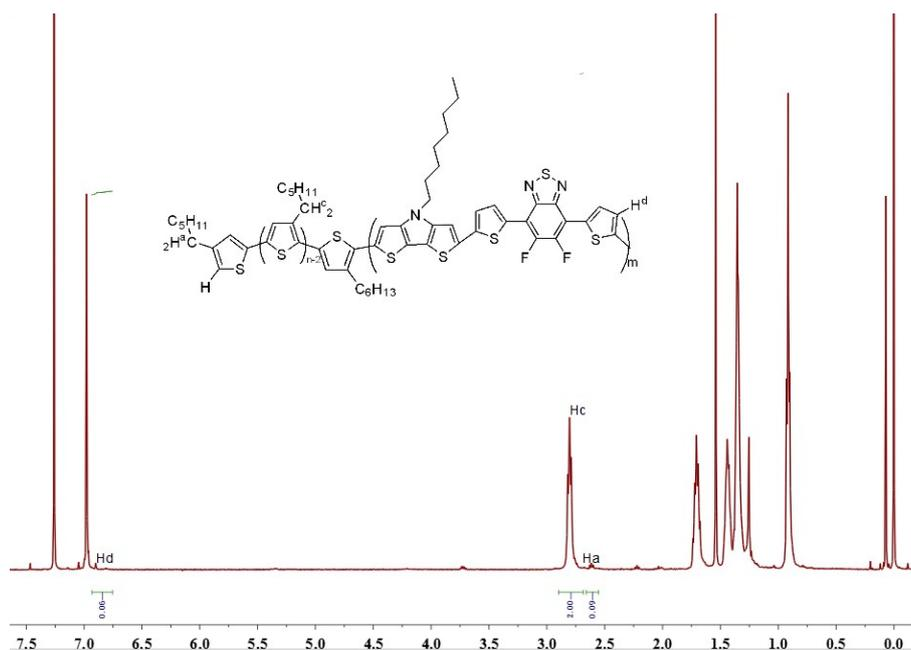
**Figure S4.**  $^1\text{H}$  NMR spectrum (400 MHz,  $\text{CDCl}_3$ , 298K) of polymer DTP.
