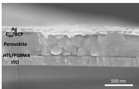
**Figure S6.** The cross-section scanning electron microscopy (SEM) image of ITO/HTL/PSBMA/perovskite/C<sub>60</sub>/BCP/Ag.
