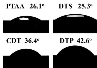
**Figure S8.** Pictures of DMF contact angle ( $\theta_{\text{DMF}}$ ) on the films of PTAA, DTS, CDT and DTP.
