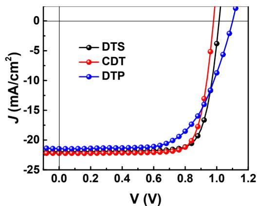
**Figure S7.**  $J$ - $V$  curves for devices fabricated with DTS, CDT and DTP.
