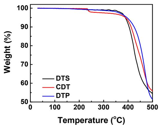
**Figure S5.** Thermogravimetric analysis (TGA) of DTS, CDT and DTP.
