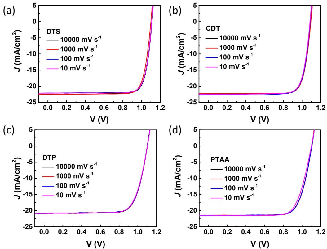
**Figure S10.**  $J$ - $V$  curves of the devices based on HTL/PSBMA/CH<sub>3</sub>NH<sub>3</sub>PbI<sub>3</sub>/C<sub>60</sub>/BAP/Ag at different scan speed.
