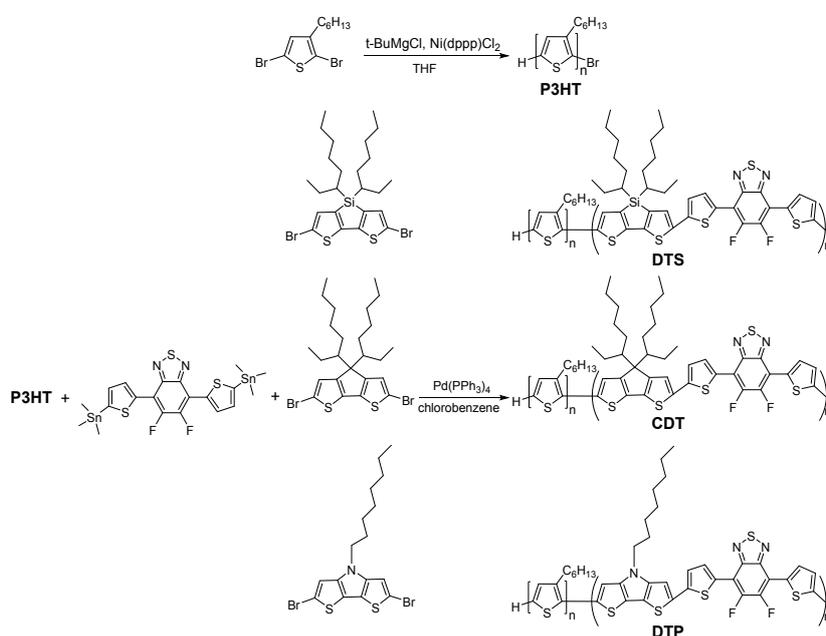
**Scheme S1** Synthetic routes of pre-polymer P3HT and the copolymers DTS, CDT, DTP.
