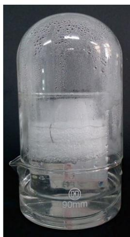
Fig. S12. Photograph of the solar desalination device for collecting purified water. Vapor condenses on the wall of glass and water flows to the bottom.
