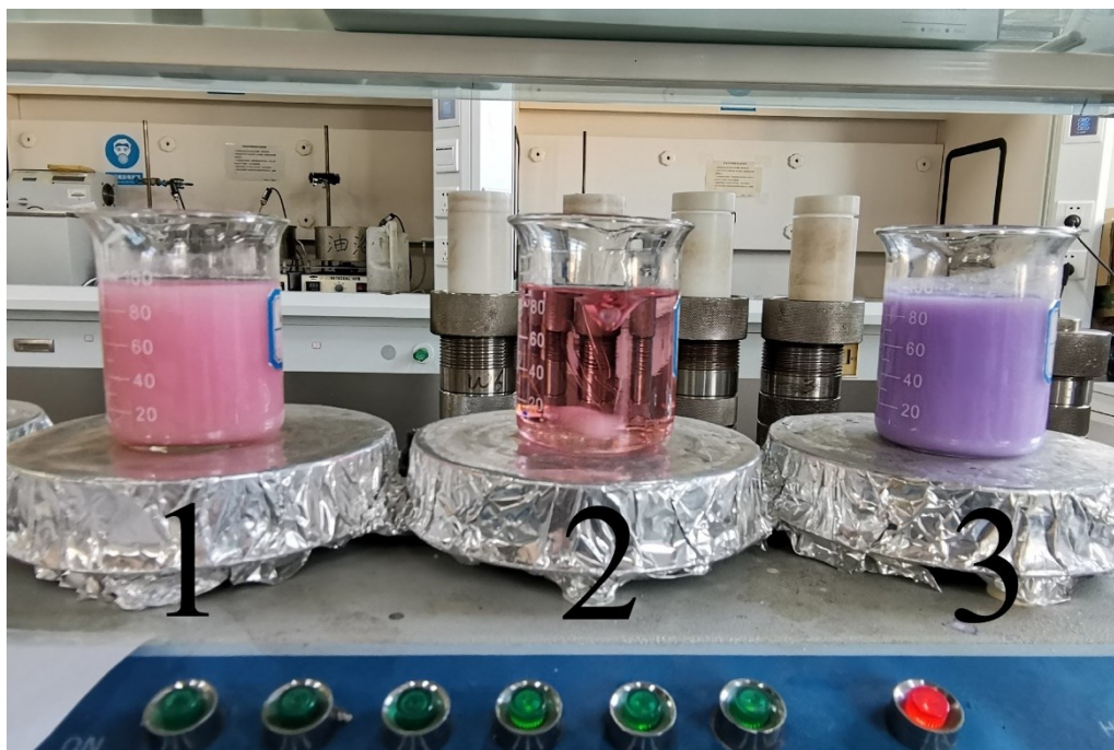
Figure S1 The photograph of different reaction systems. (1) Ammonium tungstate [(\text{NH}_4)_{10}\text{W}_{12}\text{O}_{41} \cdot x\text{H}_2\text{O}] as W source; (2) Ammonium paratungstate [(\text{NH}_4)_{10}\text{H}_2\text{W}_{12}\text{O}_{42} \cdot x\text{H}_2\text{O}] as W source; (3) Sodium tungstate ( \text{Na}_2\text{WO}_4 ) as W source.
