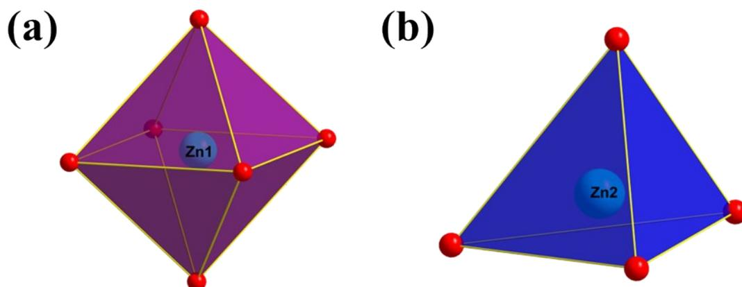
**Fig. S3.** Polyhedral representation of the coordination sphere of the Zn<sup>2+</sup> center in **kgd-Zn** (water molecules and hydrogen atoms are omitted for clarity).
