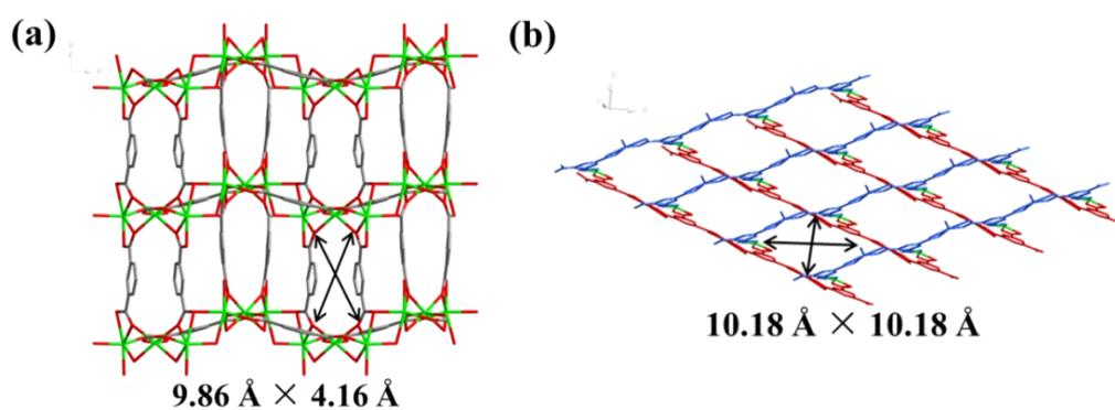
**Fig. S1.** (a) 2D layer of **sql-M** and a square pore structure with a size of 9.86 Å × 4.16 Å; (b) 2D layer of **kia-M** and a square pore structure with a size of 10.18 Å × 10.18 Å.
