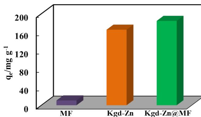
**Fig. S17.** Adsorption uptakes of CIP by MF, **kgd-Zn** and **kgd-Zn@MF**.
