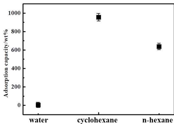
**Fig. S21.** Adsorption capacities of **kgd-Zn** toward water, hexane and cyclohexane.
