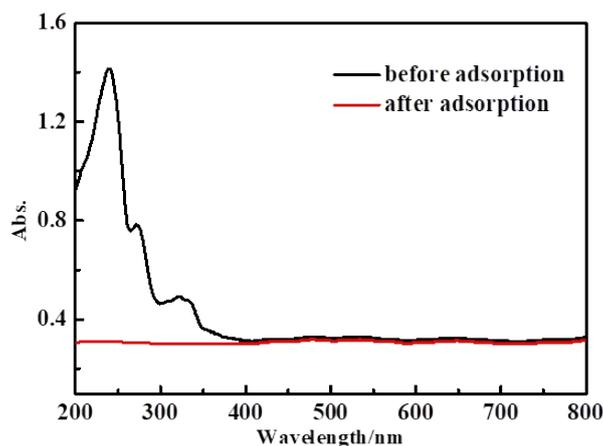
**Fig. S24.** UV-Vis spectra of the simulated wastewater containing 5 mg·L<sup>-1</sup> CIP and 1 vol% soybean oil before and after filtration.
