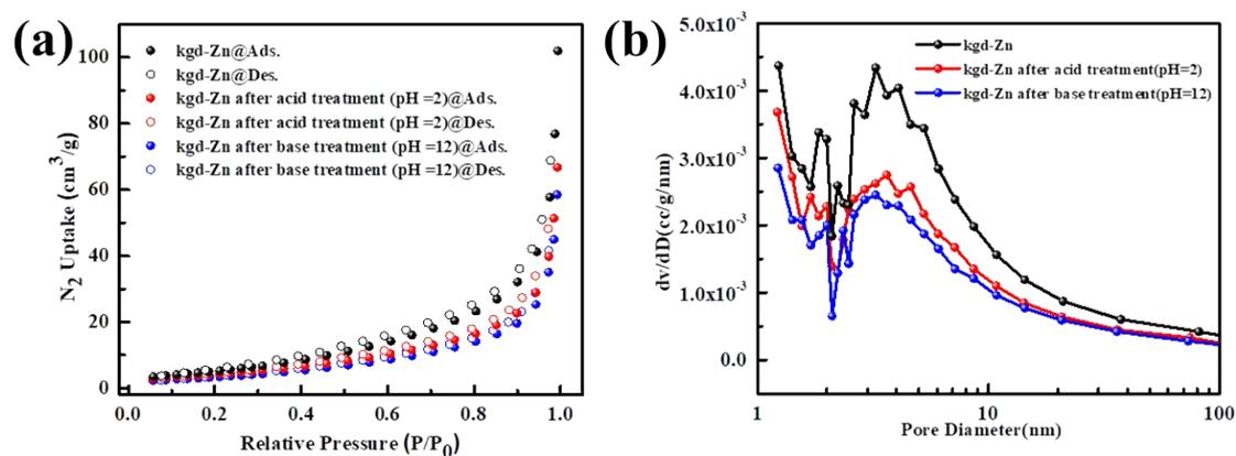
**Fig. S6.** (a)  $N_2$  adsorption/desorption isotherms of **kgd-Zn** after treated in the NaOH solution (pH=12) and HCl solutions (pH=2), respectively, at 77 K; (b) DFT pore size distribution for the corresponding MOFs.
