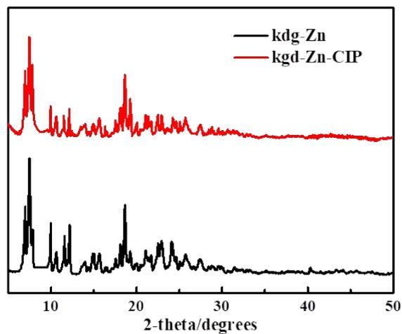
Fig. S7. The PXRD pattern of **kgd-Zn** before and after CIP adsorption.
