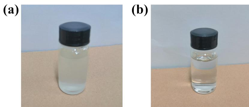
**Fig. S22.** Photographs of simulated wastewater containing 1 vol% soybean oil, 5 mg·L<sup>-1</sup> CIP (a) before and (b) after filtration.
