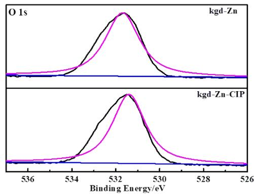
**Fig. S13.** O 1s spectra of **kgd-Zn** before (upper lines) and after (lower lines) adsorption.
