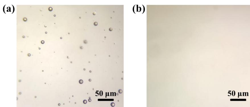
**Fig. S19.** The microscopy images of the soybean oil/water mixture (a) after and (b) before filtration.
