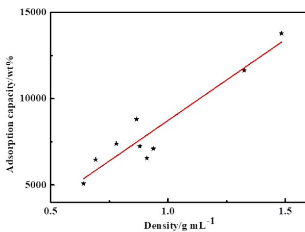
**Fig. S20.** Adsorption capacities of **kgd-Zn@MF** measured for a range of oils and organic solvents in terms of the solvent densities.
