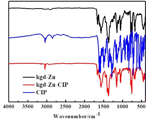
**Fig. S11.** FTIR spectra of CIP, **kgd-Zn** and **kgd-Zn** adsorbed CIP.
