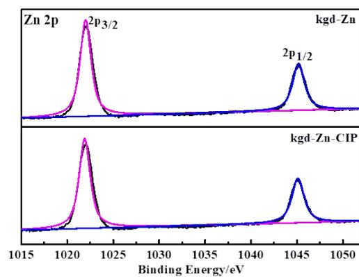
**Fig. S14.** Zn 2p spectra of **kgd-Zn** before (upper lines) and after (lower lines) adsorption.
