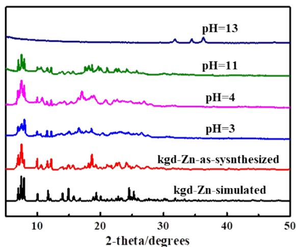
**Fig. S5.** The PXRD patterns of samples after soaked in acid or basic solutions, respectively.
