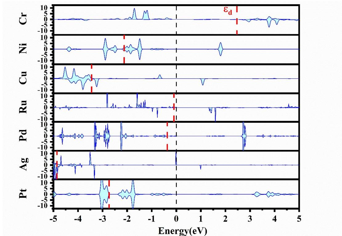
Fig. S8. Projected density of states (PDOS) for the d-orbital of single-TM-atom in 2D TM-TAA MOFs with M=Cr, Ni, Cu, Ru, Pd, Ag, Pt. The vertical dash dotted lines correspond to the Fermi level which is shifted to zero.
