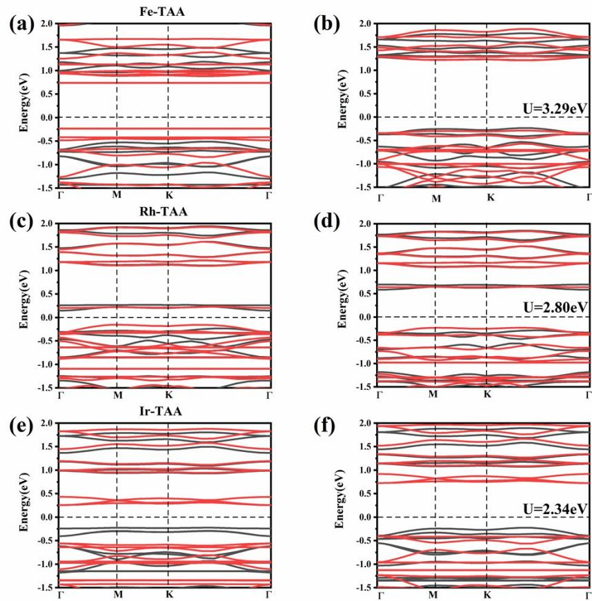
Fig.S3. The band structures with and without U of Fe-, Rh- and Ir-TAA MOF monolayers. The energy at the Fermi level was set to zero.
