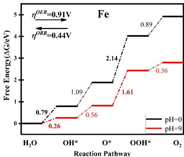
Fig. S6. Free energy diagram of Fe-TAA MOF obtained by involving solvent effect.
