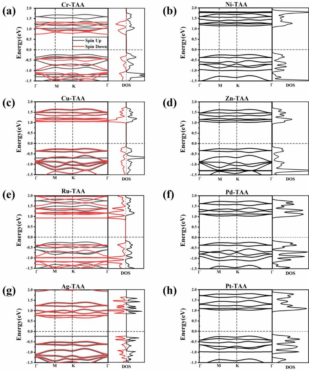
Fig. S2. Electronic band structures of the TM-TAA MOFs with TM = Ni, Cu, Zn, Ru, Rh, Pd, Cr, Pt. The energy at the Fermi level was set to zero.
