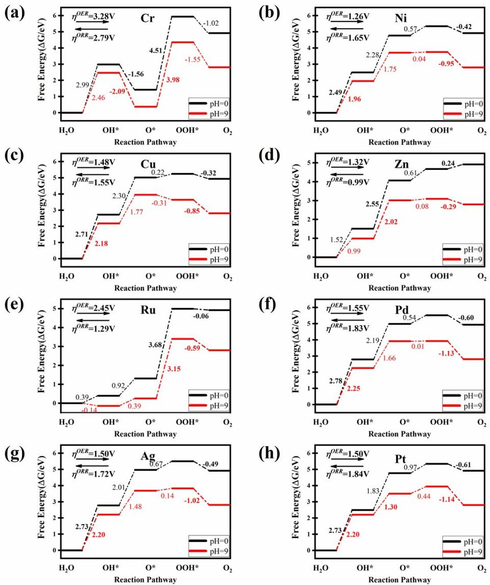
Fig. S5. Free energy figures for the OER and ORR process on TM site of (a) Cr-TAA, (b) Ni-TAA, (c) Cu-TAA, (d) Zn-TAA, (e) Ru-TAA, (f) Pd-TAA, (g) Ag-TAA and (h) Pt-TAA MOF at zero potential ( $U = 0$ ), where the elementary reaction with  $\Delta G$  in bold represent the potential-determining step for OER and ORR.
