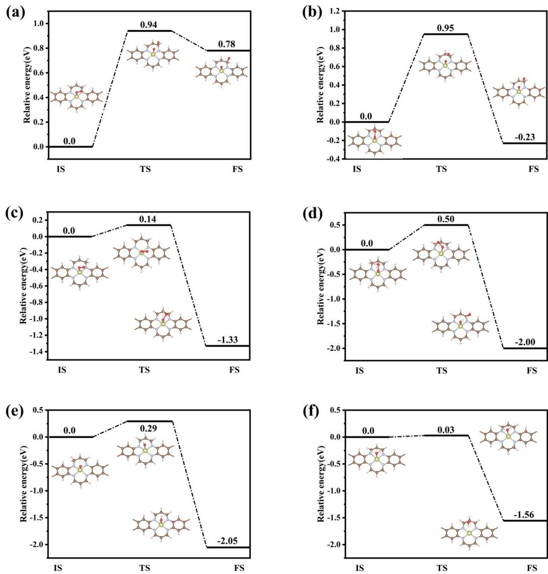
Fig.S7. The structures of the initial state (IS), transition state (TS), final state (FS) and potential energy profile for (a)  $O_2^* \rightarrow O^* + O^*$ , (b)  $OOH^* \rightarrow OH^* + O^*$ , (c)  $O_2^* + H^+ \rightarrow OOH^*$ , (d)  $OOH^* + H^+ \rightarrow O^* + H_2O$ , (e)  $O^* + H^+ \rightarrow OH^*$  and (f)  $OH^* + H^+ \rightarrow H_2O^*$  on Ir-TAA MOF.
