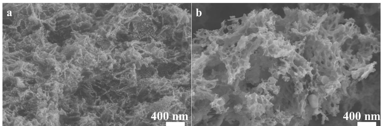
**Figure S3** SEM images of P(St-co-4VP)@PAN-derived carbon materials with different PAN loading via the bidirectional anchoring method. (a) 0.04 g. (b) 0.08 g.
