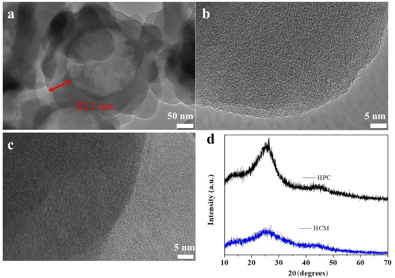
**Figure S8** (a) TEM image of HPC with hollow structure. (b) HRTEM image of HPC. (c) HRTEM image of HCM. (d) Wide-angle PXRD patterns of HCM and HPC.
