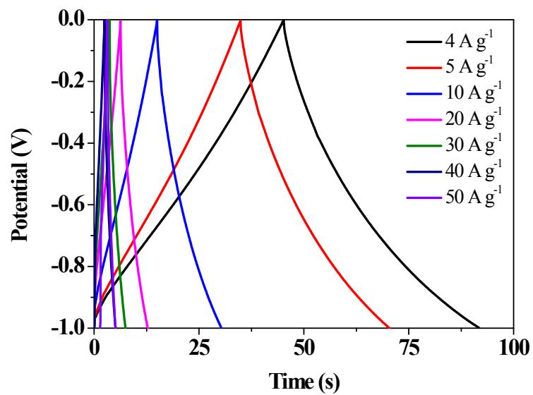
**Figure S6** GCD curves of CPCS with current densities ranging from 4 to 50  $\text{A g}^{-1}$ .
