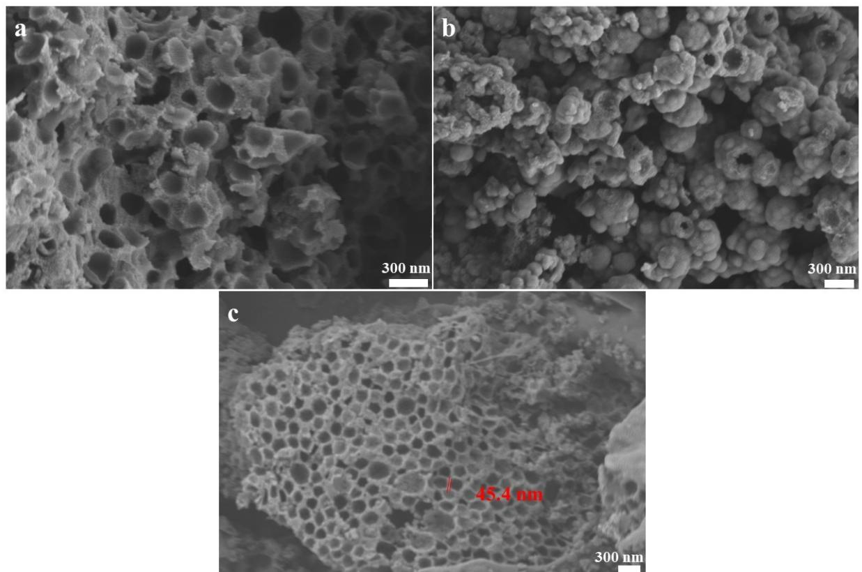
**Figure S2** SEM images of P(St-co-4VP)@PAN-based carbons obtained via the template method. (a,c) honeycomb structure. (b) hollow structure.
