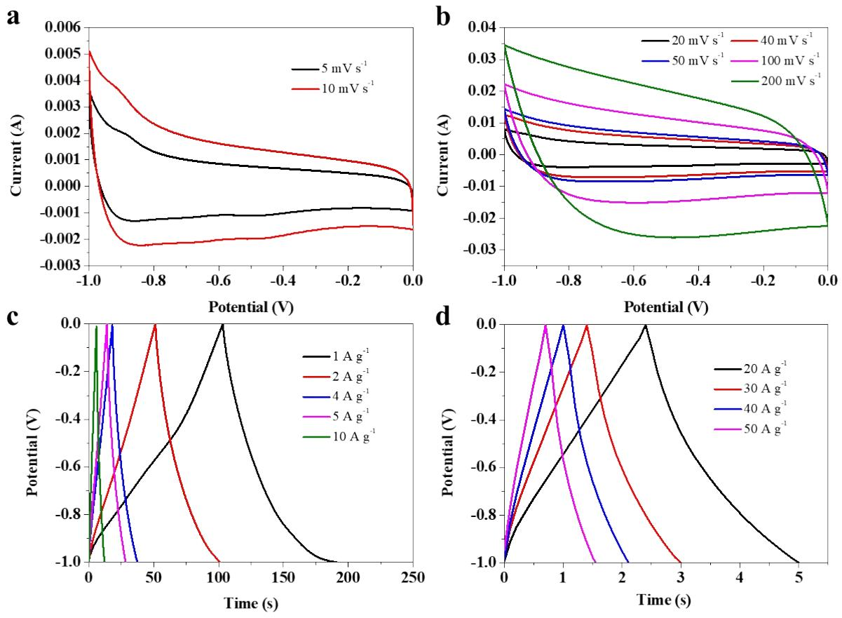
**Figure S9** (a-b) CV curves of C4VP at different scan rates. (c-d) GCD curves of C4VP at different current densities.
