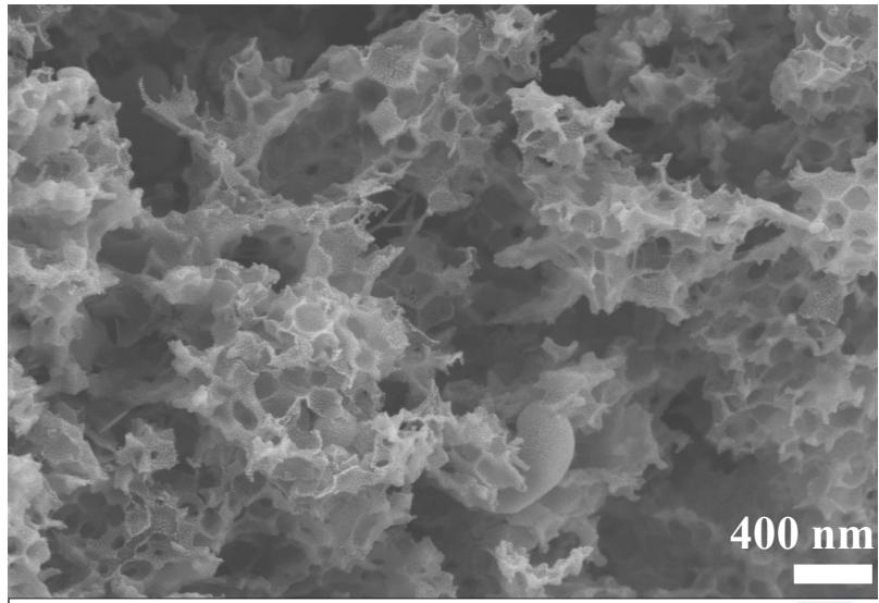
**Figure S4** SEM image of CPCS treated at 950 °C.
