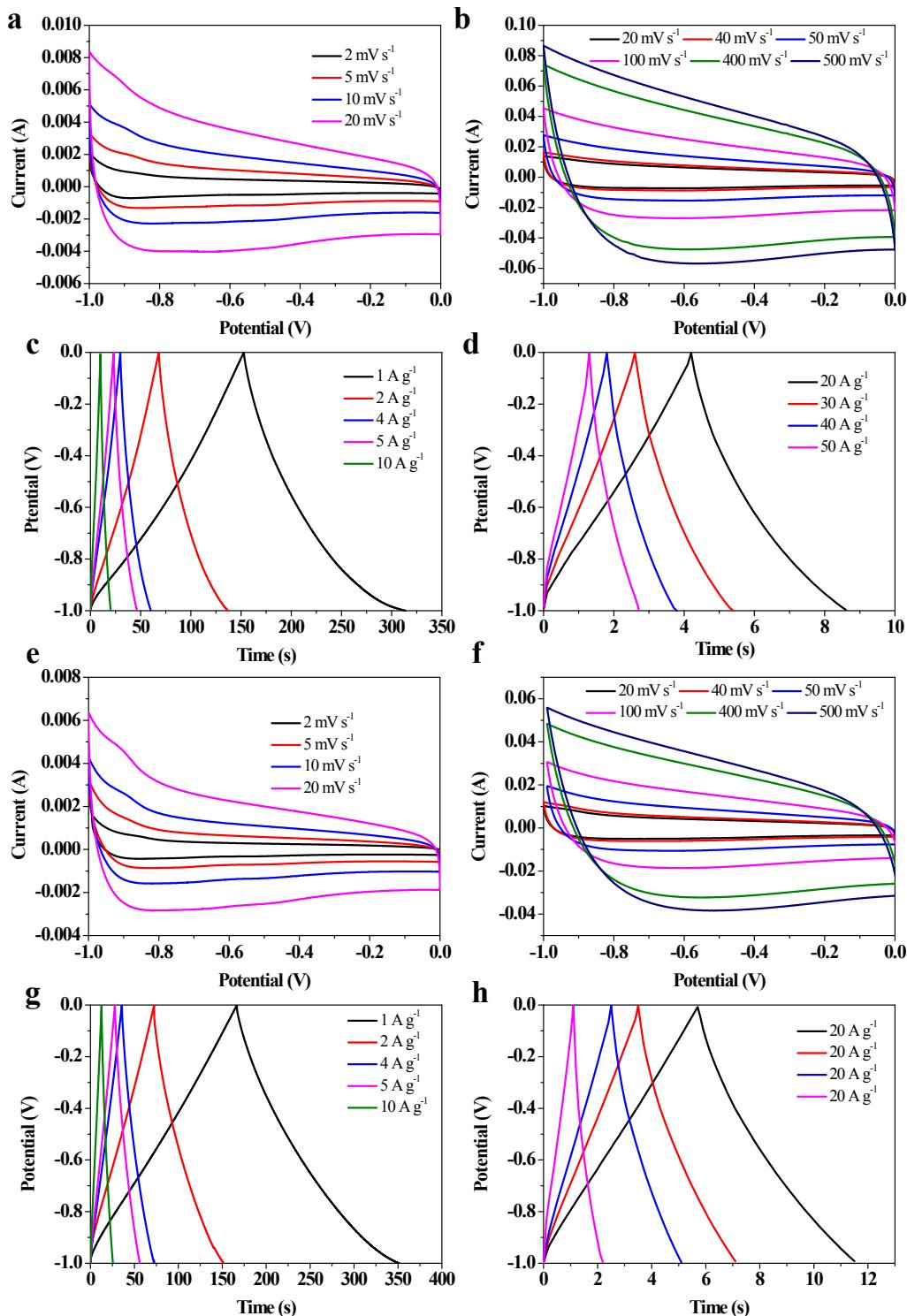
**Figure S7** (a-b) CV curves of HCM at different scan rates. (c-d) GCD curves of HCM at different current densities. (e-f) CV curves of HPC at different scan rates. (g-h) GCD curves of HPC at different current densities.
