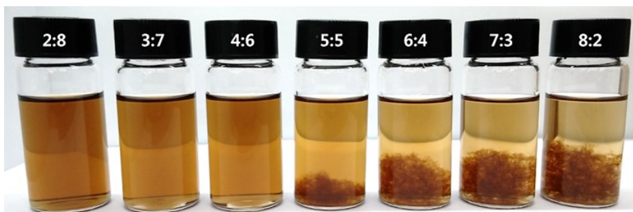
Fig. S1. Dispersion characteristics of GO at various IPA–DI water mixture ratios (e.g., 2 (IPA) : 8 (DI water) ~ 8 : 2).
