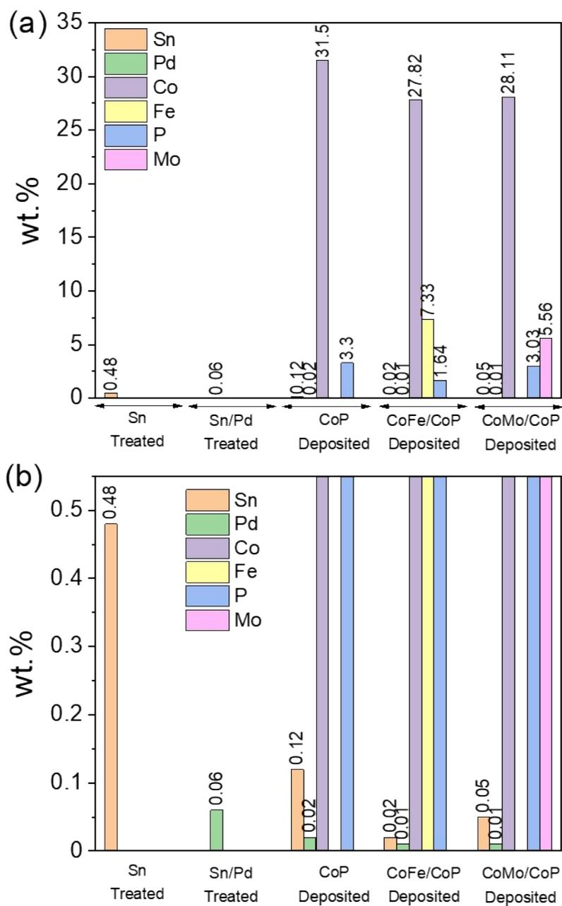
**Figure S8:** (a-b) ICP-MS data showing the wt.% of elements Sn, Pd, Co, P, Fe, and Mo.
