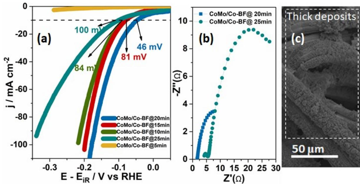
**Figure S13.** (a) The HER performance of the CoMo/Co-BF electrodes with respect to the catalyst loading (5, 10, 15, 20 and 25 min of loading, refer experimental section), (b) electrochemical impedance spectroscopy of electrodes with 20 min and 25 min deposition with optimum catalyst loading, (c) SEM micrograph of CoMo/Co-BF with maximum deposition time used showing thick deposits on the Co-BF.
