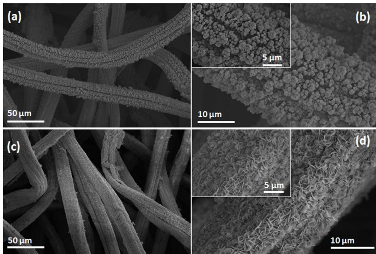
**Figure S12.** The FE-SEM micrographs of (a, b) anode (CoFe/Co-BF) and (c, d) cathode (CoMo/Co-BF) after prolonged electrolysis at a high current density ( $200 \text{ mA cm}^{-2}$ ) showed increased roughness due to aging effect.
