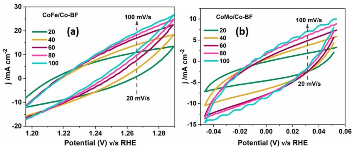
**Figure S9.** ECSA estimation determined from  $C_{dl}$ . (a,b) CV cycle recorded in non-faradic region at different scan rates for CoFe/Co-BF and CoMo/Co-BF.
