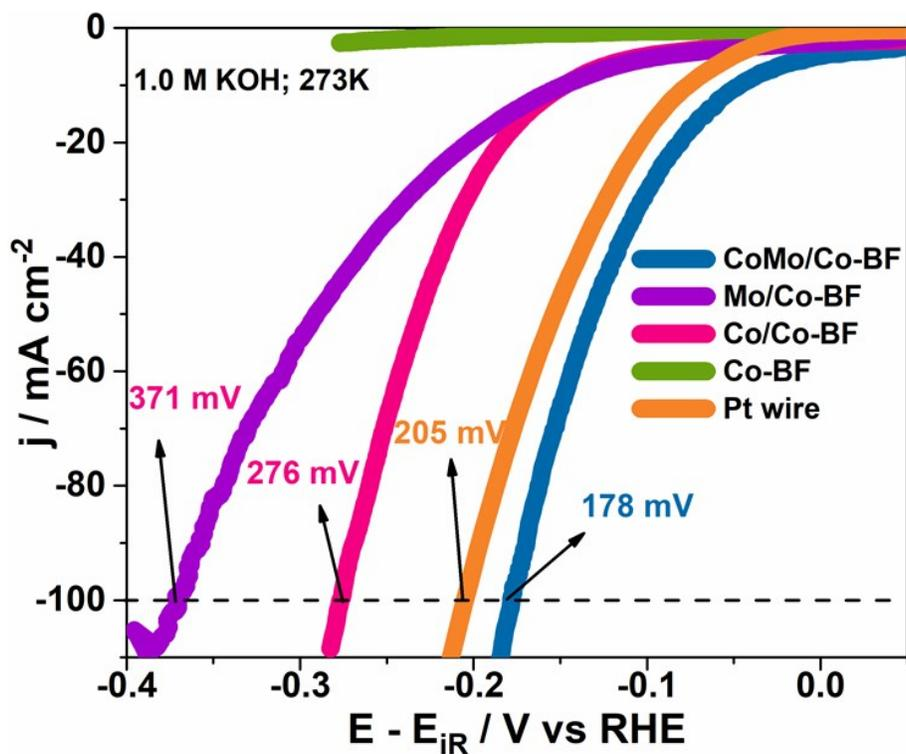
**Figure S10.** Overpotential at high current density from iR corrected polarization curves of CoMo/Co-BF, Co/Co-BF, Mo/Co-BF and Co-BF recorded at scan rate of 5mV s<sup>-1</sup>.
