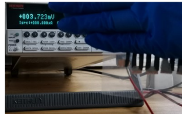
Figure S6 Output voltage testing of the original fabricated device three times after over 170 days.
