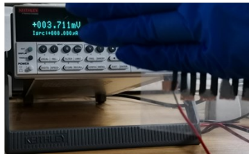
Figure S6 Output voltage testing of the original fabricated device three times after over 170 days.
