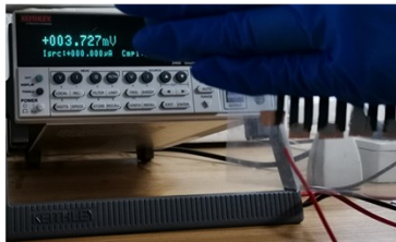
Figure S6 Output voltage testing of the original fabricated device three times after over 170 days.
