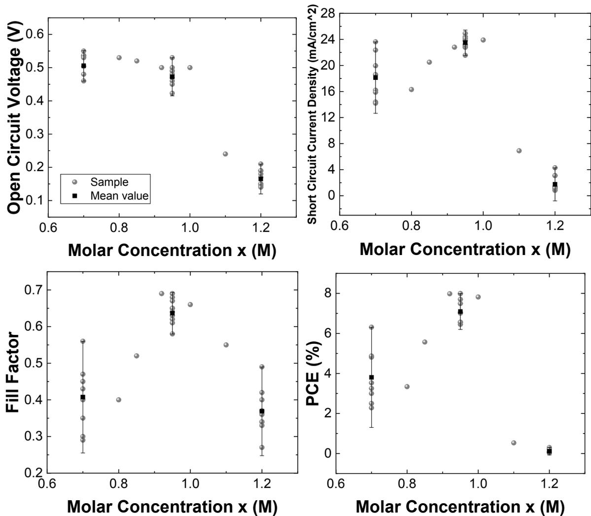
**Figure S8.** Statistics for  $V_{OC}$ ,  $J_{SC}$ , FF and PCE of devices with an active area of  $0.04 \text{ cm}^2$ . Note that: for the 0.70 M composition 8 samples were measured, for the 0.95 M composition 9 samples, and for the 1.20 M composition also 9 samples were measured. The graph includes the values from Table 1.
