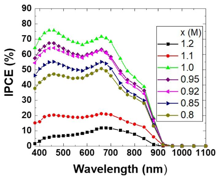
Figure S11. IPCE measurements of ITO/PEDOT:PSS/ PEA<sub>0.08</sub>FA<sub>(x)</sub>SnI<sub>3</sub>/C60/BCP/Al devices.
