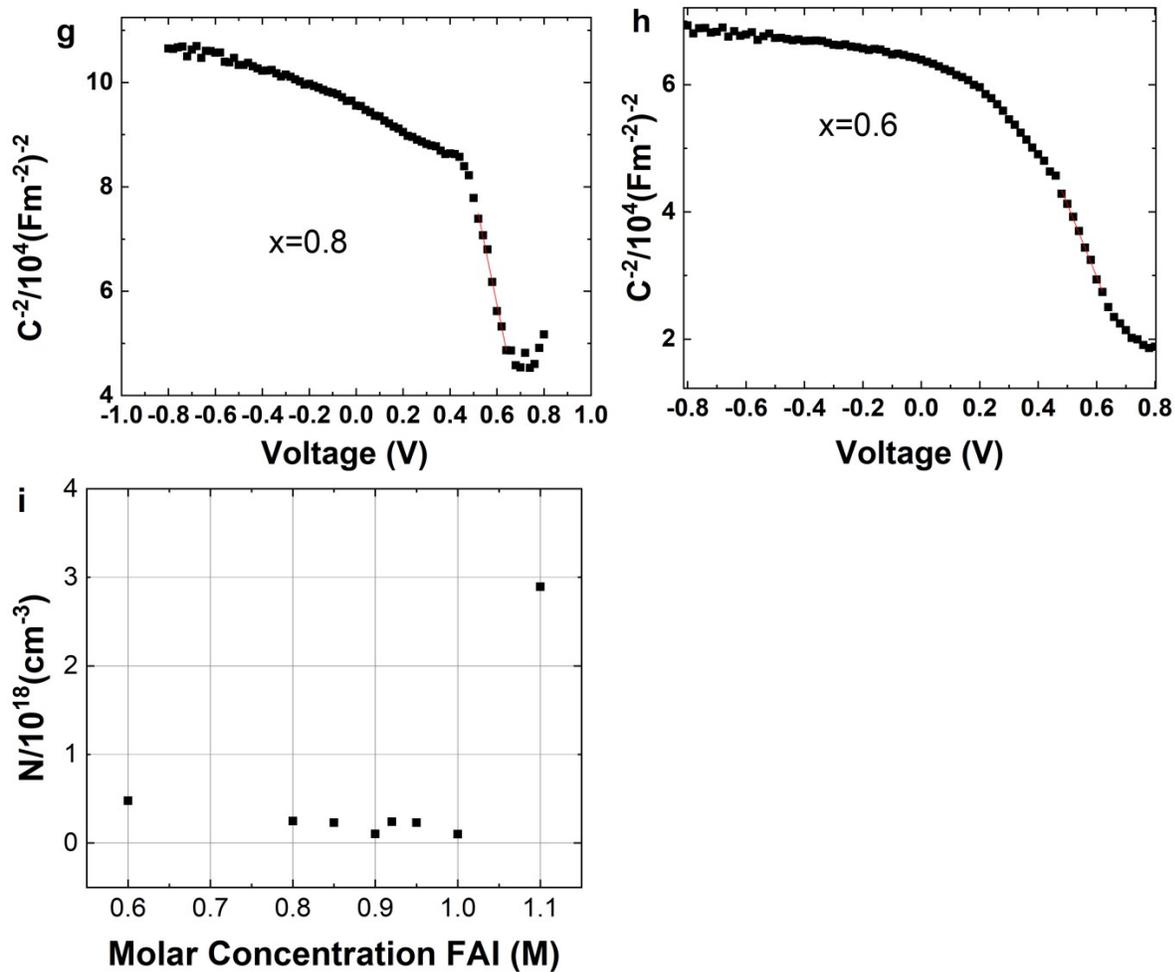
**Figure S7.** Mott-Schottky analysis of perovskite solar cells of different stoichiometry. (a-h)  $C^{-2}$  as a function of bias voltage. (i) carrier concentration as derived from Mott-Schottky analysis for the different samples.
