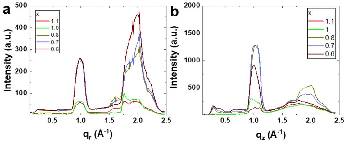
**Figure S3.** The line-cut data in (a) in-plane ( $q_z$ ) and (b) out-of-plane ( $q_y$ ) of the GIWAXS images of the  $\text{PEA}_{0.08}\text{FA}_x\text{SnI}_3$  films with X-ray incident angle of  $0.25^\circ$ , respectively.
