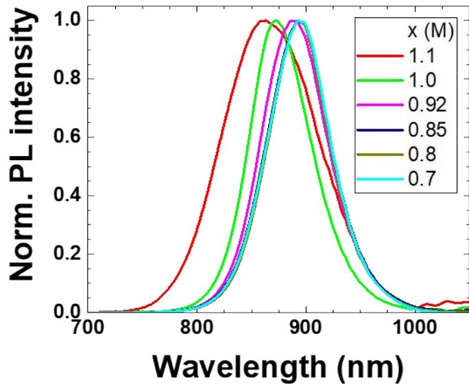
Figure S5. Normalized PL spectra of  $\text{PEA}_{0.08}\text{FA}_x\text{SnI}_3$  films.
