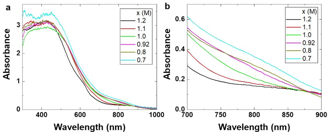
**Figure S6.** Absorbance of PEA<sub>0.08</sub>FA<sub>(x)</sub>SnI<sub>3</sub> films (a) with an incident light wavelength from 350 nm to 1000 nm and (b) from 700 nm to 900 nm. Note: the absorbance spectra in the short wavelength region (<600 nm) are saturated.
