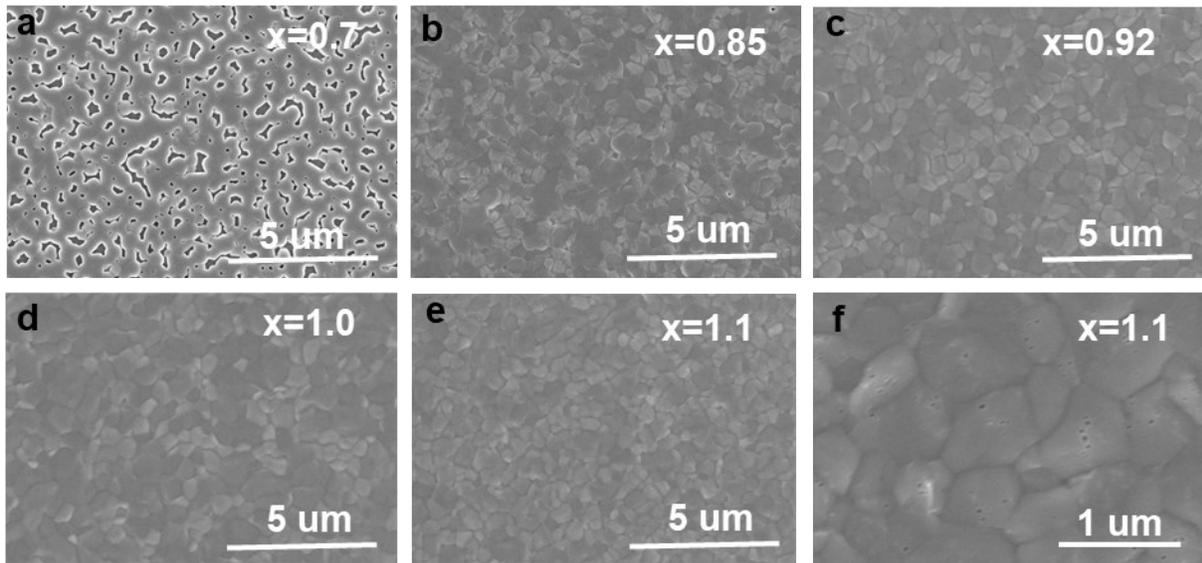
Figure S4. SEM images of the  $\text{PEA}_{0.08}\text{FA}_x\text{SnI}_3$  films: (a)  $x=0.7$ , (b)  $x=0.85$ , (c)  $x=0.92$ , (d)  $x=1.0$ , (e)  $x=1.1$ , (f) the magnified image of  $x=1.1$  sample.
