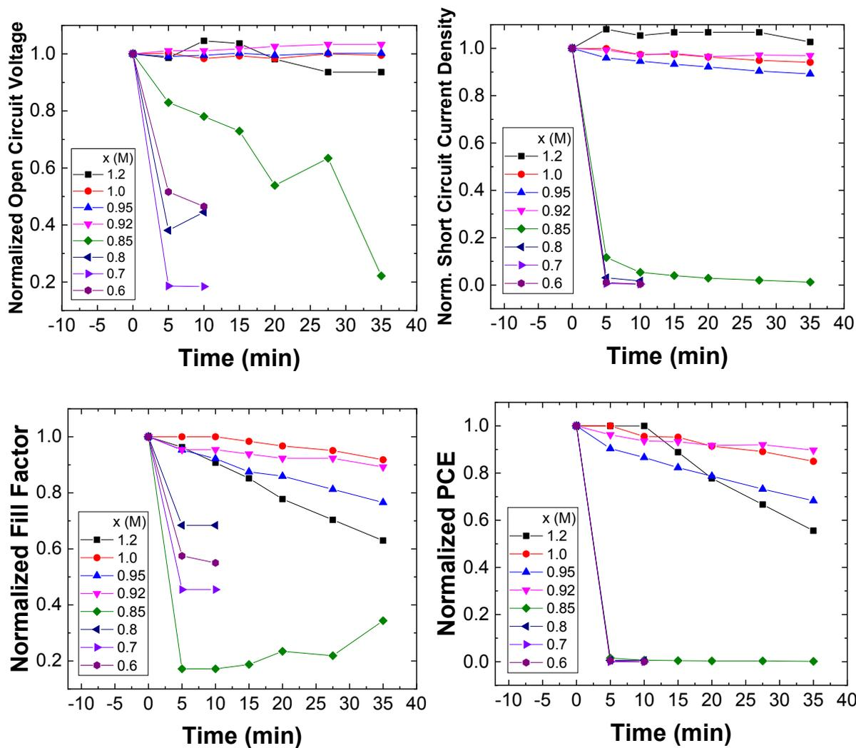
Figure 12. Variation of the  $V_{OC}$ ,  $J_{SC}$ , FF and PCE of devices using different 2D/3D films vs time they have been exposed to air.
