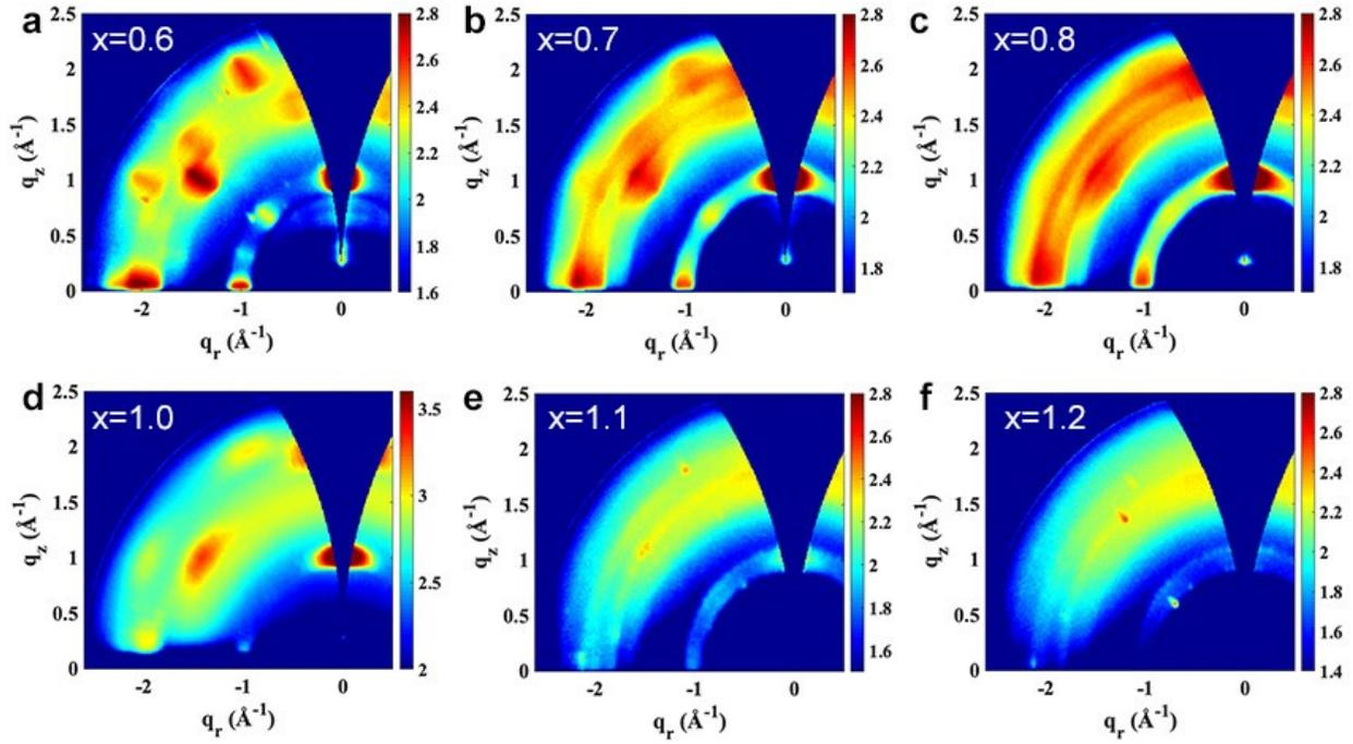
**Figure S2.** GIWAXS patterns of  $\text{PEA}_{0.08}\text{FA}_{(x)}\text{SnI}_3$  films. The images were recorded using an incident angle of  $0.25^\circ$ .
