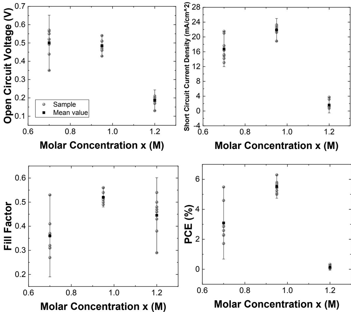
**Figure S10.** Statistics for  $V_{OC}$ ,  $J_{SC}$ , FF and PCE of devices using different 2D/3D films with an active area of  $0.25 \text{ cm}^2$ . Note that: for the 0.70 M composition 8 samples were measured, for the 0.95 M composition 9 samples, and also for the 1.20 M composition 9 samples were measured.
