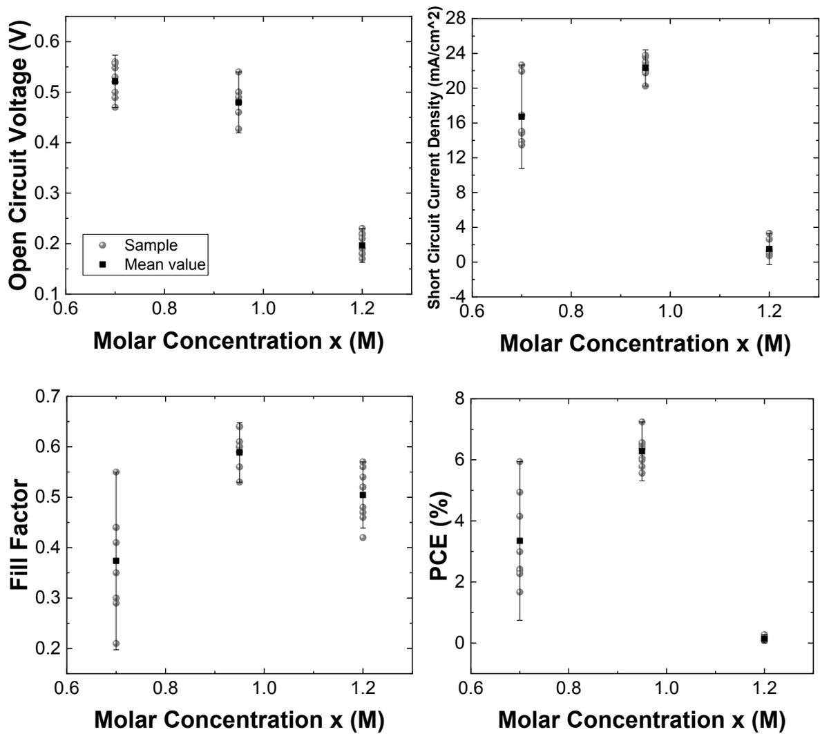
**Figure S9.** Statistics for  $V_{OC}$ ,  $J_{SC}$ , FF and PCE of devices with an active area of  $0.09 \text{ cm}^2$ . Note that: for the 0.70 M composition 8 samples were measured, for the 0.95 M composition 9 samples, and also for the 1.20 M composition 9 samples were measured.
