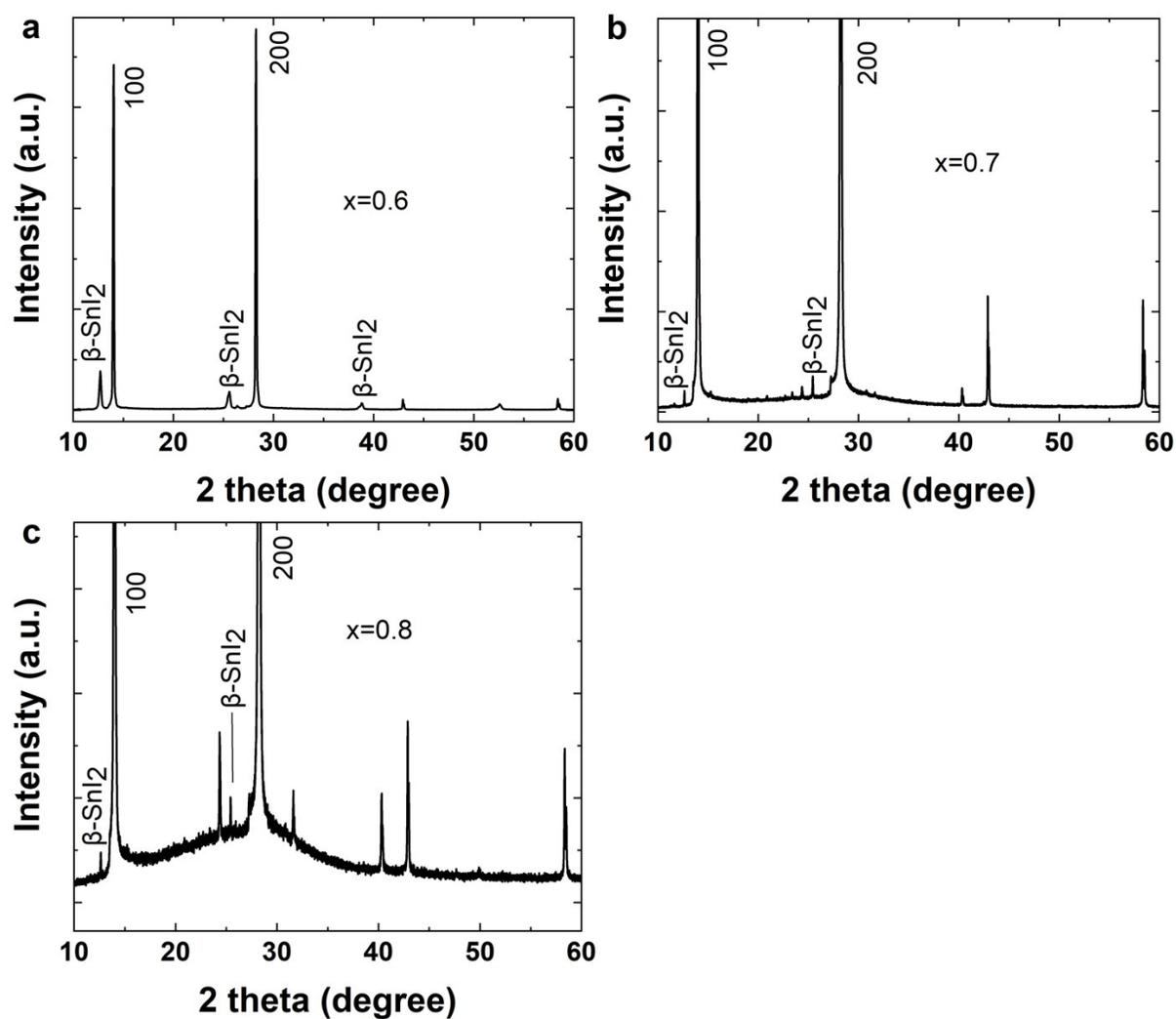
**Figure S1.** XRD patterns of (a) a PEA<sub>0.08</sub>FA<sub>0.6</sub>SnI<sub>3</sub> film with hexagonal SnI<sub>2</sub> (β-SnI<sub>2</sub>) peaks at 12.7°, 25.6°, and 38.8°, (b) a PEA<sub>0.08</sub>FA<sub>0.7</sub>SnI<sub>3</sub> film with β-SnI<sub>2</sub> peaks at 12.7° and 25.6° and (c) a PEA<sub>0.08</sub>FA<sub>0.8</sub>SnI<sub>3</sub> film with β-SnI<sub>2</sub> peaks at 12.7° and 25.6° as well [1].
