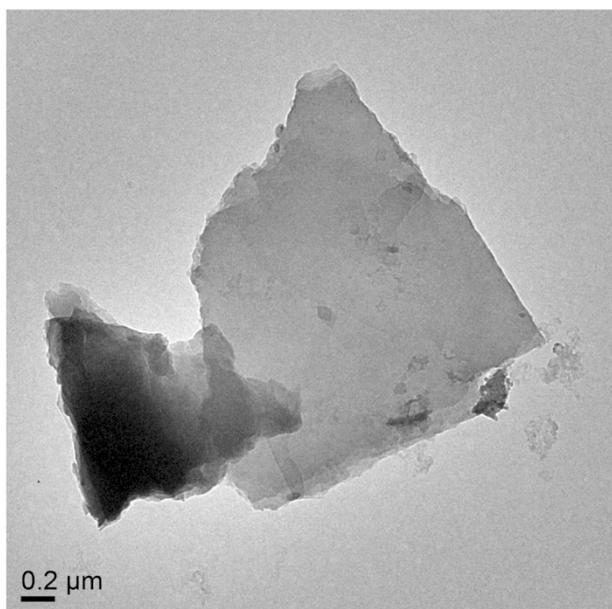
Figure S7. TEM image of PC<sub>61</sub>BM/CuTCPP-1.8% sheet.
