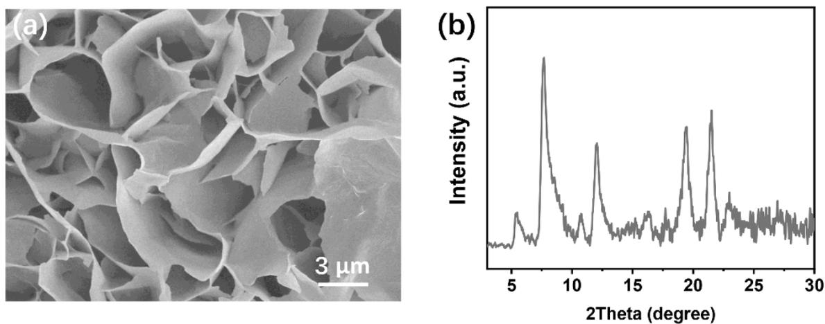
Figure S17. (a) SEM image and (b) powder XRD pattern of PC<sub>61</sub>BM/CuTCPP-1.8% film after the catalysis.
