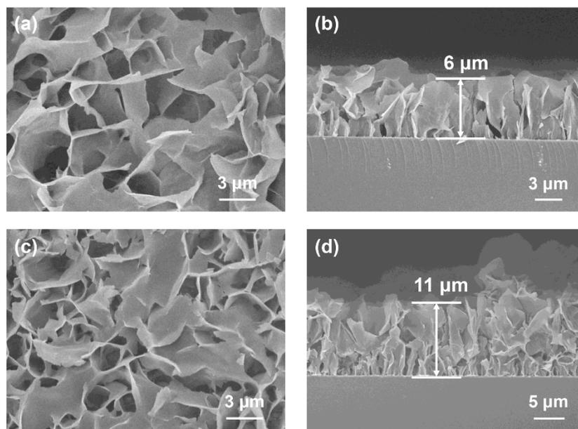
Figure S15. SEM images of (a) surface and (b) cross-section of PC<sub>61</sub>BM/CuTCPP-1.8%-6 μm, and (c) surface and (d) cross-section of PC<sub>61</sub>BM/CuTCPP-1.8%-11 μm.
