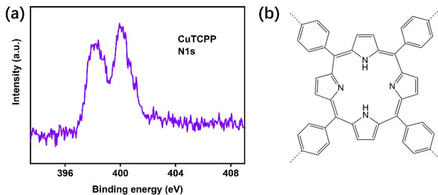
Figure S13. (a) XPS N1s spectrum of CuTCPP film. The two major peaks indicate that there are two status N atoms, as shown in (b).
