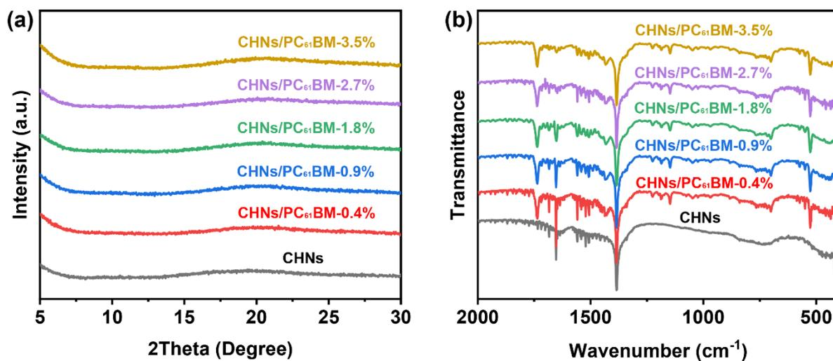
Figure S3. (a) Powder XRD patterns and (b) FTIR spectra of CHNs/PC<sub>61</sub>BM films.
