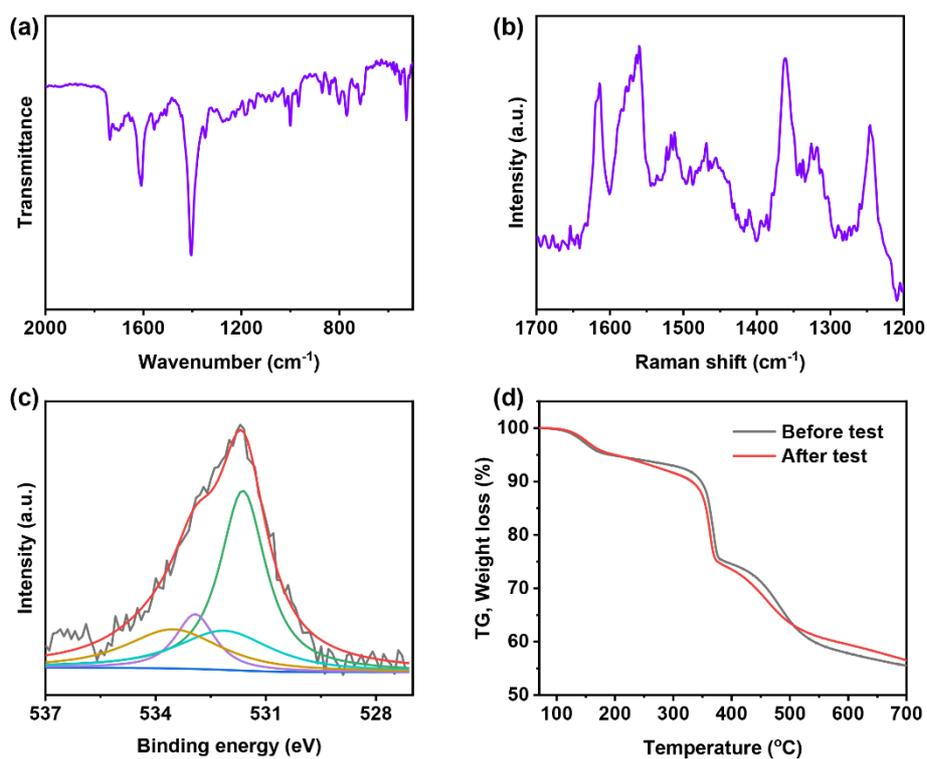
Figure S18. (a) FTIR spectrum, (b) Raman spectrum, (c) XPS O1s spectrum, and (d) TGA curve of PC<sub>61</sub>BM/CuTCPP-1.8% film after the catalysis.
