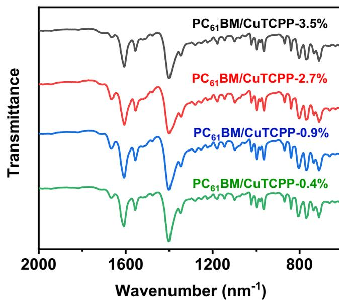
Figure S10. FT-IR spectra of PC<sub>61</sub>BM/CuTCPP films with various PC<sub>61</sub>BM concentrations.
