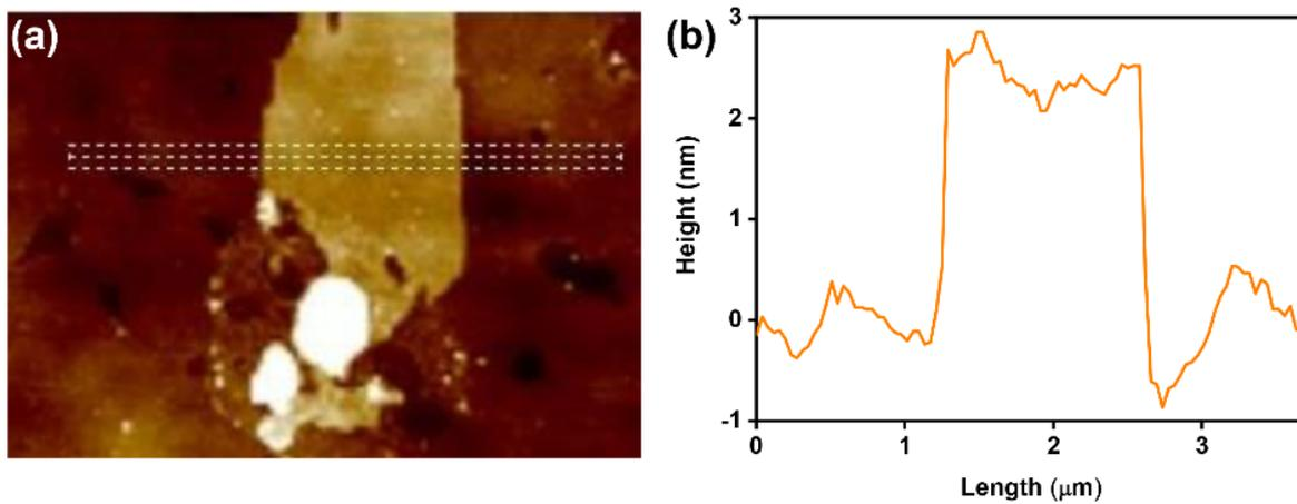
Figure S6. (a) AFM image of 2D PC<sub>61</sub>BM/CuTCPP-1.8% sheet. (b) Height of PC<sub>61</sub>BM/CuTCPP-1.8% sheet.
