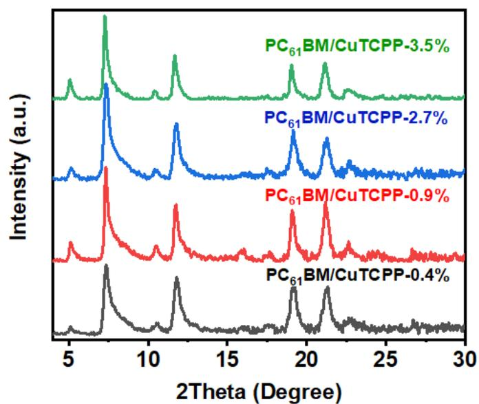
Figure S9. Powder XRD patterns of PC<sub>61</sub>BM/CuTCPP films with various PC<sub>61</sub>BM concentrations.
