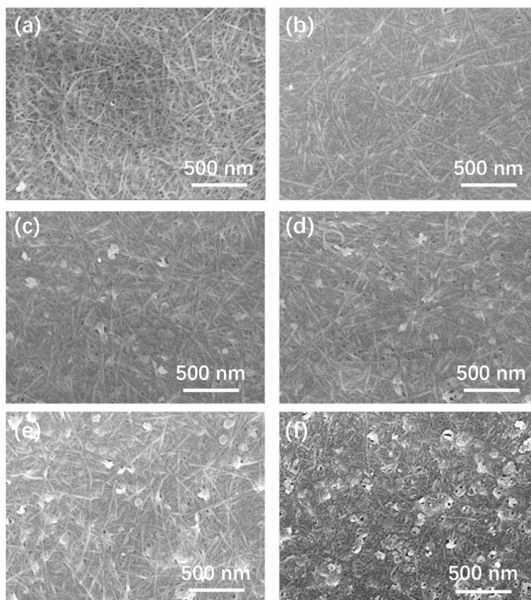
Figure S2. SEM images for surface of (a) CHNs film, (b) CHNs/PC<sub>61</sub>BM-0.4% film, (c) CHNs/PC<sub>61</sub>BM-0.9% film, (d) CHNs/PC<sub>61</sub>BM-1.8% film, (e) CHNs/PC<sub>61</sub>BM-2.7%, and (f) CHNs/PC<sub>61</sub>BM-3.5% film.
