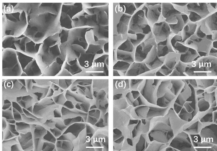
Figure S5. SEM images for surface of (a) PC<sub>61</sub>BM/CuTCPP-0.4% film, (b) PC<sub>61</sub>BM/CuTCPP-0.9% film, (c) PC<sub>61</sub>BM/CuTCPP-2.7% film, and (d) PC<sub>61</sub>BM/CuTCPP-3.5% film.
