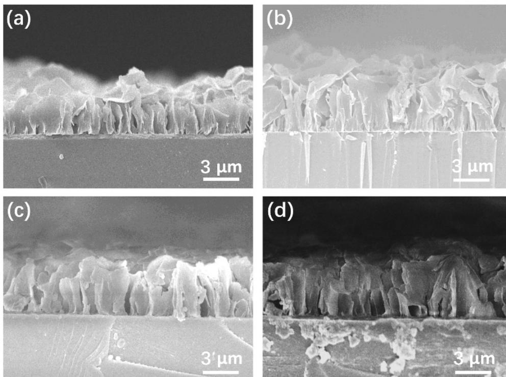
Figure S8. SEM images for cross-section of (a) PC<sub>61</sub>BM/CuTCPP-0.4% film, (b) PC<sub>61</sub>BM/CuTCPP-1.8% film, (c) PC<sub>61</sub>BM/CuTCPP-2.7% film, and (d) PC<sub>61</sub>BM/CuTCPP-3.5% film.
