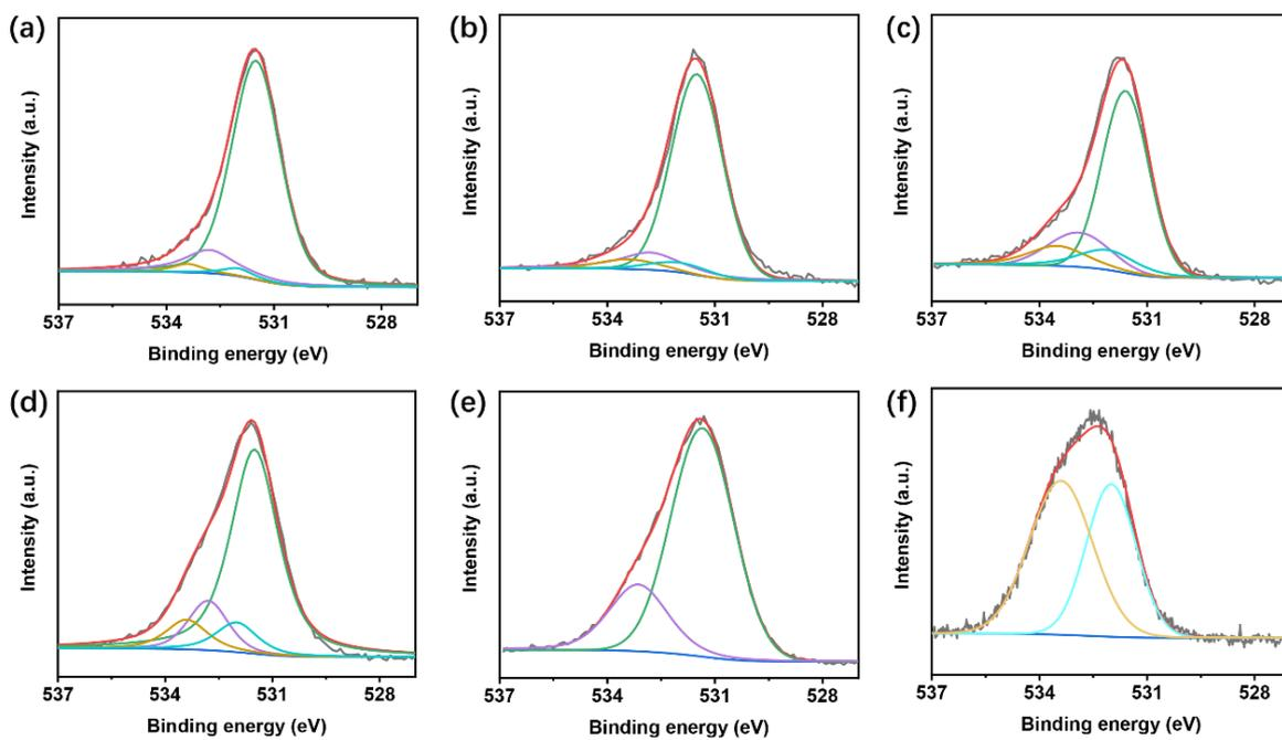
Figure S12. XPS O1s spectra of (a) PC61BM/CuTCPP-0.4% film, (b) PC61BM/CuTCPP-0.9% film, (c) PC61BM/CuTCPP-2.7% film, (d) PC61BM/CuTCPP-3.5% film, (e) CuTCPP film, and (f) PC61BM.
