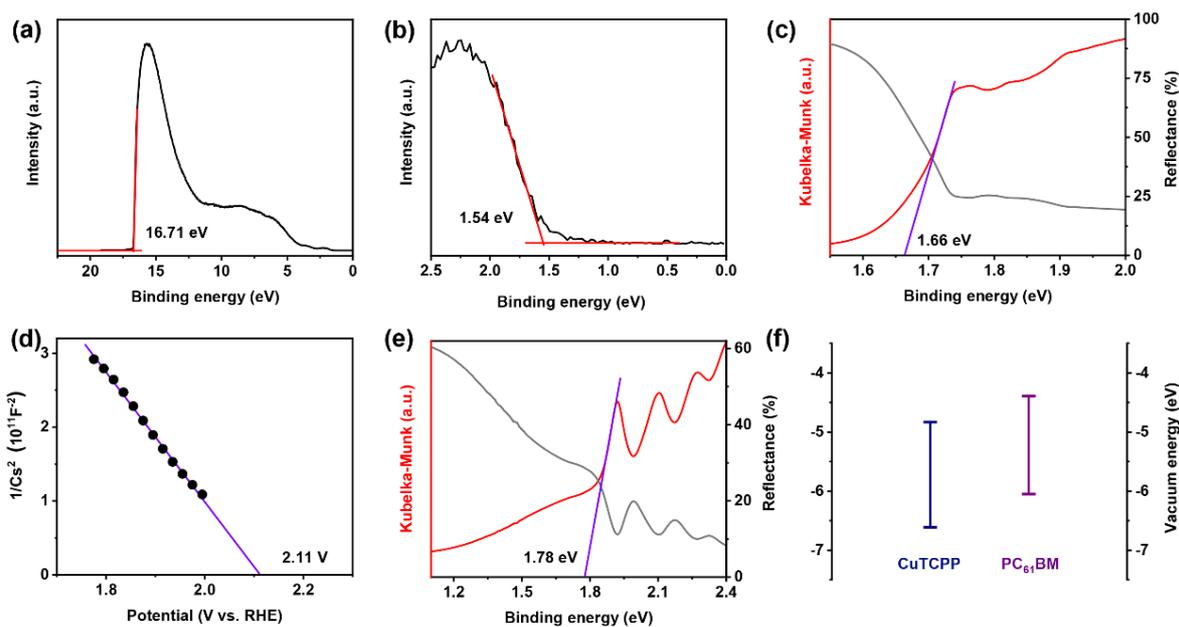
Figure S14. (a) UPS, (b) VBM and (c) UV-vis-DRS of PC<sub>61</sub>BM. (d) Mott-Schottky plot and (e) UV-vis-DRS of CuTCPP film. (f) Band structures of PC<sub>61</sub>BM and CuTCPP film.
