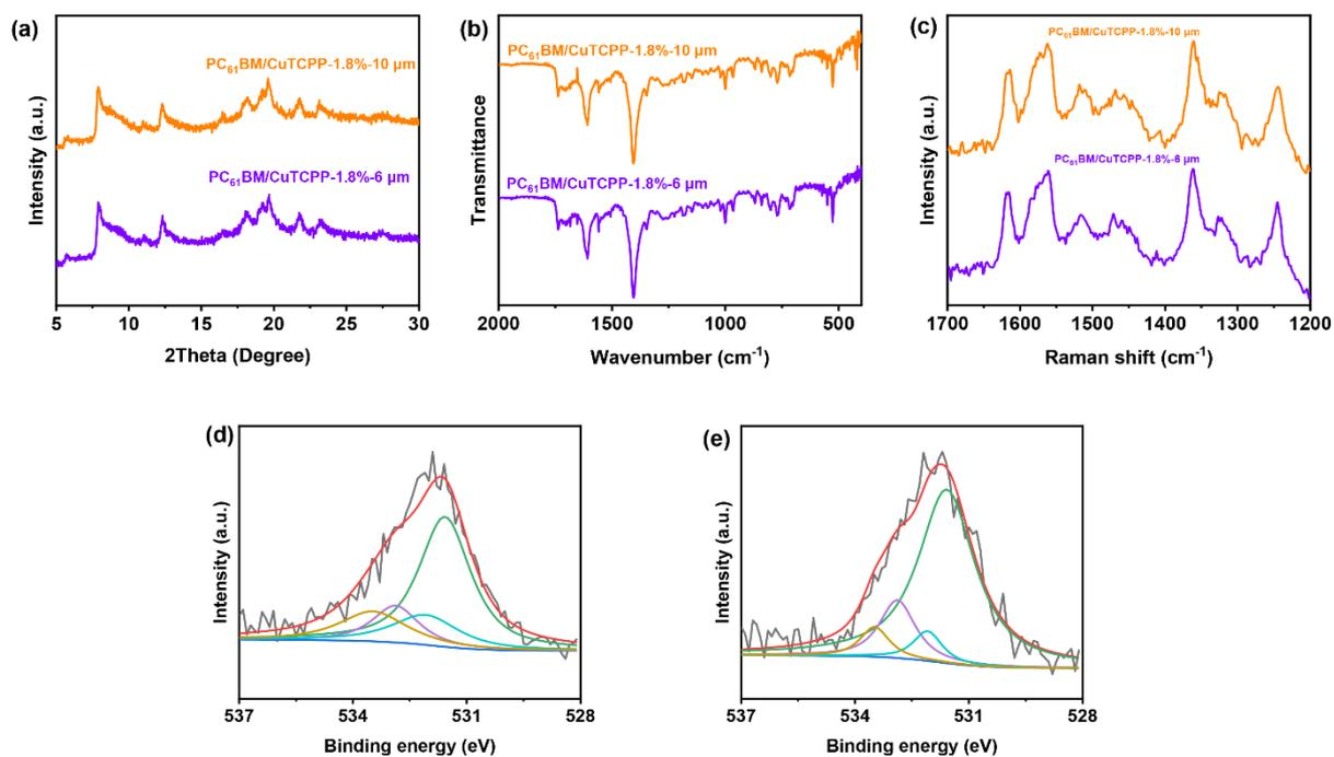
Figure S16. (a) Powder XRD patterns, (b) FTIR spectra, and Raman spectra of PC<sub>61</sub>BM/CuTCPP-1.8%-6 μm and PC<sub>61</sub>BM/CuTCPP-1.8%-11 μm. XPS O1s spectra of (d) PC<sub>61</sub>BM/CuTCPP-1.8%-6 μm and (e) PC<sub>61</sub>BM/CuTCPP-1.8%-11 μm.
