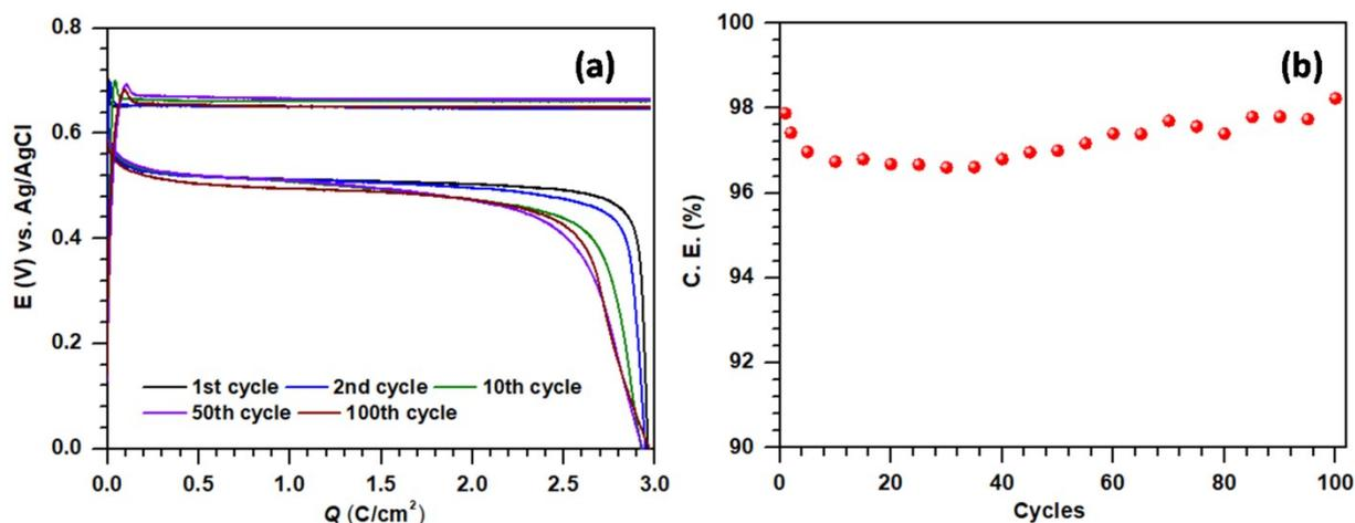
Fig. S9 (a) GCD cycles (shown for 5 specific cycles over 100) and (b) corresponding C.E. obtained during cycling on free-standing CNFs at  $Q_{\text{charge}}$  of 3 C/cm<sup>2</sup> in 1 M acetate buffer containing 0.1 M MnCl<sub>2</sub> (pH = 5).
