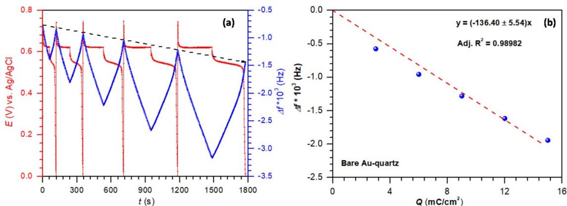
Fig. S7 (a) Galvanostatic (50  $\mu$ A/cm<sup>2</sup>) charge-discharge curves with different loads ( $Q_{\text{charge}}$ ) of 3, 6, 9, 12, and 15 mC/cm<sup>2</sup> applied successively on the same electrode and the simultaneous QCM trace for the bare Au-quartz electrode. (b) Corresponding  $\Delta f$  vs.  $Q_{\text{charge}}$  response.
