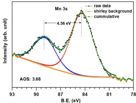
Fig. S4 Core-level Mn 3s XPS spectra of free-standing CNFs after electrodeposition of MnO<sub>2</sub> for  $Q_{\text{charge}}$  of 180 mC/cm<sup>2</sup> (charged state). The binding energy (B.E.) of Au 4f doublet exactly overlaps with that of Mn 3s doublet. Therefore, we performed XPS on the MnO<sub>2</sub> covered free-standing CNF electrodes after the first charge.
