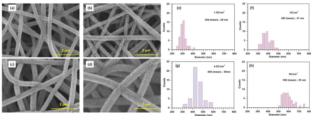
Fig. S8 (a-d) FEG-SEM images of free-standing CNFs after electrodeposition of  $\text{MnO}_2$  at  $1 \text{ mA}/\text{cm}^2$  for  $Q_{\text{charge}}$  of 1.5, 3, 4.5, and 6  $\text{C}/\text{cm}^2$ , respectively. (e-h) Distribution and mean diameter size of CNFs after electrodeposition of  $\text{MnO}_2$  at  $1 \text{ mA}/\text{cm}^2$  for  $Q_{\text{charge}}$  of 1.5, 3, 4.5, and 6  $\text{C}/\text{cm}^2$ , respectively.
