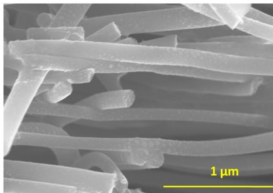
Fig. S3 Cross-section FEG-SEM image of CNF-covered Au-quartz electrode after electrodisolution of  $\text{MnO}_2$  for  $Q_{\text{charge}}$  of 180  $\text{mC}/\text{cm}^2$  (discharged state).
