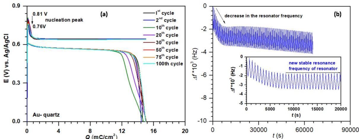
Fig. S6 (a) GCD cycles (shown for eight specific cycles) and (b) simultaneous QCM monitoring (frequency change) for electrodeposition-electrodissolution of MnO<sub>2</sub> on the bare Au-quartz electrode at 50  $\mu$ A/cm<sup>2</sup> for a total load ( $Q_{\text{charge}}$ ) of 15 mC/cm<sup>2</sup>. The inset in (b) shows the frequency change for the initial few cycles.
