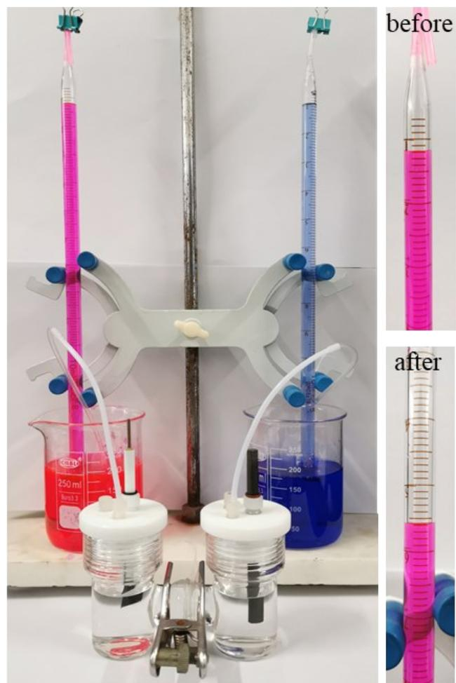
Figure S17. Faradic efficiency test device.
