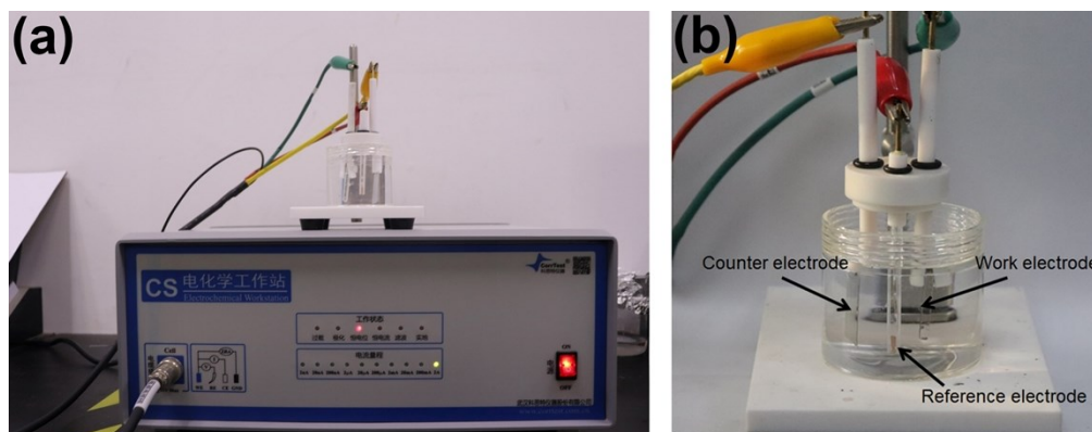
Figure S1. Digital photographs of the CS380 electrochemical workstation (a) and the three-electrode cell (b).
