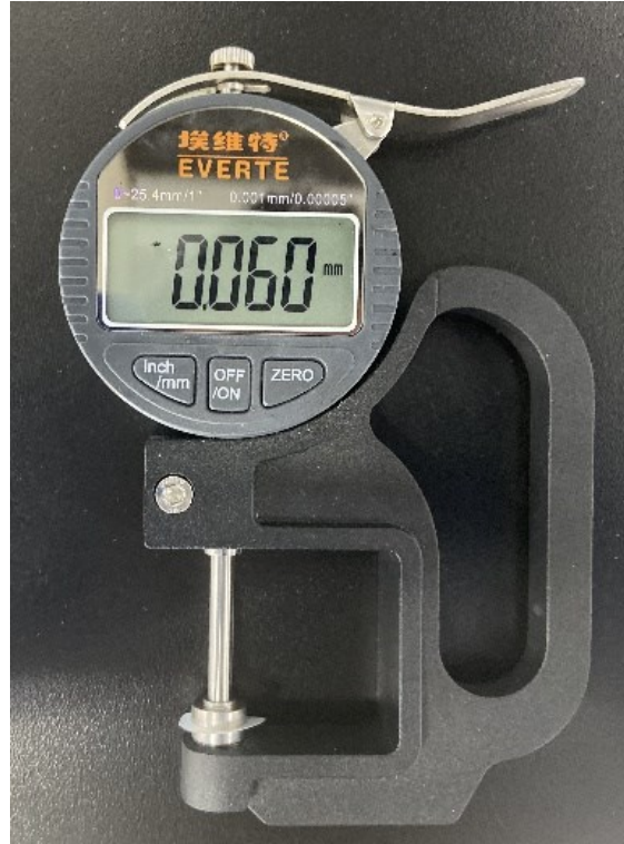
Fig. S2 Thickness of the porous P-PLC-IL SPE (60 \mu\text{m} ).
