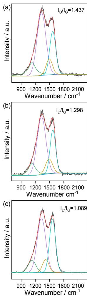
Figure S4. Raman spectra of MT-600 (a), MT-800 (b) and MT-1000 (c).
