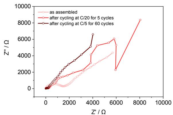
Figure S12. Nyquist plot of a cell that underwent long term cycling.
