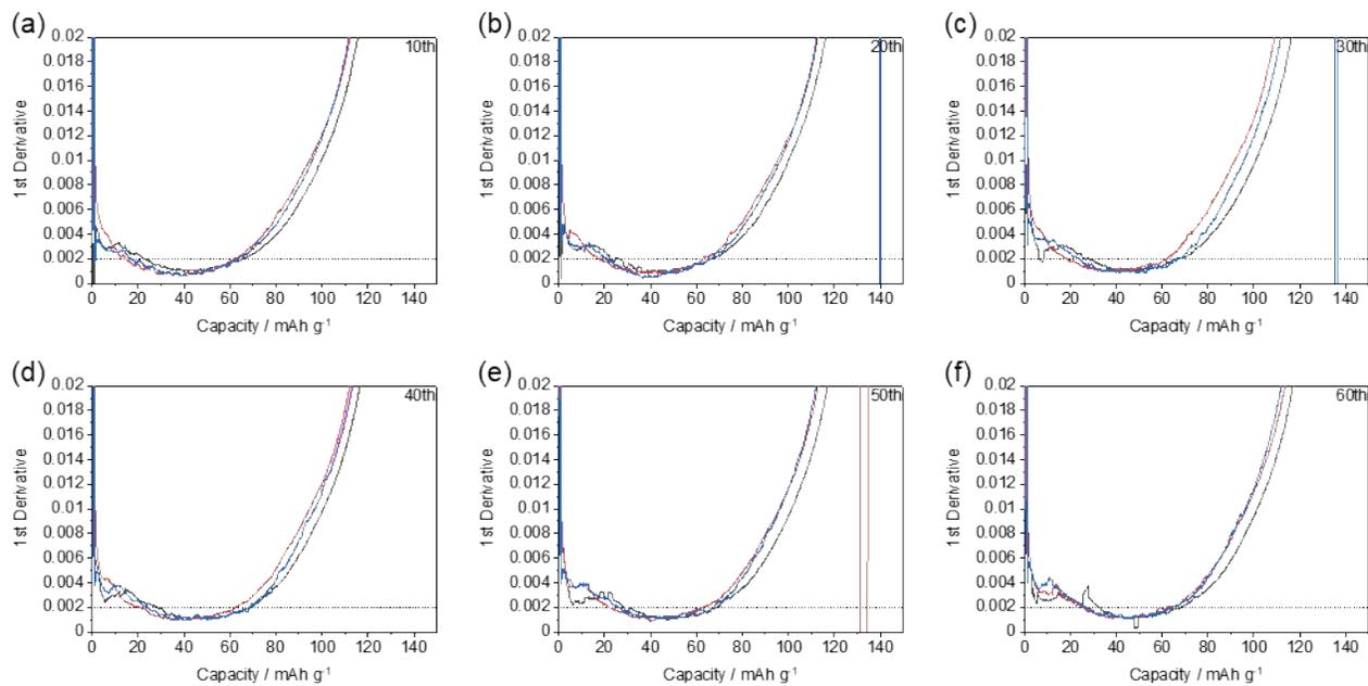
Figure S11. First derivation of desodiation curves of MT-1000 cycled for 60 cycles at current density  $C/5$  with sodiation limit of  $139 \text{ mAh g}^{-1}$  and desodiation limit of  $2.5 \text{ V}$ . Dotted line signifies the end of the plateau. (a) 10<sup>th</sup>, (b) 20<sup>th</sup>, (c) 30<sup>th</sup>, (d) 40<sup>th</sup>, (e) 50<sup>th</sup>, and (f) 60<sup>th</sup> cycle are shown.
