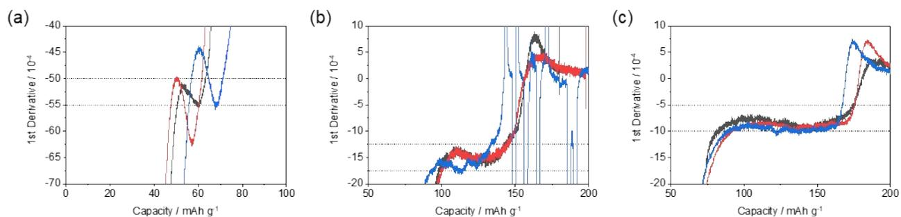
Figure S7. First derivation of dipped sodiation curves of (a) MT-600, (b) MT-800, and (c) MT-1000 at current density  $C/20$ . Lower dotted line signifies the beginning of the plateau while the upper one signifies the end of the plateau and the beginning of sodium plating.
