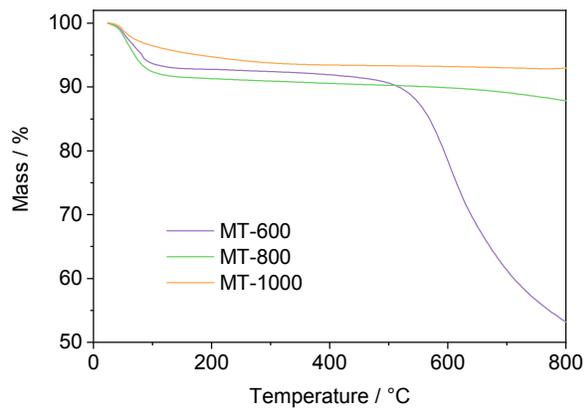
Figure S2. Thermogravimetric analysis (TGA) of MT-600, MT-800 and MT-1000 under nitrogen atmosphere.
