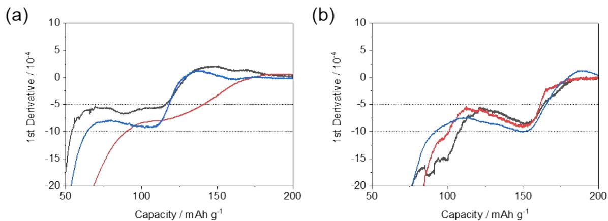
Figure S10. First derivation of dipped sodiation curves of MT-1000 at current densities  $C/2$  (a) and  $C/5$  (b). Lower dotted line signifies the beginning of the plateau while the upper one signifies the end of the plateau and the beginning of sodium plating.
