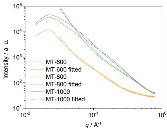
Figure S5. SAXS curves fitted to the pore-matrix approximation.
