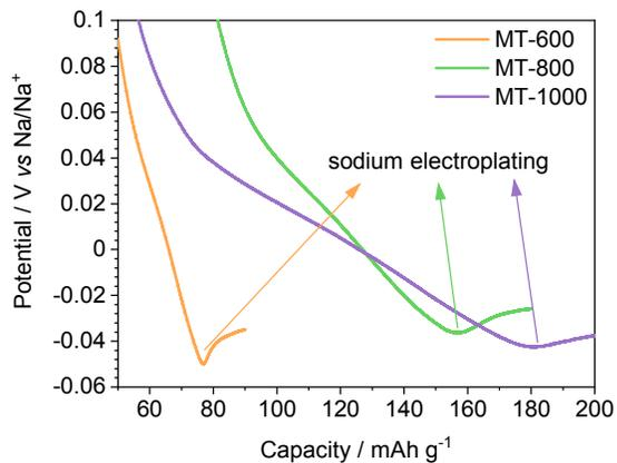
Figure S8. Magnification of electroplating presented in Figure 4d.
