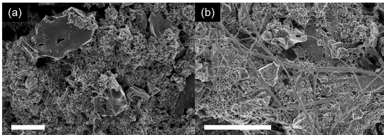
Figure S13. MT-1000 incorporated in the electrode (a) before any electrochemical experiments and (b) after 5 cycles at current density C/20 followed by 60 cycles at current density C/5. The bar represents 20  $\mu\text{m}$ .
