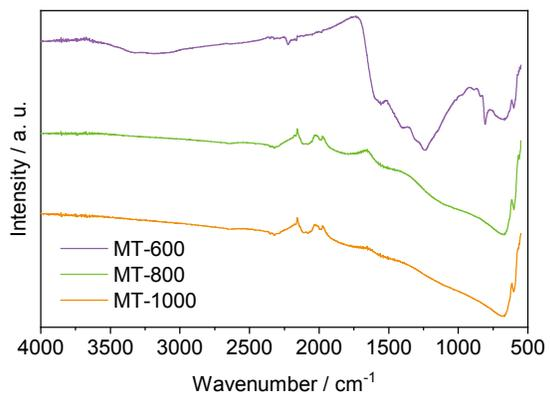
Figure S3. Infrared spectra of MT-600, MT-800 and MT-1000.
