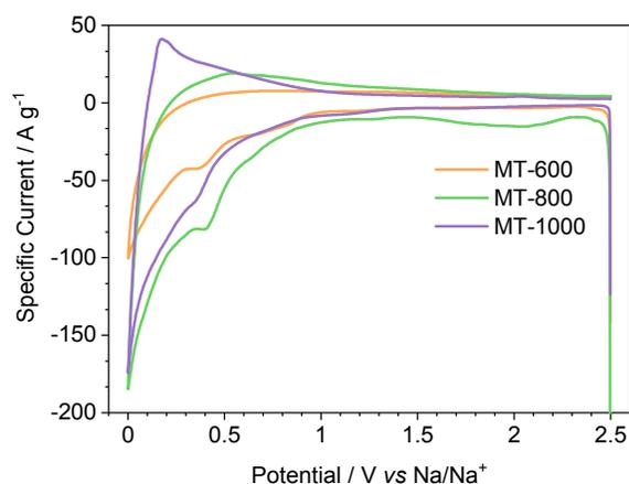
Figure S6. First cycle of cyclic voltammetry of MT-600, MT-800 and MT-1000 at the scan rate of  $0.1 \text{ mV s}^{-1}$ .
