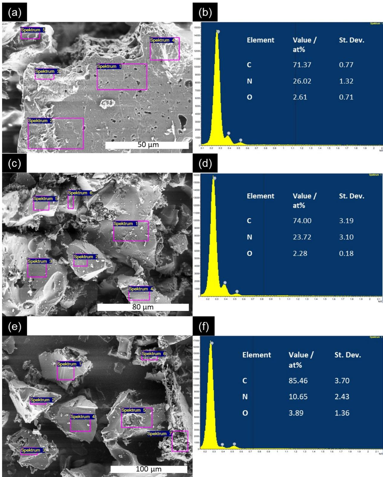
Figure S1. Energy-dispersive X-ray spectroscopy (EDX) analysis of (a,b) MT-600, (c,d) MT-800, and (e,f) MT-1000. Image of (a,c,e) the analysed samples and (b,d,f) corresponding spectra are shown.
