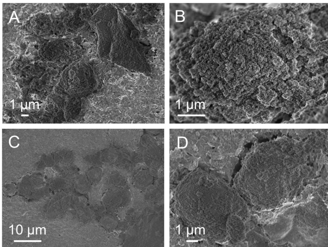
**Figure S18** SEM images of samples collected after hydrothermal synthesis for 6h (A, B) and 8h (C, D).
