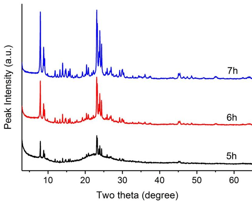
**Figure S16** XRD patterns of the sample obtained after hydrothermal synthesis at 443 K for 5 h, 6h and 7h.
