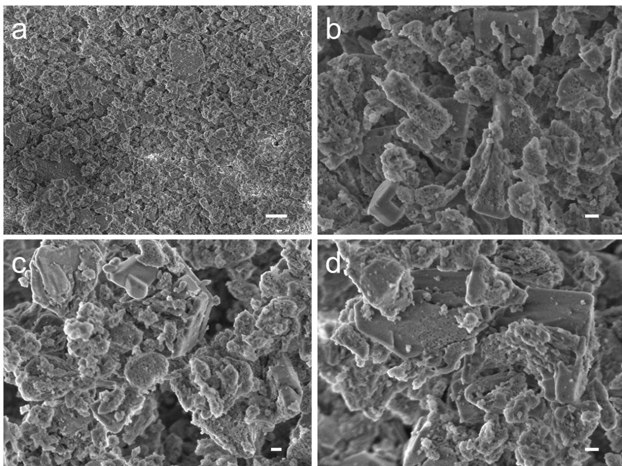
**Figure S21** SEM images at different magnifications showing the defect-zoning of the calcined ZSM-5-H1 zeolite after  $\text{NH}_4\text{F}$  treatment. Scale bars are 100 nm in b-d and 1  $\mu\text{m}$  in a.
