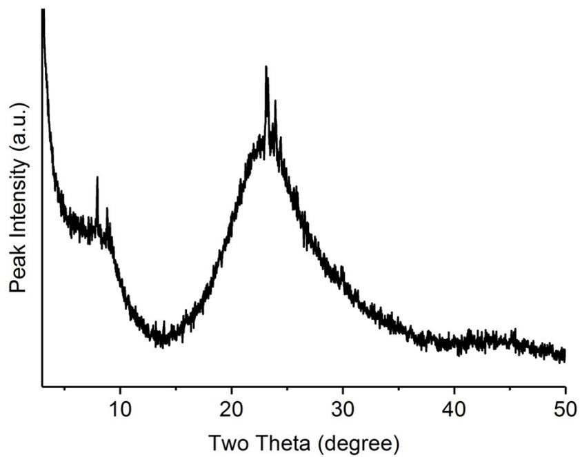
**Figure S15** XRD pattern of the sample obtained after hydrothermal synthesis at 443 K for 4 h.
