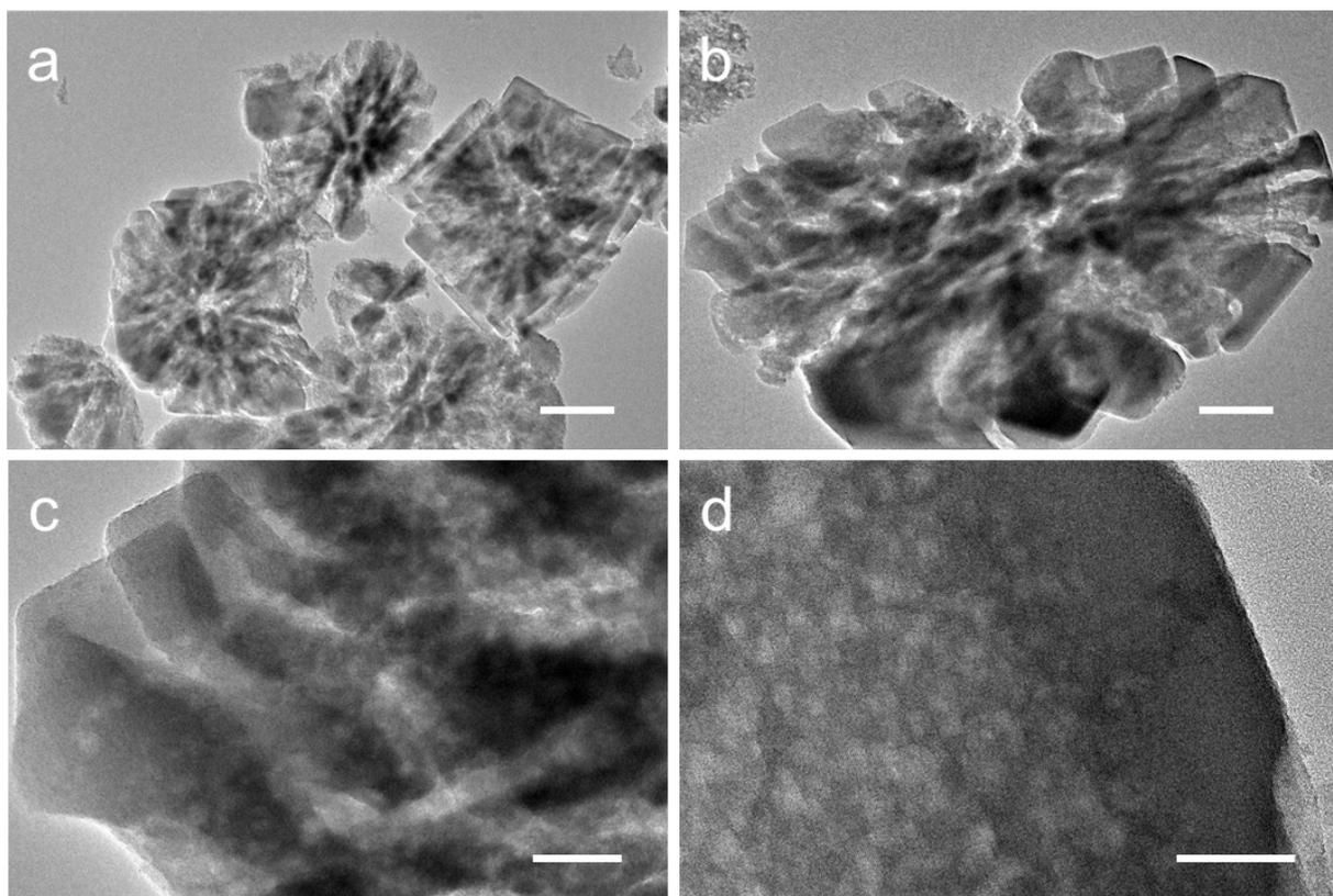
**Figure S22** TEM images at different magnifications showing the defect-zoning of the calcined ZSM-5-H1 zeolite after  $\text{NH}_4\text{F}$  treatment. Scale bars are 500 nm in a, 200 nm in b and 50 nm in c and d.
