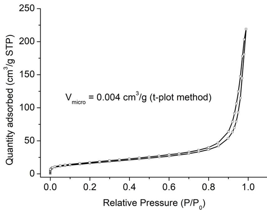
**Figure S10** N<sub>2</sub> (77K) physisorption isotherms of Na<sup>+</sup> exchanged TPA-Z<sub>F</sub> zeolite.
