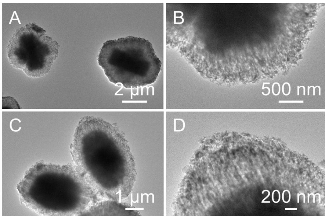
**Figure S4** TEM images showing the either rectangular (A) or elliptical shaped (C) core part (“egg-yolk”) of sample TPA-Z<sub>F</sub>. Figures S4B and S4D highlight the very porous nature of the outer layer (“egg-white”) and the much less porous nature of the core part.
