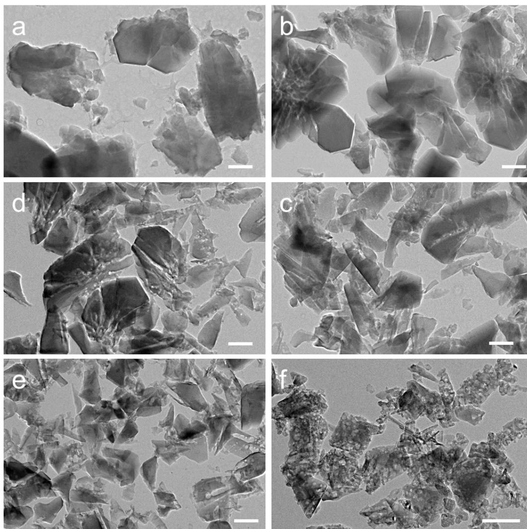
**Figure S20** TEM images of the parent ZSM-5-I from Grace Davison (a), and the samples treated by  $\text{NH}_4\text{F}$  for different time (b: 5 min; c: 10 min; d: 20 min; e: 40 min; f: 60 min), scale bars in a-f are 200 nm. The experimental conditions for the  $\text{NH}_4\text{F}$  etching of  $\text{Z}_p$  are identical with the fluoride etching of the ZSM-5 sample from Grace Davison.
