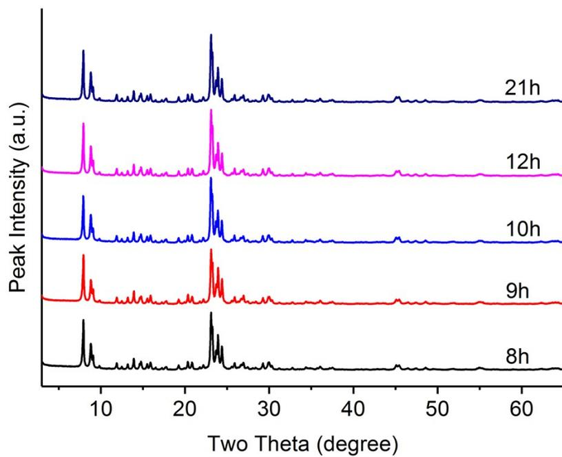
**Figure S17** XRD patterns of zeolites obtained after different times of hydrothermal synthesis.
