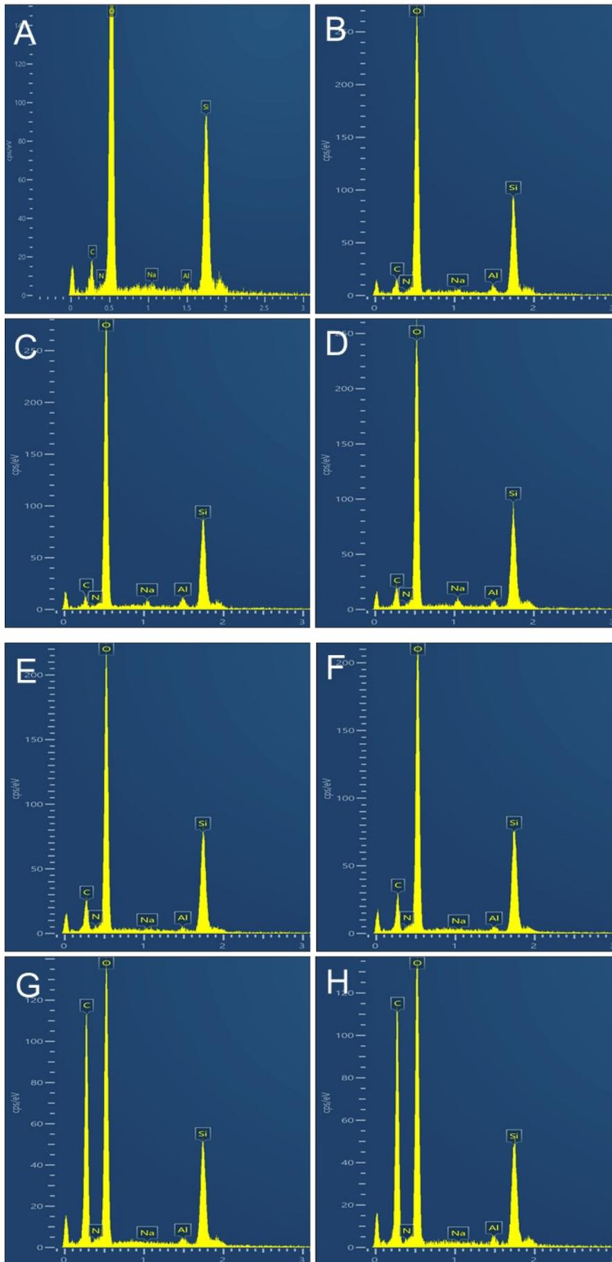
**Figure S5** SEM-EDX spectra showing the point analysis results for zones 1 (A), 2 (B), 3 (C) and 4 (D) indicated in Figure 4A; zones 1 (E), 2 (F), 3 (G) and 4 (H) indicated in Figure 4C.
