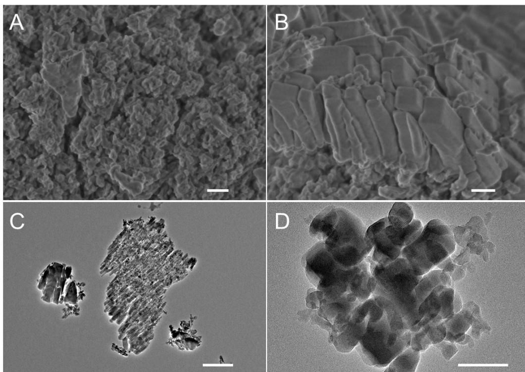
**Figure S9** SEM (A, B) and TEM (C, D) images showing the surface details of the  $R_2$  (A) and  $R_1$  (B-D) zones of sample TPA- $Z_F$ . Scale bar: 100 nm in A, B and D; 500 nm in C.
