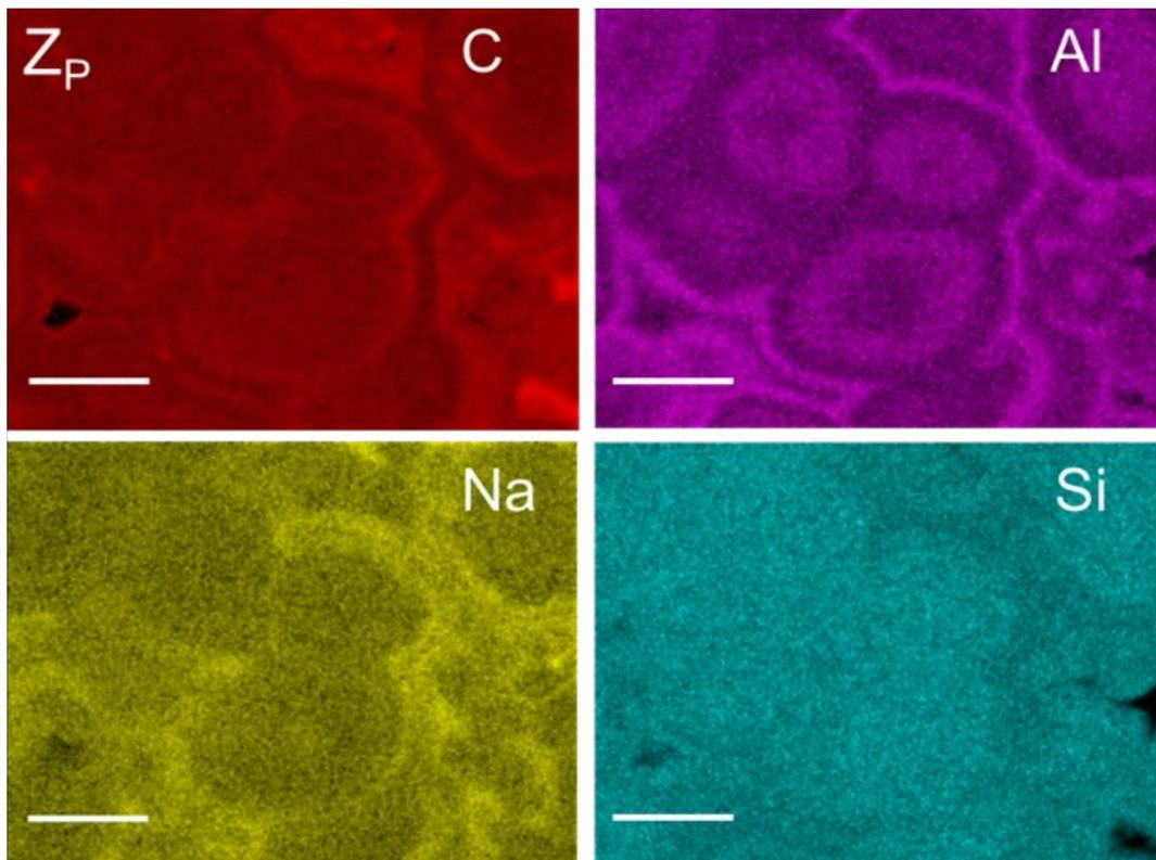
**Figure S6** SEM EDX mappings of the Z<sub>p</sub> (parent ZSM-5) zeolite crystals. Scale bar = 2.5 μm.
