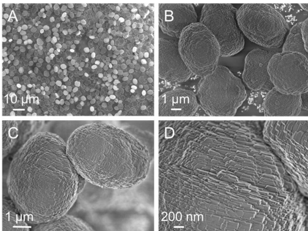
**Figure S1.** SEM images of Z<sub>p</sub> (parent ZSM-5 zeolite).
