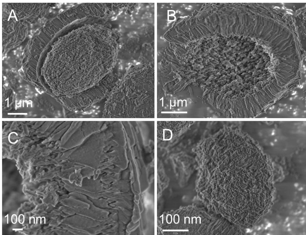
**Figure S3** SEM images of sample TPA-Z<sub>F</sub> showing the core-shell structure (A), the empty shell (B), the structural details of the shell (C) and the naked core part (D).
