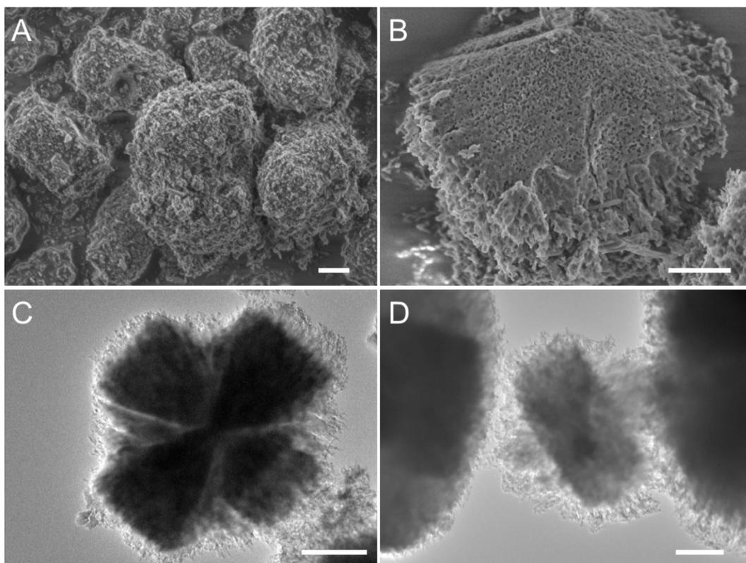
**Figure S8** SEM (A, B) and TEM (C, D) images of calcined ZSM-5 samples (no TPA<sup>+</sup>) treated by NH<sub>4</sub>F. (A, C, D) The sample was collected after 1 h treatment with NH<sub>4</sub>F. (B) The sample was collected after 2 h treatment with NH<sub>4</sub>F. Scale bar: 1 μm in A and C; 500 nm in B and D.
