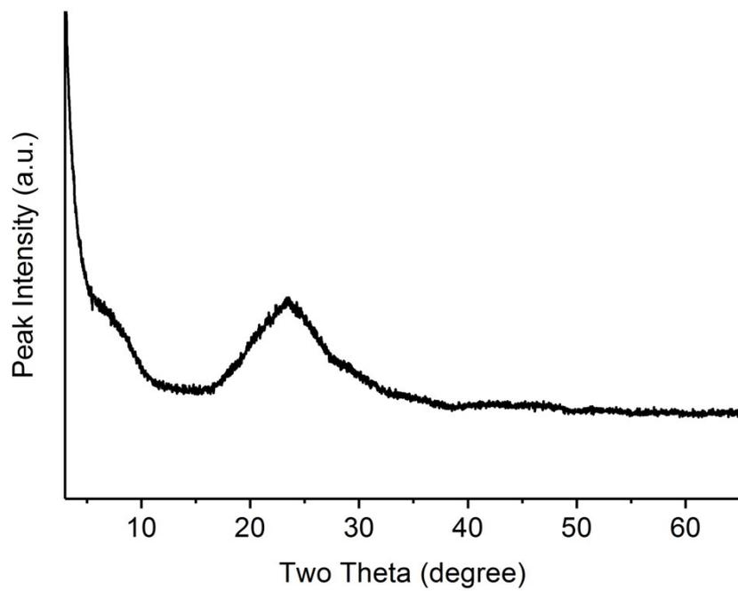
**Figure S12** XRD pattern of the sample collected after hydrothermal synthesis at 443 K for 2 h.
