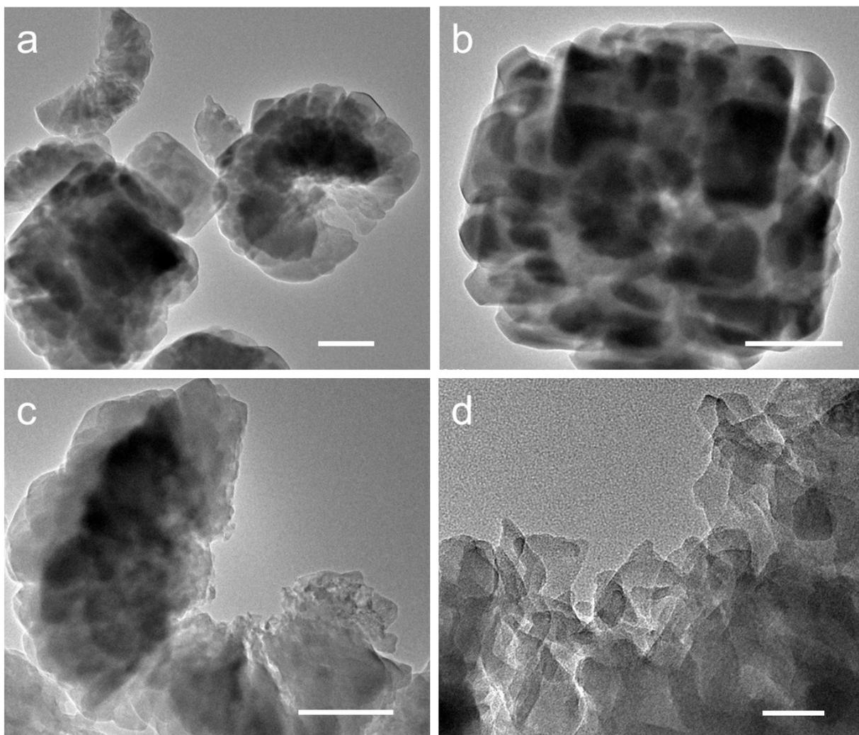
**Figure S24** TEM images of the as-synthesized ZSM-5-H1 zeolite after  $\text{NH}_4\text{F}$  treatment (a-d). Scale bars are 500 nm in a-c, and 50 nm in d.
