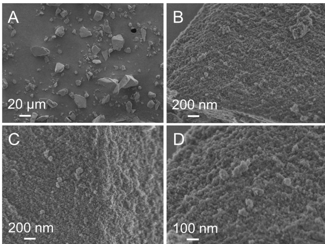
**Figure S13** SEM images of samples obtained after hydrothermal synthesis at 443 K for 2 h.
