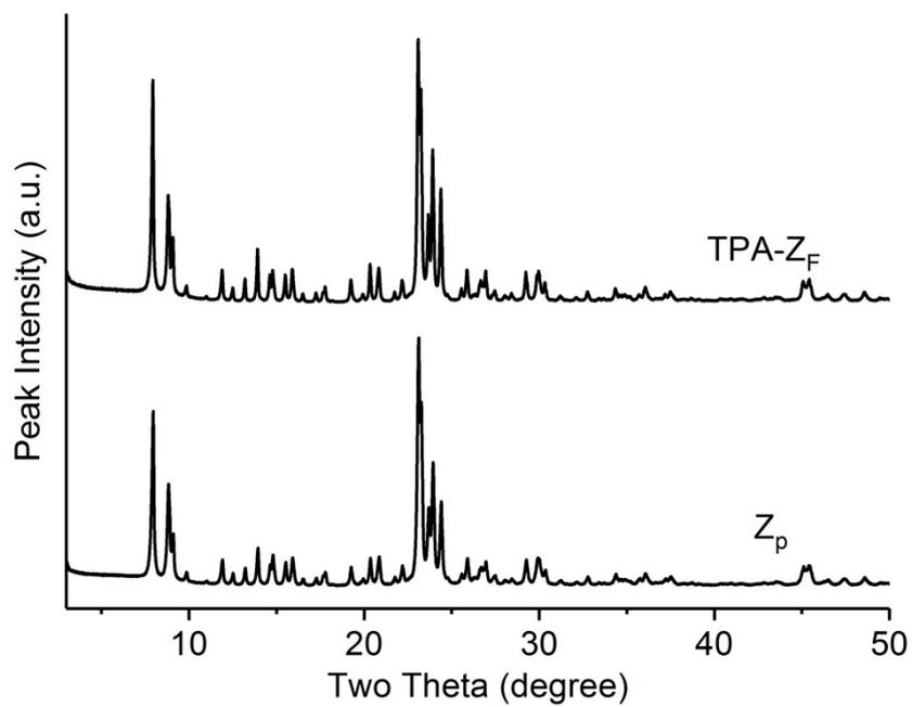
**Figure S2** XRD patterns of the Z<sub>p</sub> (parent) and TPA-Z<sub>F</sub> (NH<sub>4</sub>F treated) ZSM-5 zeolite samples.
