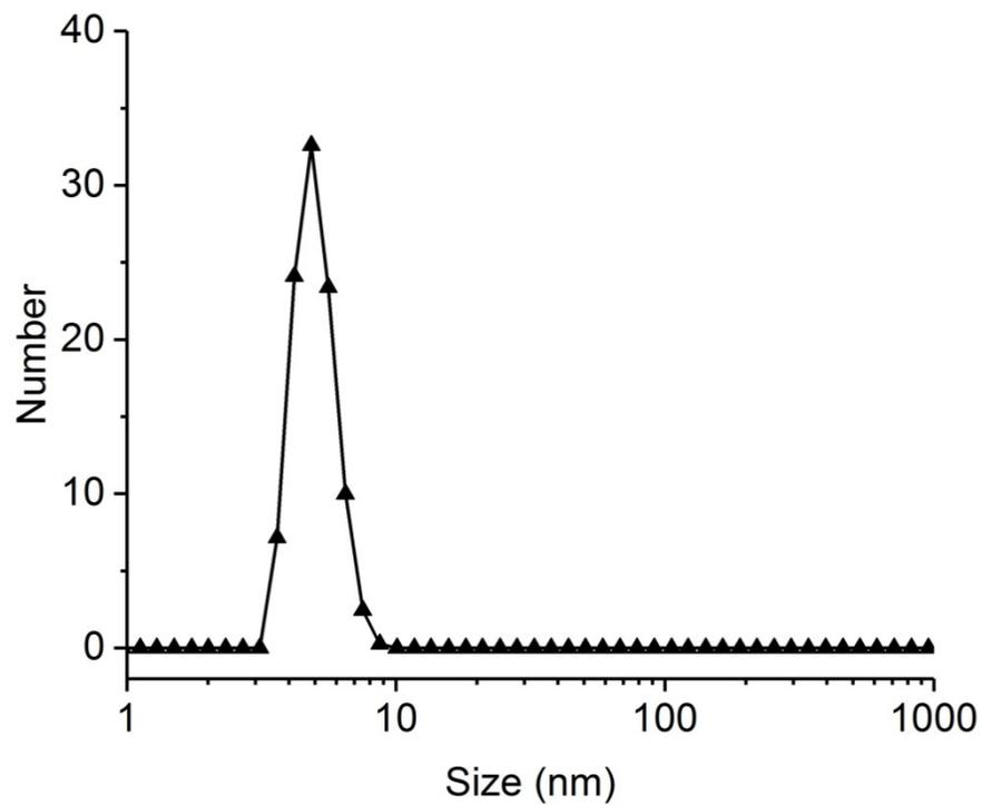
**Figure S11** Particles size distribution of the aluminosilicate precursor gel determined by dynamic light scattering (DLS).
