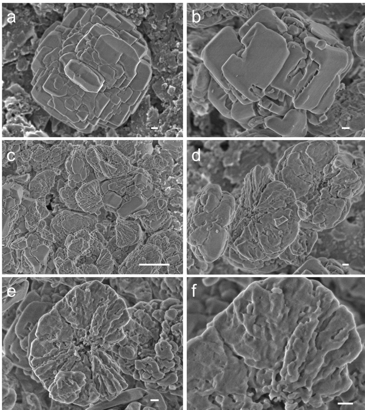
**Figure S23** SEM images of the as-synthesized ZSM-5-H1 zeolite (a) and the  $\text{NH}_4\text{F}$  treated counterparts (b-f) showing the preferential dissolution of zeolite core and the splitting of crystals along extended grain boundaries. The durability of zeolite crystals in  $\text{NH}_4\text{F}$  solution is due to the protection effect of charge and defect sites compensating  $\text{TPA}^+$ . Scale bars are all 100 nm except 1  $\mu\text{m}$  in c.
