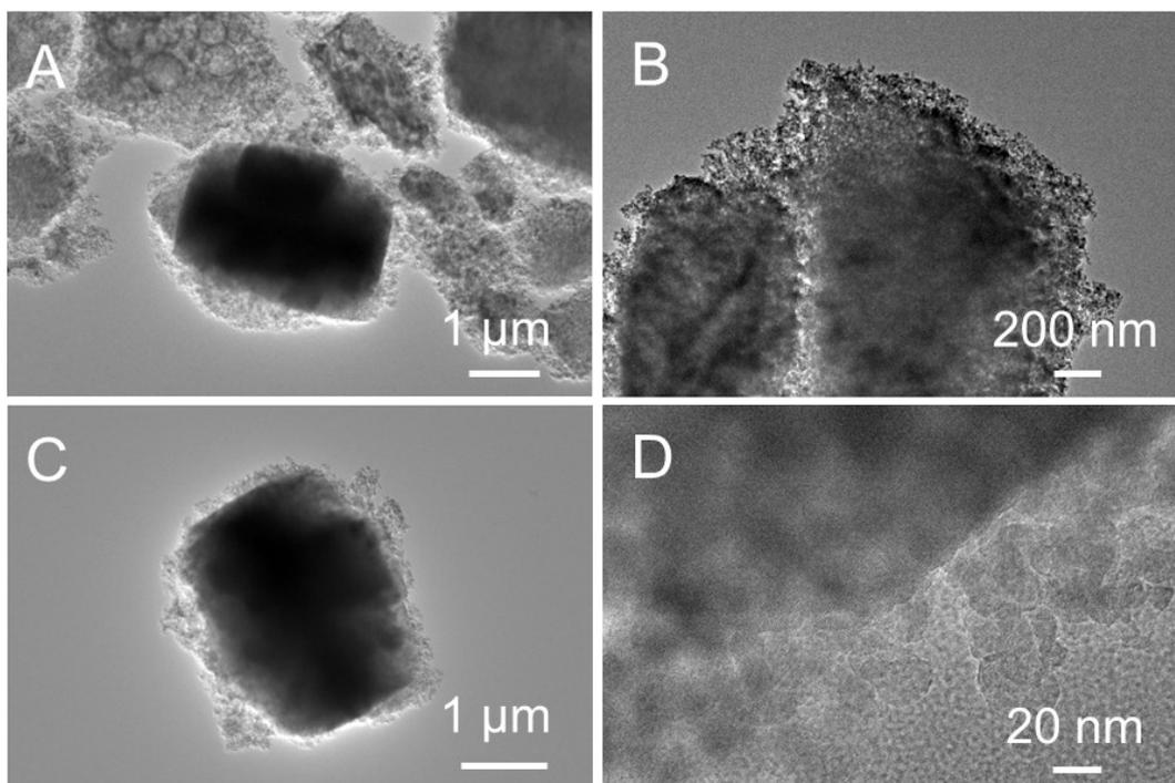
**Figure S14** TEM images of sample obtained after hydrothermal synthesis at 443 K for 4 h.
