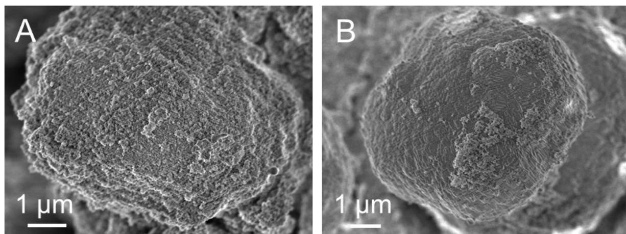
**Figure S19** SEM images showing the morphology change of zeolite particles after hydrothermal synthesis of (A) 9 h and (B) 12 h.
