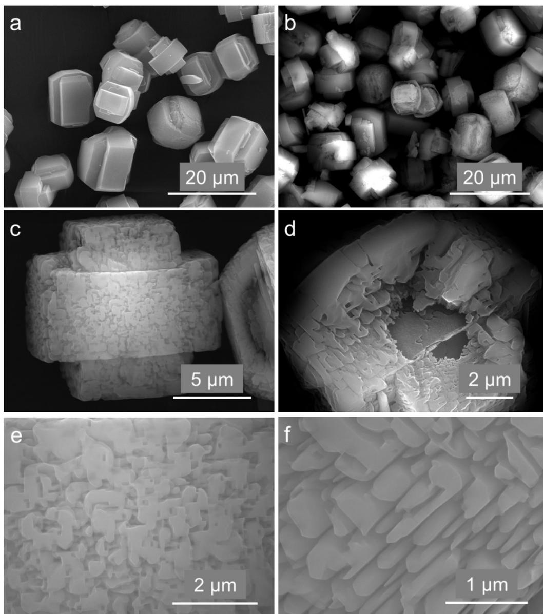
**Figure S25** SEM images of parent (a) and NH<sub>4</sub>F treated (b-f) ZSM-5-H2 zeolite at different magnifications showing the dissolution behavior of ZSM-5-H2 under the protection of TPA<sup>+</sup>.
