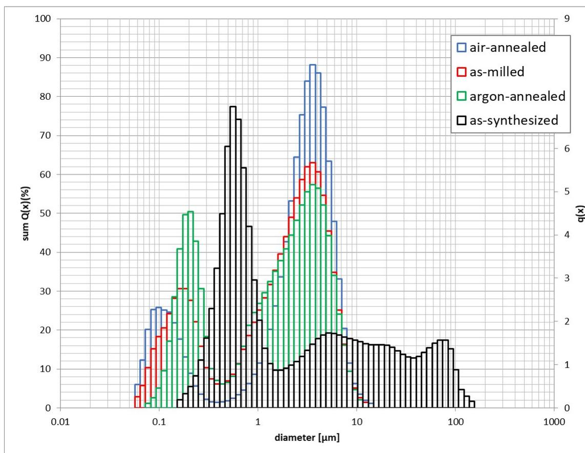
Supp 1 Particle size distribution of the LLZO powders before milling, after milling and after annealing
