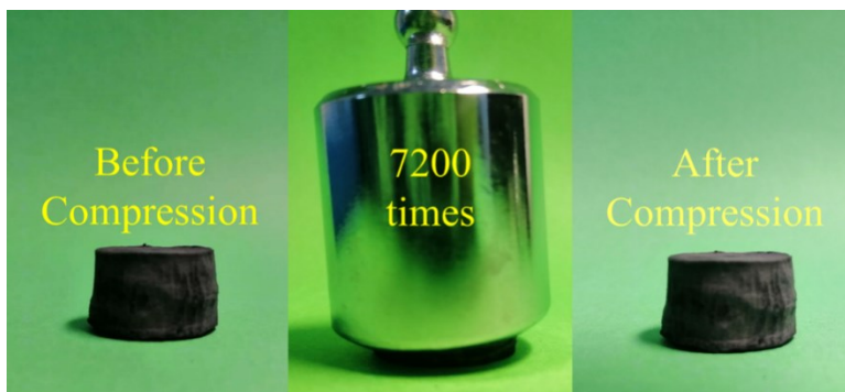
Fig. S9 Digital photos showing the state of the prepared C/rGO-10 aerogel upon a heavy weight.
