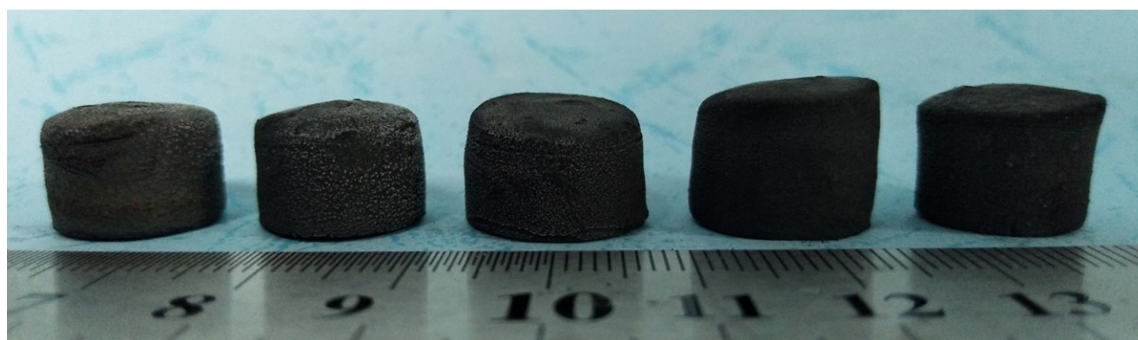
Fig. S6 Digital images of (a) BC/GO and (b) C/rGO aerogels with different GO loading (0%, 5%, 10%, 15%, 20%).
