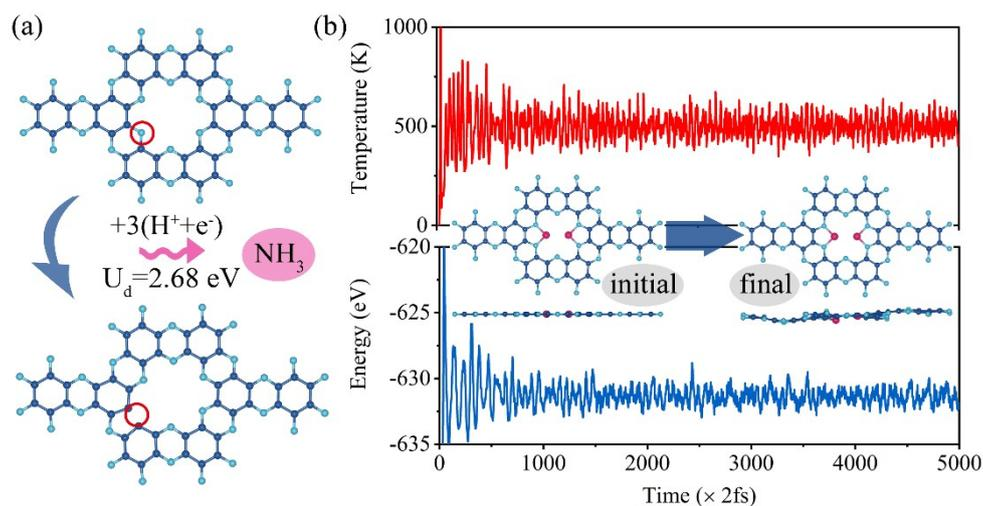
**Figure S9.** (a) Decomposition mechanism of C<sub>2</sub>N substrate. (b) Variations of temperature and energy against the time for AIMD simulations of 2P@C<sub>2</sub>N, insert are top and side views of the snapshot of initial and final structures. The simulation is run under 500 K for 10 ps with a time step of 2 fs.
