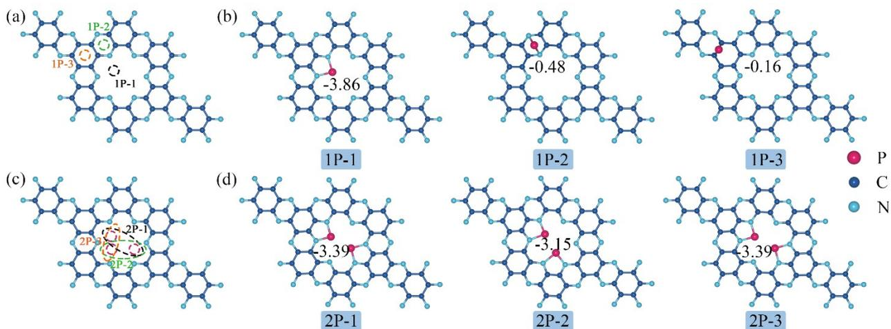
**Figure S1.** Possible doping sites of (a) single and (c) double P atoms on C<sub>2</sub>N. Optimized structures of (b) single and (d) double P atoms doped C<sub>2</sub>N, the corresponding adsorption energies are included.
