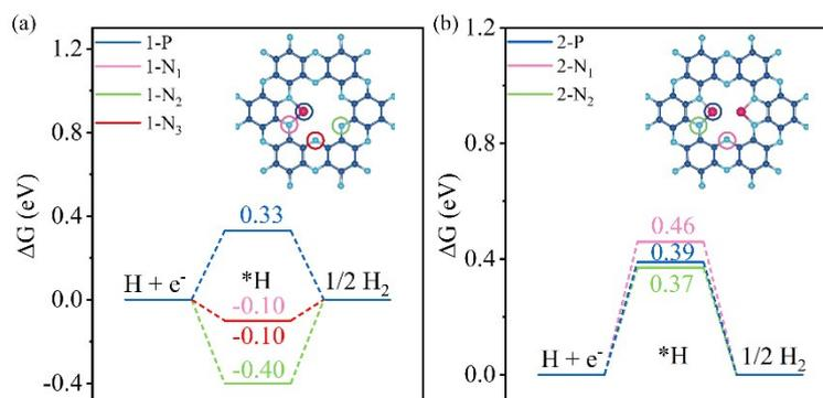
**Figure S7.** Gibbs free energy diagrams for HER on possible adsorption sites of (a)  $1P@C_2N$  and (b)  $2P@C_2N$ . Inserts illustrate the possible adsorption sites of H atom on  $1P@C_2N$  and  $2P@C_2N$ .
