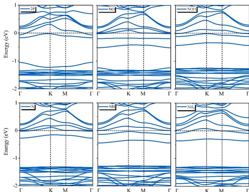
**Figure S5.** Band structures of intermediates for NORR on 2P@C<sub>2</sub>N through O-distal pathway.
