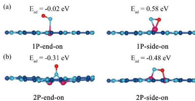
**Figure S2.** Crystal structures of NO adsorbed (a) 1P@C<sub>2</sub>N and (b) 2P@C<sub>2</sub>N with end-on and side-on configurations, the corresponding adsorption energies ( $E_{ad}$ ) are included.
