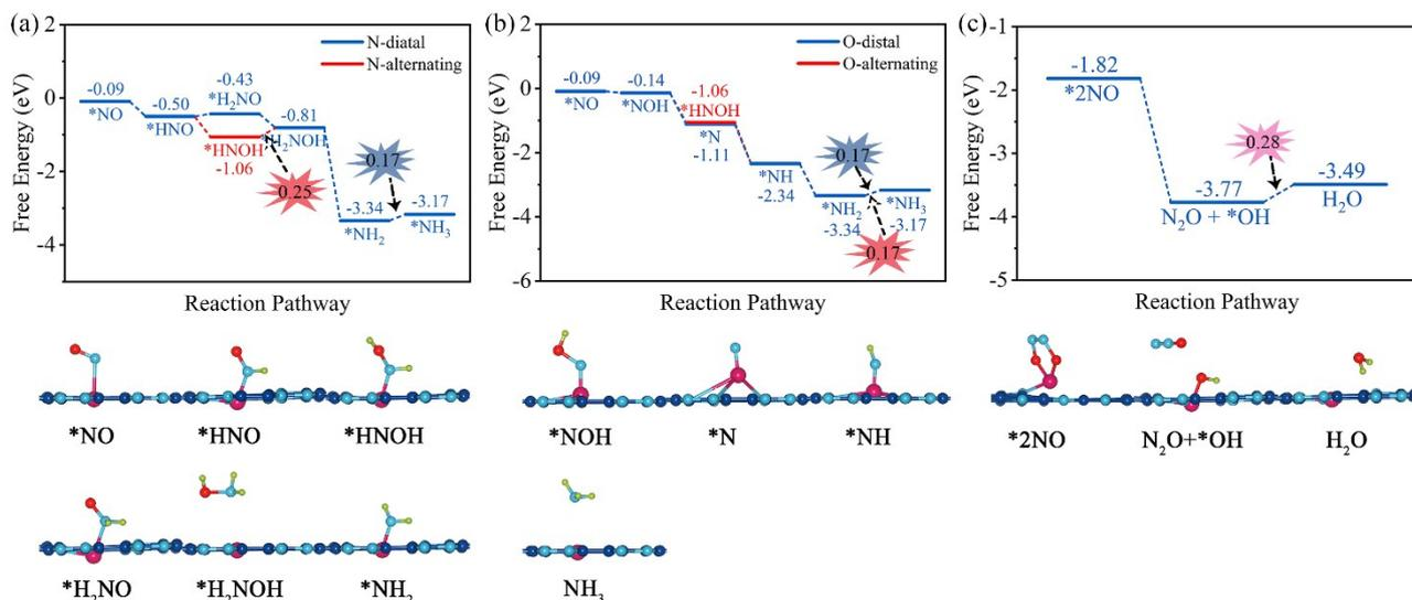
**Figure S3.** Optimized intermediates and calculated Gibbs free energy diagrams of NORR for NH<sub>3</sub> synthesis through (a) N-distal/alternating and (b) O-distal/alternating reaction pathways on 2P@C<sub>2</sub>N at U = 0 V. (c) Optimized intermediates and calculated Gibbs free energy diagrams of NORR for N<sub>2</sub>O synthesis on 2P@C<sub>2</sub>N at U = 0 V.
