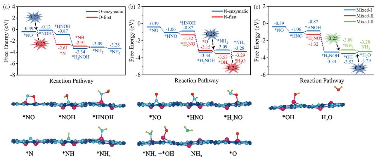
**Figure S4.** Optimized intermediates and calculated Gibbs free energy diagrams of NORR for NH<sub>3</sub> synthesis through (a) O-first/enzymatic, (b) N-first/enzymatic and (c) Mixed-I/II/III reaction pathways on 2P@C<sub>2</sub>N at U = 0 V.
