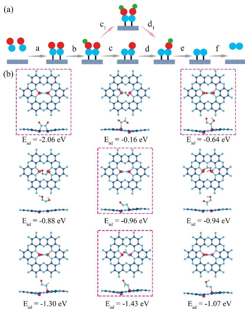
**Figure S6.** (a) Schematic illustration of the possible reaction pathways of NORR for  $N_2$  synthesis. (b) Possible configurations and the corresponding adsorption energies for the intermediates. The dotted box marks the most stable adsorption configuration in each reaction step.
