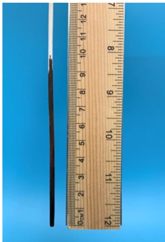
Figure S16. The final height of fluid transport along the delignified reed.
