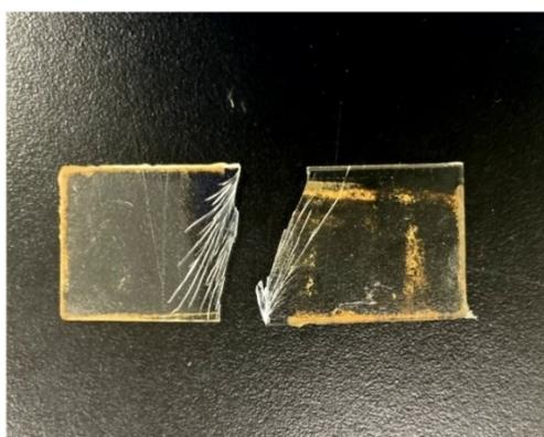
**Figure S8.** Digital image of a fragile CE without PA.
