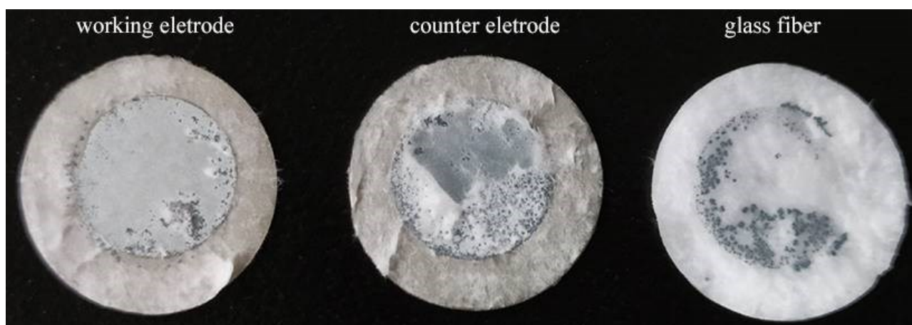
Figure S2. Digital photos of the working electrode, the counter electrode, and the separator (Post-mortem cell after short-circuit)
