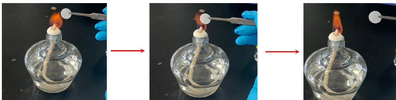
Figure S4. Photographs of the ignition tests of the glass fibers saturated with glycerol/water (50/50) hybrid electrolyte.
