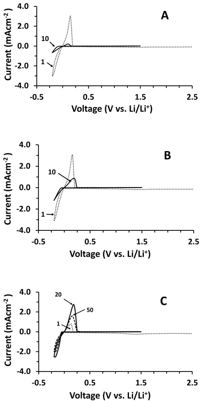
**Fig. S2.** Cyclic voltammograms for Li plating/stripping on SS in 0.25 M  $\text{LiBF}_4/\text{ADN}$  with  $\text{Li}/\text{Li}_2\text{O}$  treated in (A) 0.5, (B) 1.0, and (C) 2.0 wt%  $\text{NO}_2\text{BF}_4$ . Scan rate = 0.2  $\text{mVs}^{-1}$ . Coin cell ( $\text{Li}/\text{Li}_2\text{O} \parallel \text{SS}$ ).
