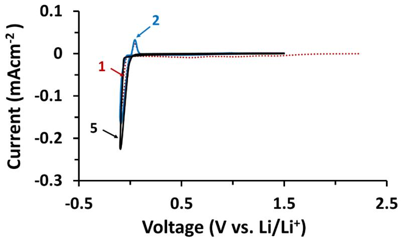
**Fig. S5.** Cyclic voltammograms for Li plating/stripping on SS coupled with Li/ $\text{Li}_2\text{O}$  in 1.0 M LiTFSI/ADN. Scan rate = 0.2 mVs<sup>-1</sup>. Coin cell (Li/ $\text{Li}_2\text{O}$  || SS).
