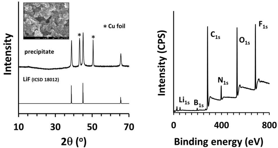
**Fig. S3.** (left) XRD pattern of precipitates produced during Li plating/stripping with bare Li (described in Fig. 3A). Inset shows a FESEM image of precipitates. The precipitates are composed of spherical particles of ca. 100 nm in diameter, which can block the separator in a coin cell set-up (Figure 1B). (right) XPS spectrum of precipitates.
