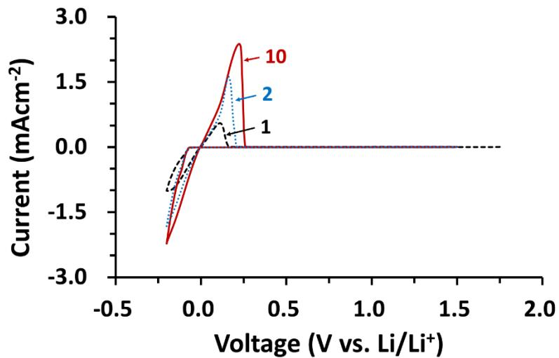
**Fig. S1.** Cyclic voltammograms for Li plating/stripping on SS in 0.25 M LiBF<sub>4</sub>/EC:DEC (ethylene carbonate : diethyl carbonate, 3:7). Scan rate = 0.2 mVs<sup>-1</sup>. Coin cell (Li || SS).
