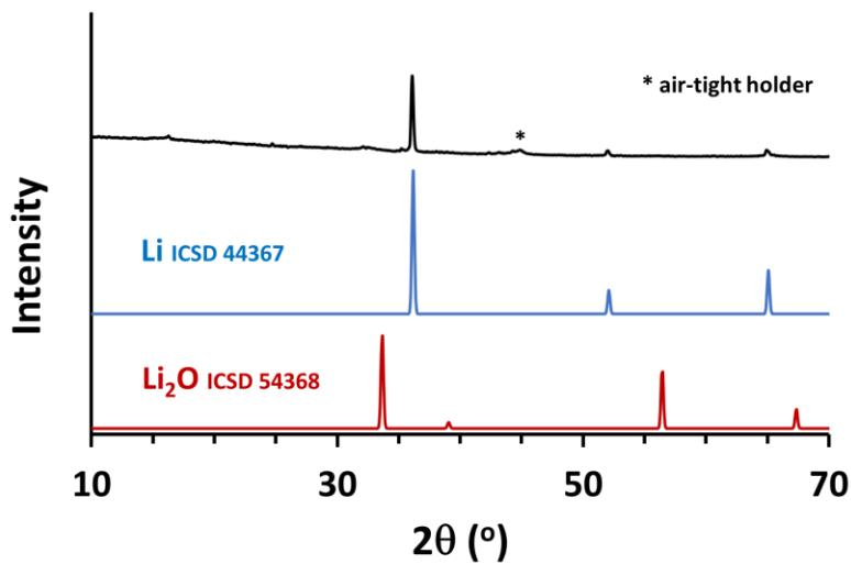
**Fig. S4.** XRD pattern of a powdery sample obtained from the surface film generated by immersing Li foil in  $\text{NO}_2\text{BF}_4$ /ADN. The surface film was gently rubbed with a soft rod to avoid the inclusion of a large quantity of underlying Li metal.
