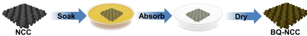
**Scheme S1.** Schematic illustrating the fabrication of BQ-NCC composite electrodes via a simply “solution-adsorption” process.
