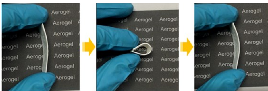
Figure S8. Photographs of a hand bending test on SP2, which demonstrate that SP2 shows high bending flexibility.
