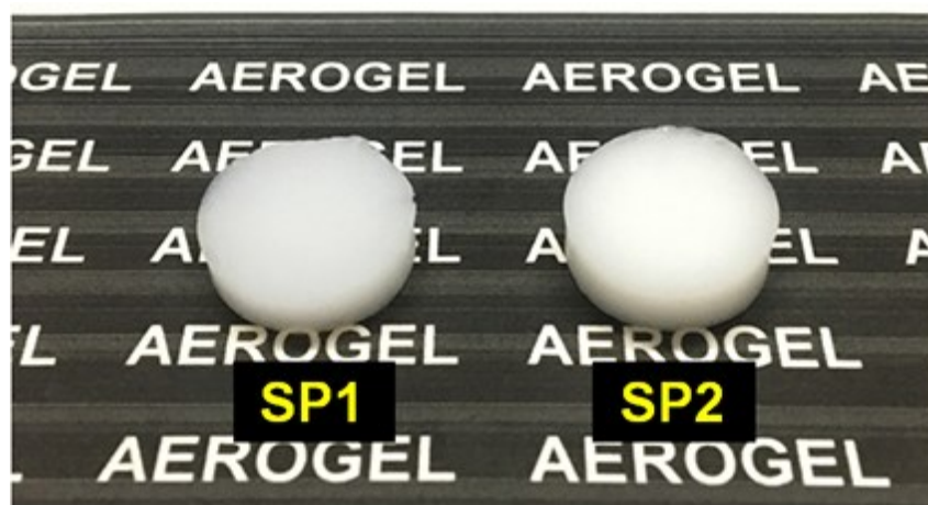
Figure S1. Photograph of starch/polyorganosiloxane biocomposite aerogels obtained via APD. It is shown that the samples SP1 and SP2 are monolithic and optically opaque.
