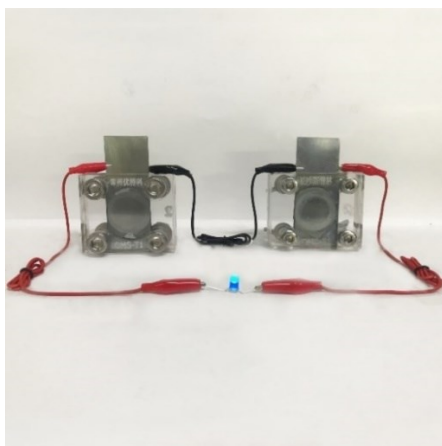
Fig. S10 Photograph of a blue LED ( \approx 3 V) lit by two series Zn-air batteries with MNSs@NGA as air cathode after 24 h.
