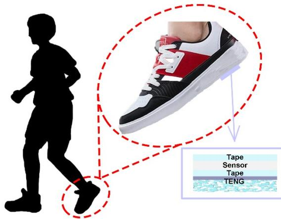
**Fig. S6** Schematic diagram for monitoring human gaits.
