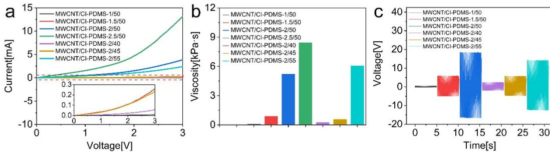
**Fig. S2** (a) The current to voltage (I-V) curves and (b) steady shear viscosities of a series of MWCNT/CI-PDMS composites with different MWCNT and CI contents. (c) The triboelectric output performance at 40.0 N of different MWCNT/CI-PDMS based TENGs.
