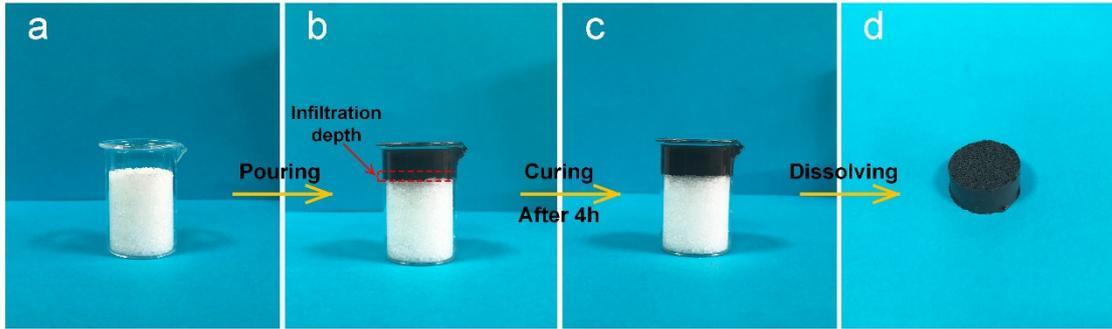
**Fig. S1** (a-d) Preparation process of the CI-Ecoflex-70 sponge, in which the high viscosity impeded its flowability.
