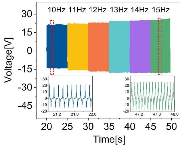
**Fig. S4** Real-time voltages of TENG subjected to varying frequency of 10-15 Hz.
