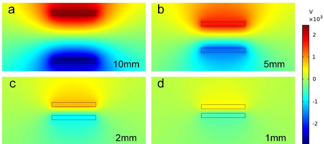
**Fig. S3** (a-d) Simulated electric potential distributions when an object was approaching the TENG.
