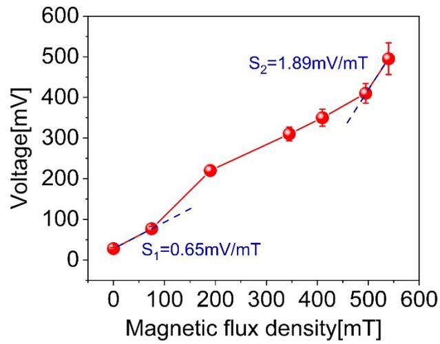
**Fig. S7** The calculated magnetic field monitoring sensitivity, which was defined as the increment of voltage caused by the change of unit magnetic flux density.
