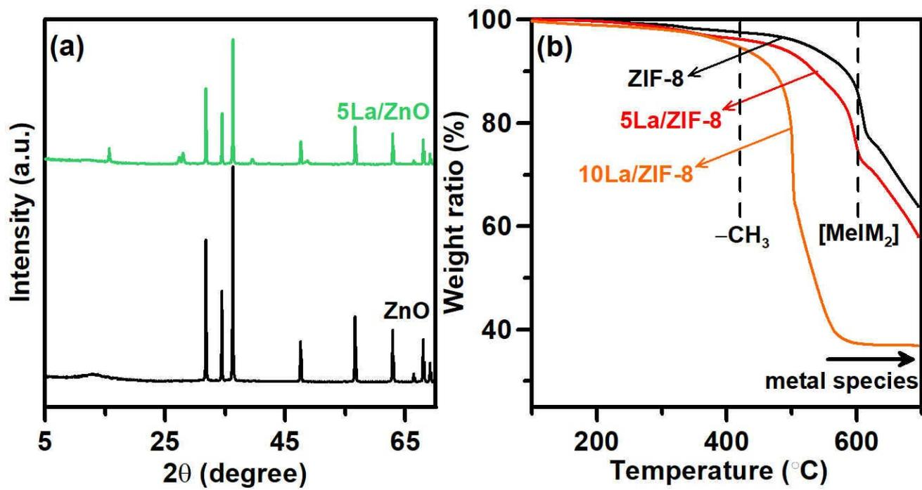
**Figure S1** (a) XRD patterns of ZnO and 5La/ZnO, (b) TGA plot of ZIF-8, 5La/ZIF-8, and 10La/ZIF-8 measured at 100–750 °C with a heating rate of 10 °C min<sup>-1</sup> under continuous air purging.
