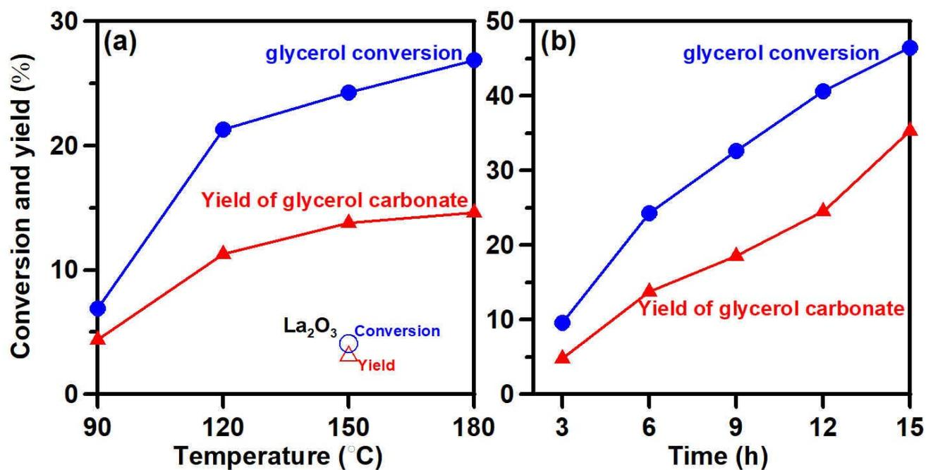
**Figure S5** Catalytic CO<sub>2</sub>/GL conversion at (a) different temperatures with 6 h of reaction, and (b) different reaction times at a reaction temperature of 150 °C. Reaction conditions: 0.1 g of 5La/ZIF-8 (solid symbols) or La<sub>2</sub>O<sub>3</sub> (hollow symbols) catalyst, 5 mL of CH<sub>3</sub>CN as the dehydrating agent, 15 mL of glycerol and 7 bar of CO<sub>2</sub> atmosphere.
