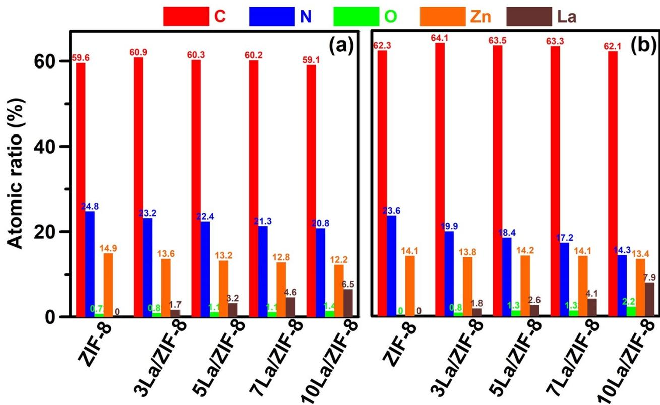
**Figure S4** Elemental analyses of ZIF-8 and La/ZIF-8 samples obtained using (a) XPS and (b) SEM-EDS.
