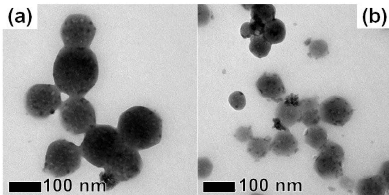
**Figure S7** TEM images of 5La/ZIF-8 (a) before and (b) after the catalytic CO<sub>2</sub>/GL reaction.
