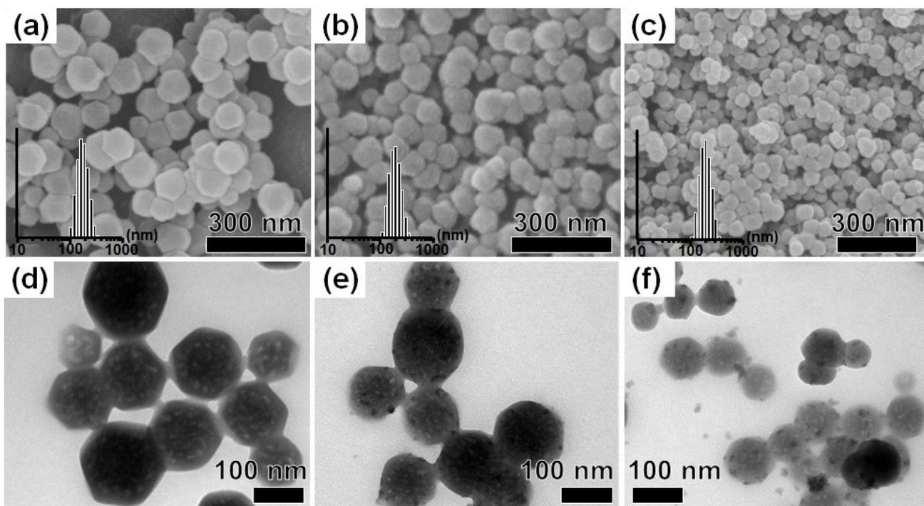
**Figure S2** (a–c) SEM and (d–e) TEM images of ZIF-8, 5La/ZIF-8, and 10La/ZIF-8. Insets of (a–c) indicated the particle size distribution as obtained from DLS analysis.
