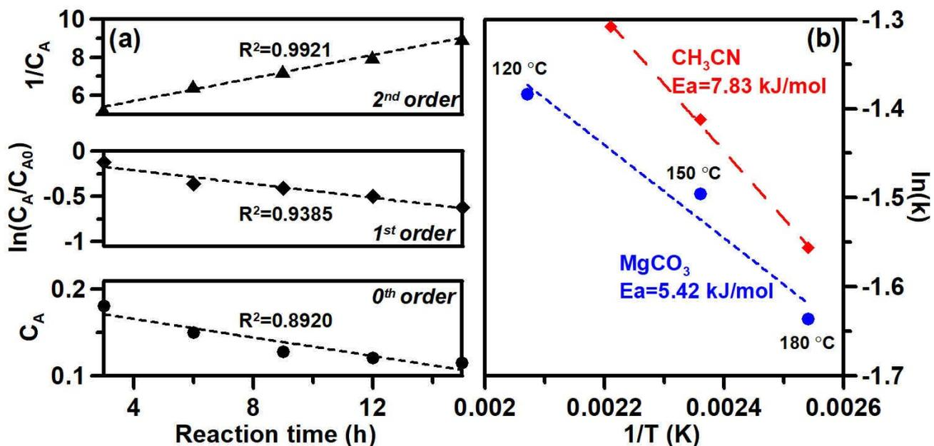
**Figure S8** (a) The calculation of reaction orders and (b) the activation energy for the catalytic  $\text{CO}_2/\text{GL}$  conversion using  $\text{CH}_3\text{CN}$  or  $\text{MgCO}_3$  as the dehydrating agent. The dehydrating agent in (a) is  $\text{CH}_3\text{CN}$ , and the  $C_A$  refers to the concentration of glycerol.
