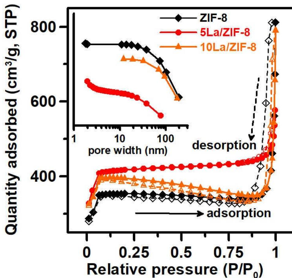
**Figure S3** N<sub>2</sub> adsorption-desorption isotherm of ZIF-8, 5La/ZIF-8, and 10La/ZIF-8 samples. The inset shows the BJH (Barrett, Joyner, and Halenda) pore distribution of these samples.
