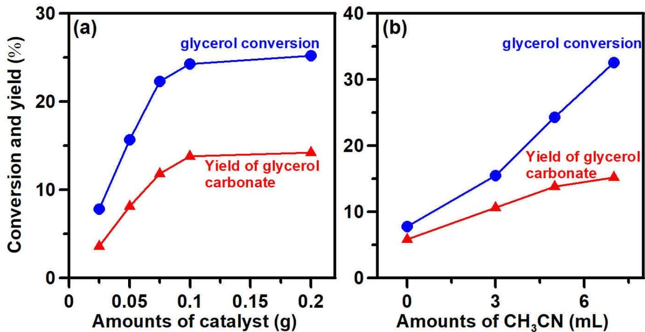
**Figure S6** Catalytic CO<sub>2</sub>/GL conversion using (a) different amounts of catalyst (0.025, 0.05, 0.075, 0.1, and 0.2 g) with 5 mL of CH<sub>3</sub>CN as the dehydrating agent and (b) different amounts of CH<sub>3</sub>CN (0, 3, 5, and 7 mL) with 0.1 g of 5La-ZIF-8 as catalyst. Reaction conditions: 15 mL of glycerol and 7 bar of CO<sub>2</sub> atmosphere at reaction temperature of 150 °C for 6 h.
