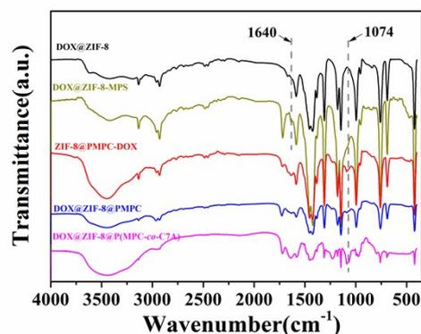
**Figure S3.** The Fourier transform infrared spectra of the DOX@ZIF-8, DOX@ZIF-8-MPS, ZIF-8@PMPC-DOX, DOX@ZIF-8@PMPC and DOX@ZIF-8@P(MPC-co-C7A). The peak at 1640  $\text{cm}^{-1}$  belongs to carbon-carbon double bonds. The peak at 1074  $\text{cm}^{-1}$  belongs to P-O bond.
