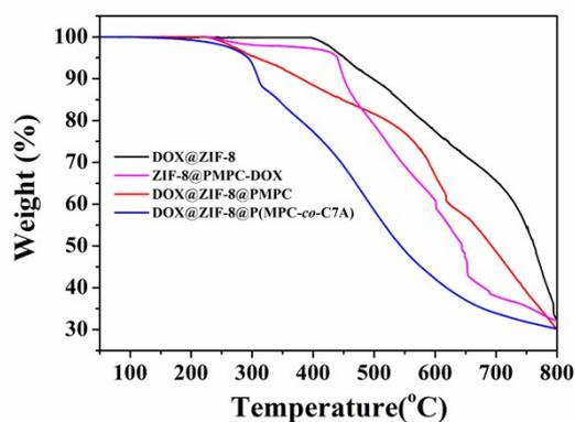
**Figure S5.** Thermogravimetric analysis curve of DOX@ZIF-8, ZIF-8@PMPC-DOX, DOX@ZIF-8@PMPC and DOX@ZIF-8@P(MPC-co-C7A) in the atmosphere of  $\text{N}_2$ .
