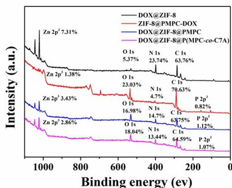
**Figure S4.** The X-ray photoelectron spectroscopy (XPS) spectra of the DOX@ZIF-8, ZIF-8@PMPC-DOX, DOX@ZIF-8@PMPC and DOX@ZIF-8@P(MPC-co-C7A).
