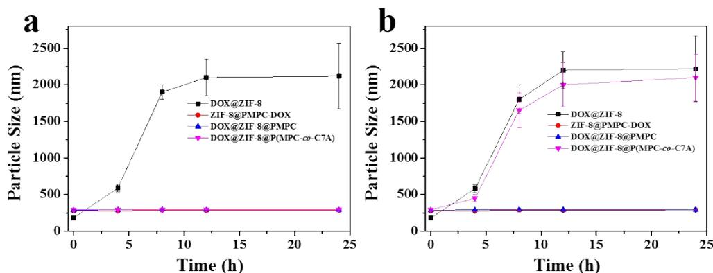
**Figure S11.** The variation of particle size of the DOX@ZIF-8, ZIF-8@PMPC-DOX, DOX@ZIF-8@PMPC and DOX@ZIF-8@P(MPC-co-C7A) at pH 7.4 (a) or 6.5 (b).
