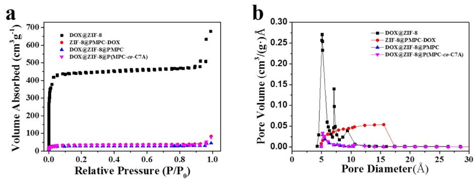
**Figure S6.** Nitrogen adsorption-desorption isotherms (a) and pore size distribution curves (b) for DOX@ZIF-8, ZIF-8@PMPC-DOX, DOX@ZIF-8@PMPC and DOX@ZIF-8@P(MPC-co-C7A).
