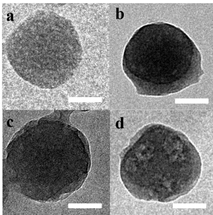
**Figure S2.** The higher magnification TEM images of the DOX@ZIF-8 (a), DOX@ZIF-8@PMPC (b), DOX@ZIF-8@P(MPC-co-C7A) (c) and ZIF-8@PMPC-DOX (d). Scale bars were 50 nm.
