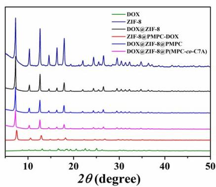
**Figure S7.** Powder X-ray diffraction patterns of DOX, ZIF-8, DOX@ZIF-8, ZIF-8@PMPC-DOX, DOX@ZIF-8@PMPC and DOX@ZIF-8@P(MPC-co-C7A).
