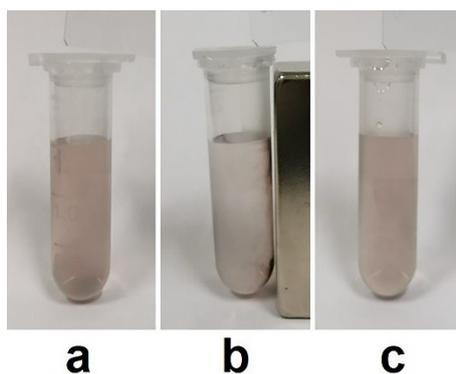
**Figure S3.** Photographs of CM-Fe<sub>3</sub>O<sub>4</sub>@Au-Ab before (a) and after (b) magnetic separation and the removal (c) of the extra magnet.
