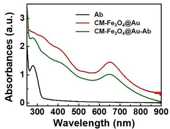
**Figure S2.** UV-vis-NIR spectra of Ab, CM-Fe<sub>3</sub>O<sub>4</sub>@Au and CM-Fe<sub>3</sub>O<sub>4</sub>@Au-Ab.
