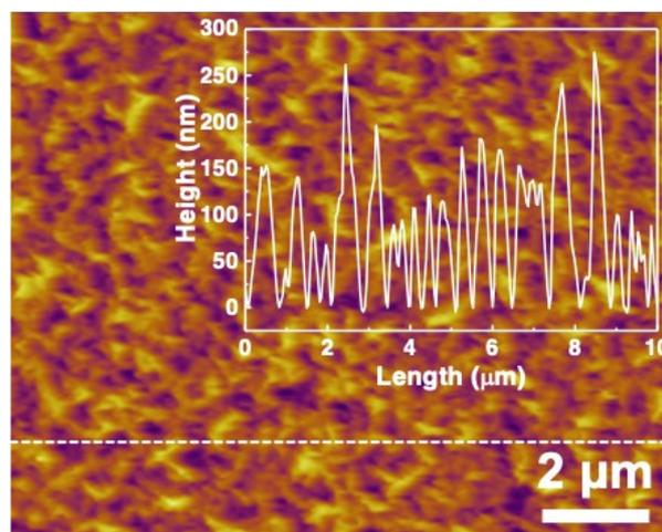
Fig. S6 Contact-mode AFM image of the graphene grown on the Si and SiO<sub>2</sub> substrates. The inset shows the height of the graphene materials.
