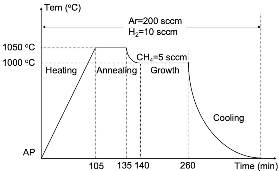
Fig. S1 Experimental thermal process schematic illustrates the growth of the horizontally aligned graphene films.
