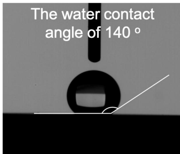
Fig. S7 The water contact angle of graphene grown on the Si and SiO<sub>2</sub> substrates.
