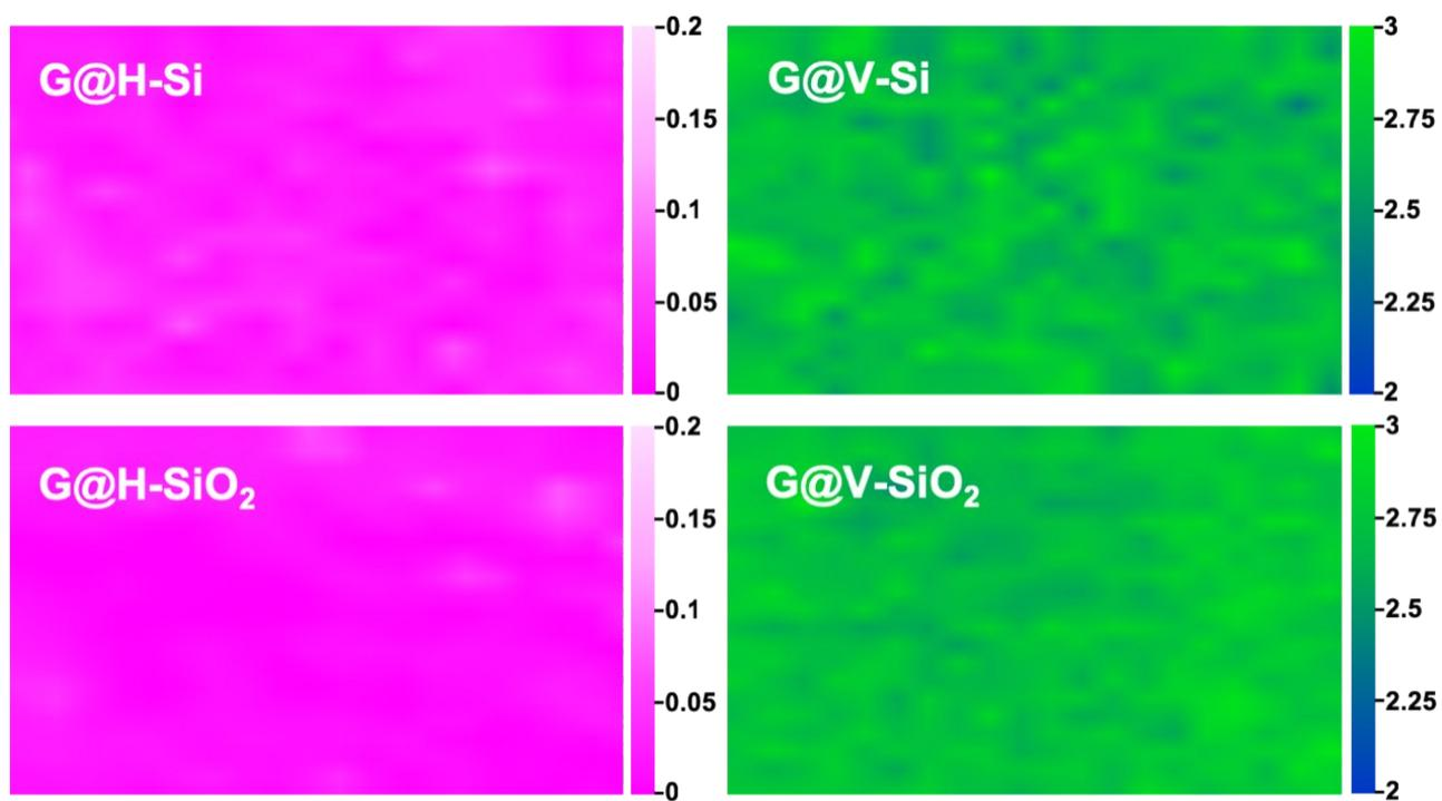
Fig. S5 The  $I_D/I_G$  peak ratio derived from Raman mapping over an area measuring  $1\text{ cm} \times 1\text{ cm}$  on the graphene coatings.
