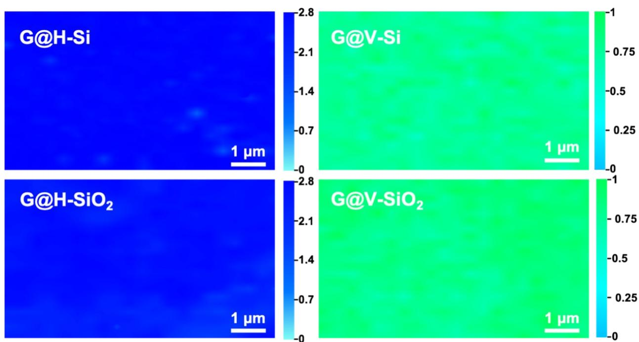
Fig. S4 The  $I_{2D}/I_G$  peak ratio derived from Raman mapping over an area measuring 1  $\text{cm} \times 1 \text{cm}$  on the graphene coatings.
