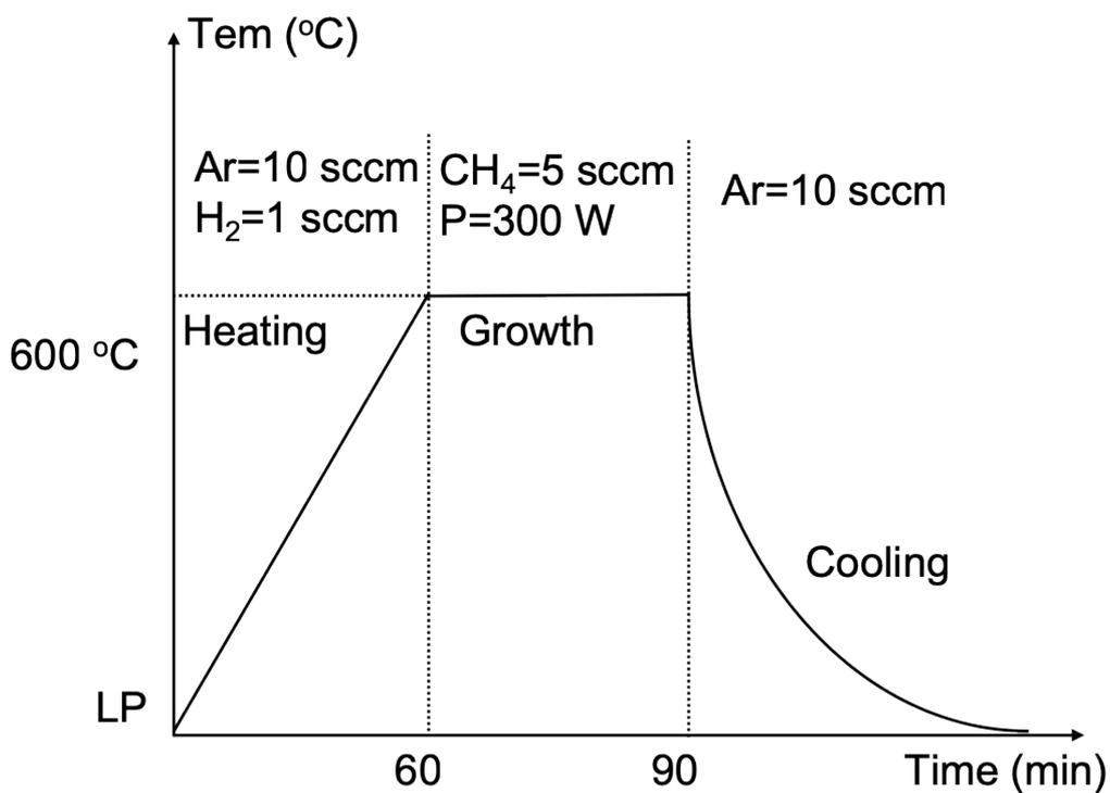
Fig. S2 Experimental thermal process schematic demonstrates the growth of the vertically aligned graphene sheets.
