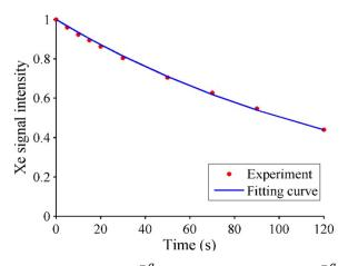
Figure S5. Longitudinal relaxation rates  $R_1^a$  of <sup>129</sup>Xe in solution. The  $R_1^a$  value of 0.0069 s<sup>-1</sup> was measured by fit
