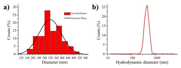
Figure S3. a) size distribution and gaussian fitting of FLAME by transmission electron microscopy (TEM). The average diameter of FLAME is 325 nm and the Standard deviation is 73 nm. b) Hydrodynamic diameter of the FLAME by Dynamic light scattering (DLS), the average hydrodynamic diameter of FLAME is 396 nm.
