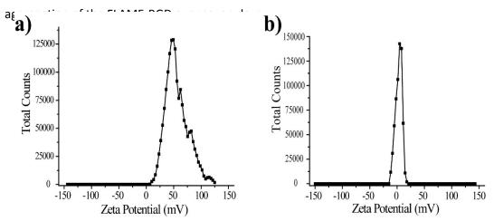
Figure S8. The Zeta potential distribution curves of FLAME and FLAME-RGD. The carboxyl-PEG on the surface of FLAME-RGD reduced the Zeta potential of FLAME-RGD
