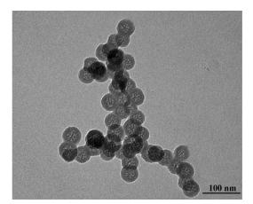
Figure S1. TEM image of MSNs. Fresh prepared MSNs were suspended in water and loaded on copper mesh a day before test.
