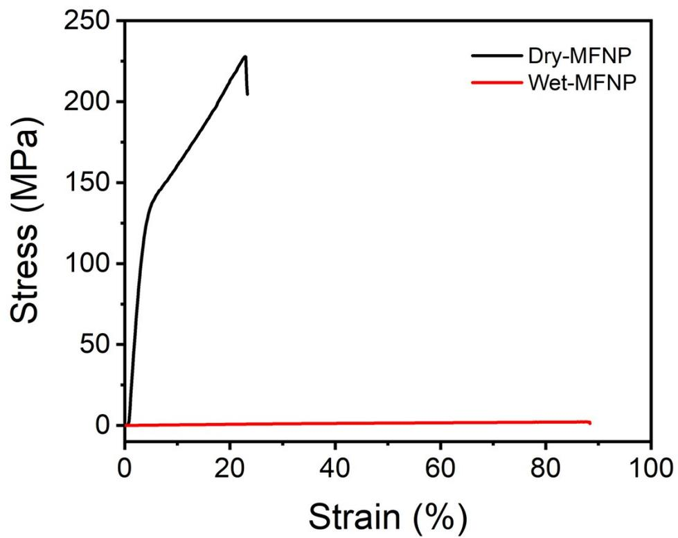
**Figure S9.** Stress-strain curves of dry and wet fibers.
