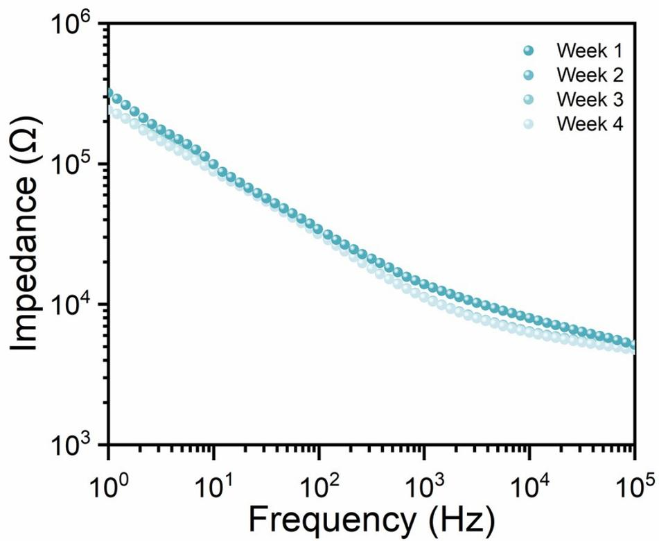
**Figure S20.** Impedance spectra of a Wet-MFNP immersed in artificial cerebrospinal fluid of mice for 4 weeks.
