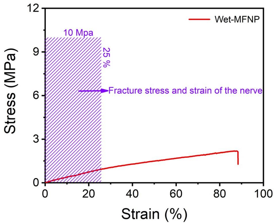
**Figure S10** Stress-strain curve of the wet fiber and fracture stress and strain of the nerve.
