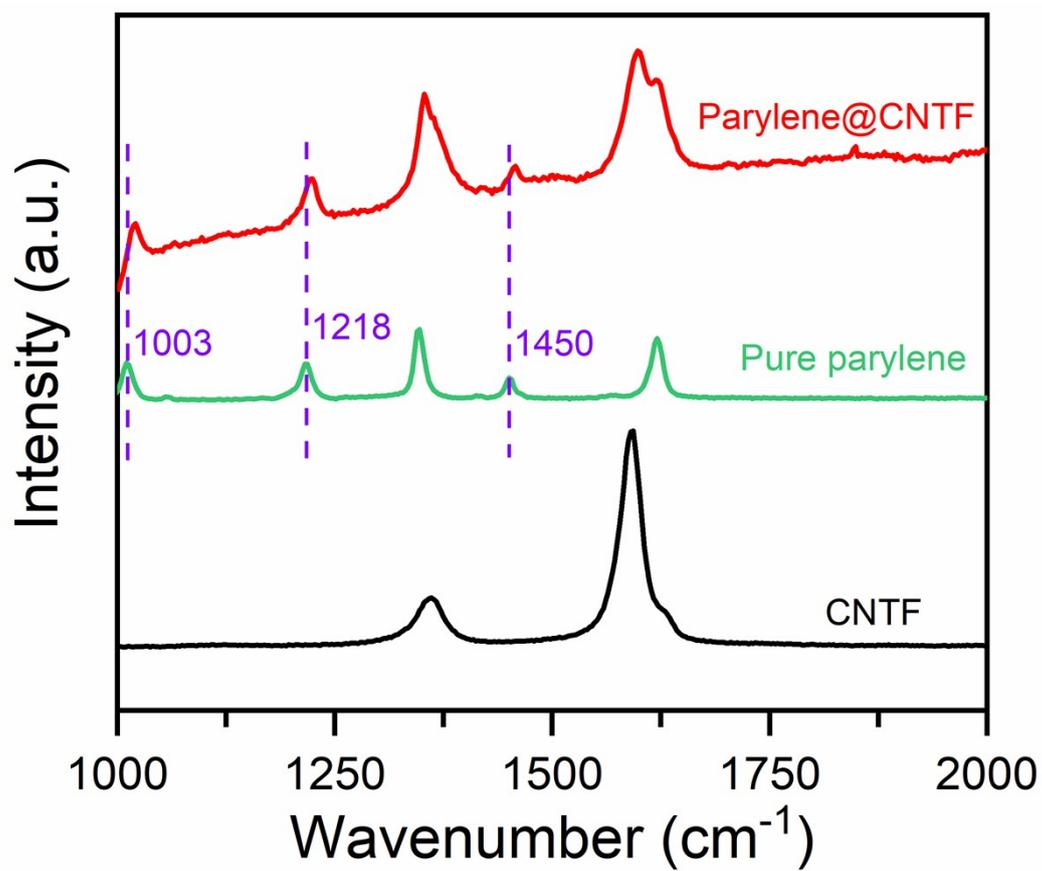
**Figure S2.** Raman spectra of the CNTF, parylene and CNTF coated with parylene on the surface.
