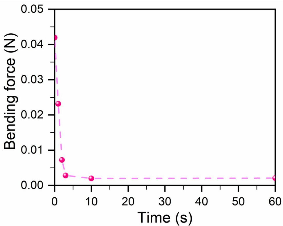
**Figure S7.** The tested bending force of Dry-MFNPs after immersed in artificial cerebrospinal fluid of mice for different periods.
