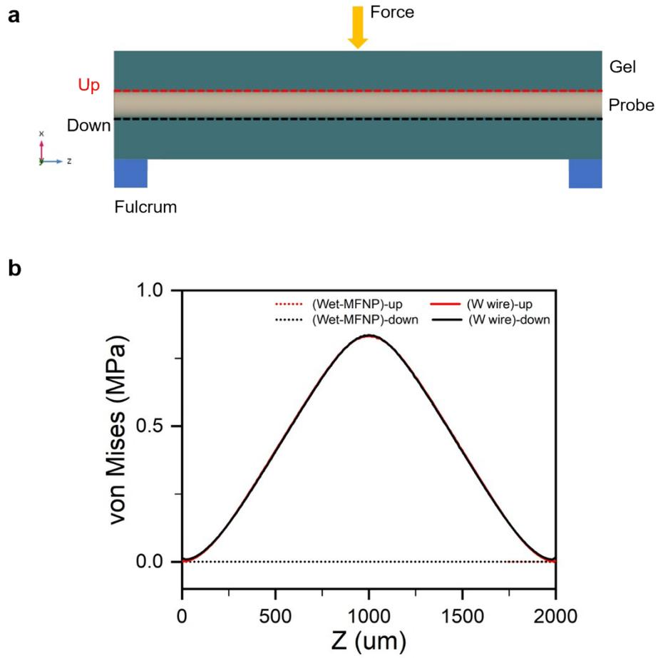
**Figure S12. a**, The gel was fixed at both ends, and an equal amount of displacement occurs in the middle. **b**, Distribution of von Mises in gel/probe interface.
