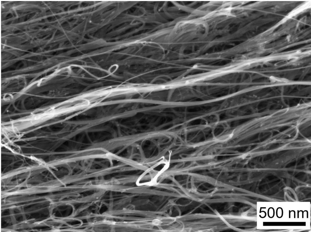
**Figure S4.** SEM image of a CNTF.
