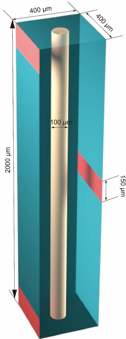
**Figure S11.** Model and size for finite element analysis.
