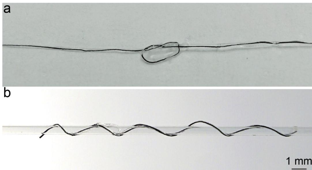
**Figure S5.** Photographs of the Wet-MFNP being (a) folded and (b) wrapped around a capillary.
