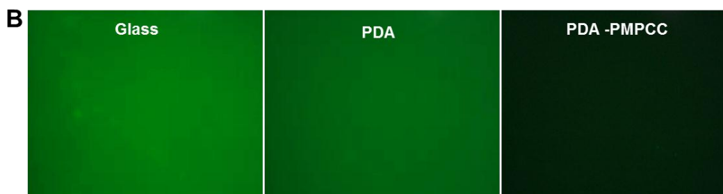
Fig. S6. (A) Fluorescence intensity vs concentration curve of FITC-BSA solutions. (B) Fluorescence microscopic images of the FITC-BSA adsorbed from 1.00 mg/mL solution on the bare, PDA and PDA-PMPCC coated glass surfaces.
