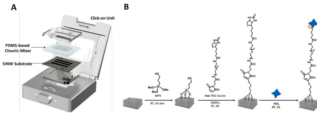
**Supplementary Figure 1.** (A) Schematic diagram of the components of the NanoVelcro Chips. The chip holder compresses the PDMS-based chaotic mixer against the channels of the silicon nanowire chip to create a microfluidic channel which optimizes cellular interactions with the chip surface. (B) Illustration of the modification procedures of the NanoVelcro Chips before capture of biotinylated anti-EpCAM labeled tumor cells.
