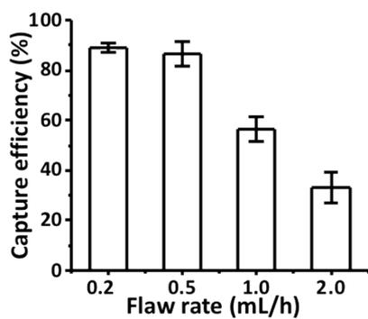
**Supplementary Figure 2.** CTC-capture efficiency of the NanoVelcro Chips was studied at flow rates of 0.2, 0.5, 1.0 and 2.0 mL h<sup>-1</sup>.
