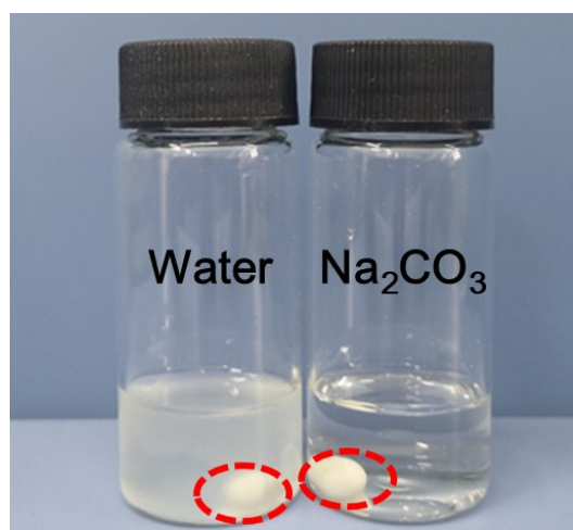
Fig. S2 Photographs of the PVP-Ca 15-0.3 hydrogels immersed in distilled water and 1 mol L -1 Na 2 CO 3 aqueous solution.
