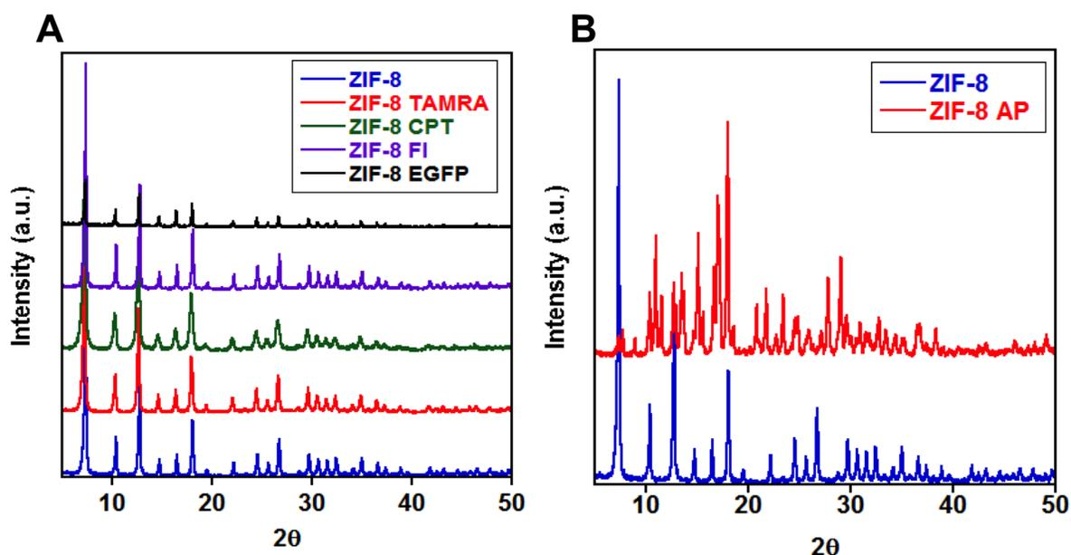
**Figure S2.** (A) PXRD spectra of ZIF-8 with different cargo shown retaining the characteristic peak pattern for an empty ZIF-8 MOF. The ZIF-8 PXRD spectrum is consistent with those reported in simulations and literatures.<sup>2-4</sup> (B) PXRD spectrum comparison between ZIF-8 and ZIF-8 AP.
