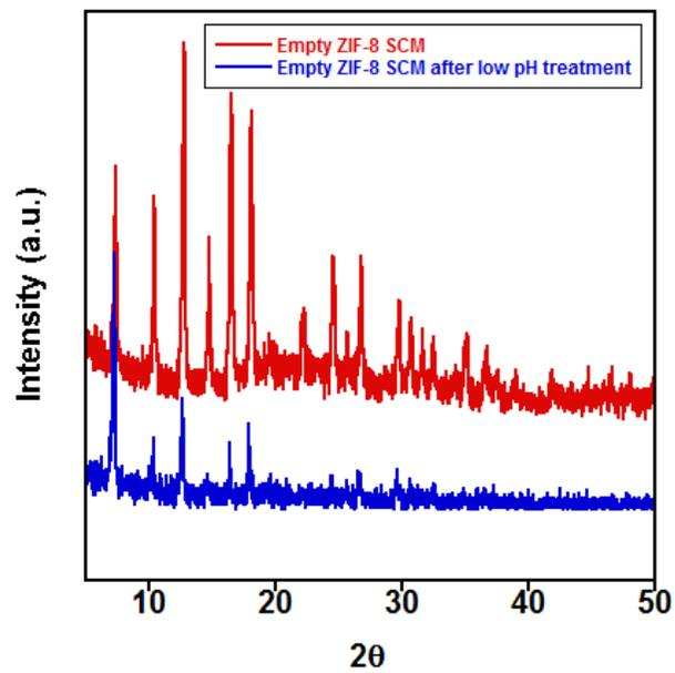
**Figure S4A.** PXRD spectrum indicating the retention of ZIF-8 crystal structure inside the SCM even after incubating at low pH (0.10 M pH 5.20 sodium acetate buffer) for an hour.
