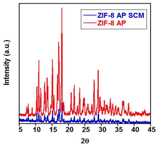
**Figure S3.** PXRD spectrum comparison between ZIF-8 AP and ZIF-8 AP SCM showing the preservation of ZIF-8 AP crystallinity and the influence of the protein cargo on the overall structure.
