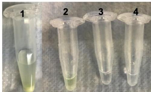
**Figure S9** (1) ZIF-8 AP + substrate (2) ZIF-8 AP SCM + esterase + substrate (3) ZIF-8 AP SCM + substrate (4) esterase + substrate. Unmasking the ZIF-8 AP SCM with esterase allows the clear substrate (PNPP) to diffuse into the ZIF-8 MOF and be converted to the bright yellow product (PNP). All nanoparticles are dispersed in 40 mM pH 8.0 Tris-HCl buffer with 1 mM  $\text{MgCl}_2$ .
